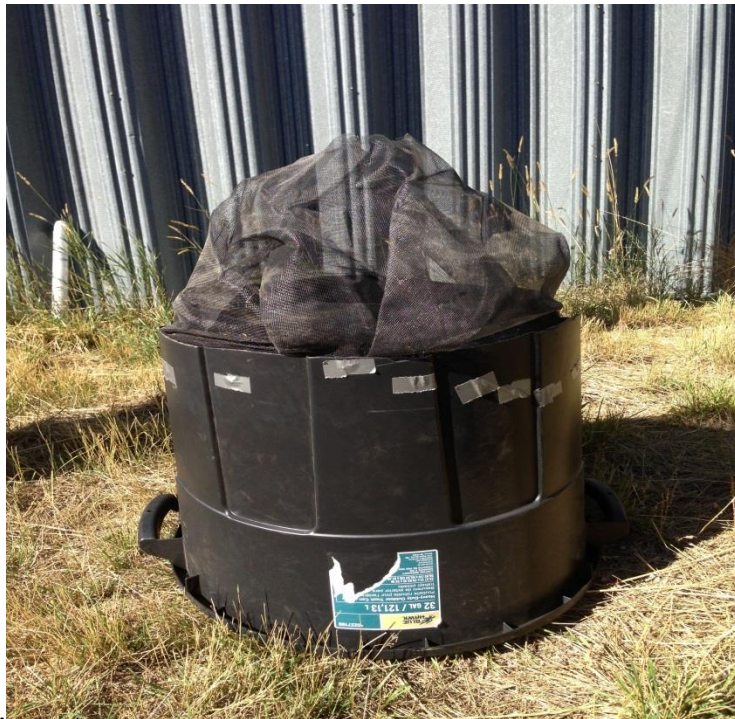
Figure 8. Drop-trap used to vacuum-collect insects constructed from a trash can (121.13 Liters) and mesh window screen.
