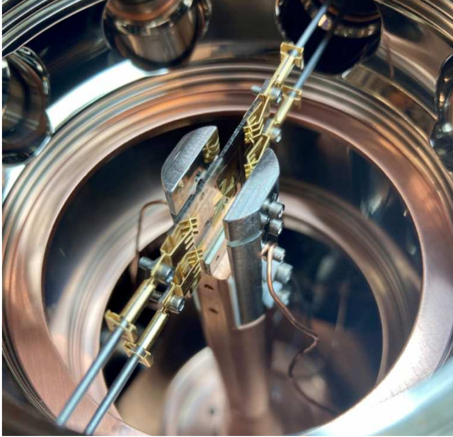
Figure 2.5: An image of the assembled trap is shown within the vacuum chamber. The diamond wafer with gold coated electrodes is secured to a copper post for heat dissipation, with titanium endcaps mounted on either side.
