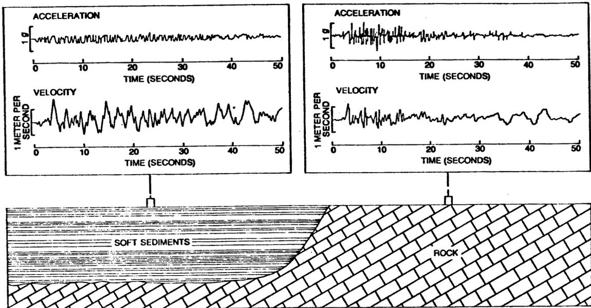
Figure 19. Effects of local site conditions on shaking intensity and frequency of ground motion for sites subjected to strong ground shaking.
