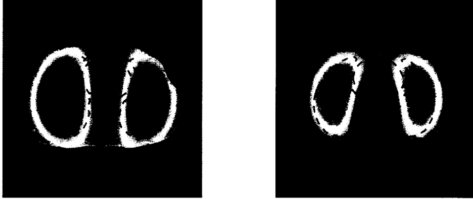
Figure 9.7: Reconstructions of t_{diff}^{exp} using \Lambda_{\gamma_1} with a heart = 670mS/m and lungs = 100mS/m using dTCP and different nonhomogeneous \Lambda_{\gamma_2} . On the left \Lambda_{\gamma_2} using a heart = 500mS/m and lungs = 200mS/m and on the right \Lambda_{\gamma_2} using a heart = 750mS/m and lungs = 40mS/m. The truncation radius was set to 2.4.
