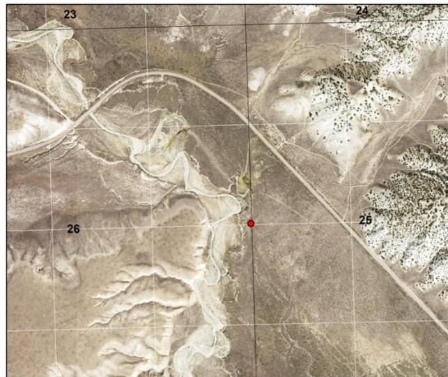
**Figure A.5.** Monumented  $\frac{1}{4}$  section corner between S26 and S25 in T8NR98W. The monument stone to mark the corner placed by surveyors during the 1906 survey was located by surveyors during a subsequent resurvey in 1984. Given the proximity to the Sand Wash channel, the monuments persistence suggests that the 1906 channel was incised below the terrace surface on which the  $\frac{1}{4}$  section corner monument sits at the time it was placed.
