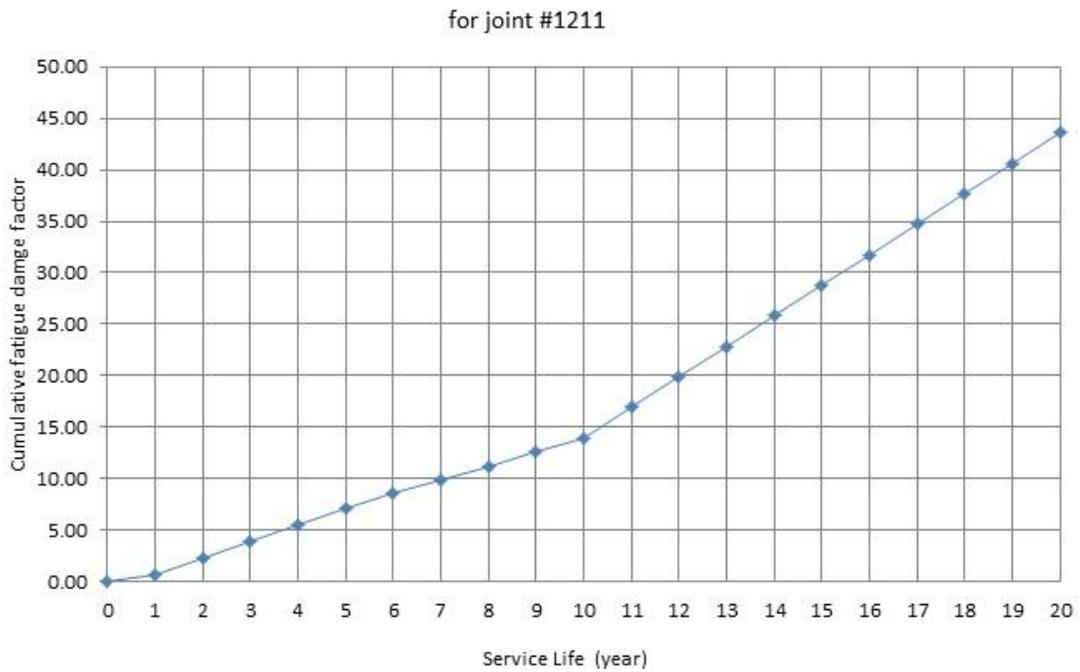
Figure 5.25 Cumulative damage facto versus service life for joint #1211
