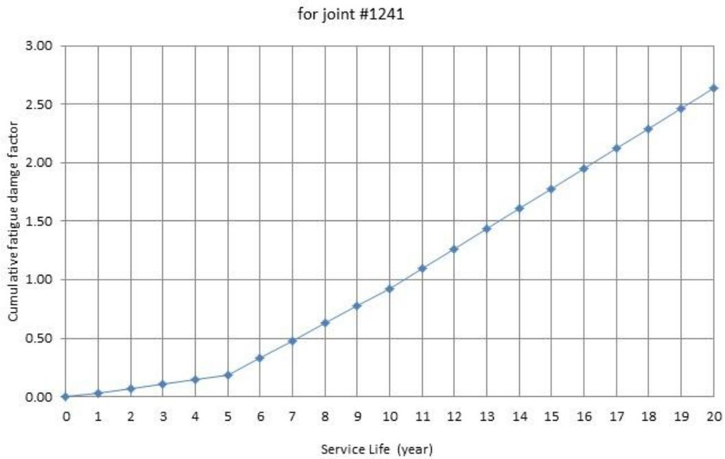
Figure 5.27 Cumulative damage facto versus service life for joint #1241
