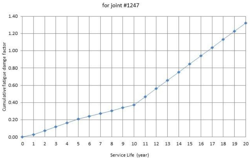
Figure 5.29 Cumulative damage facto versus service life for joint #1247
