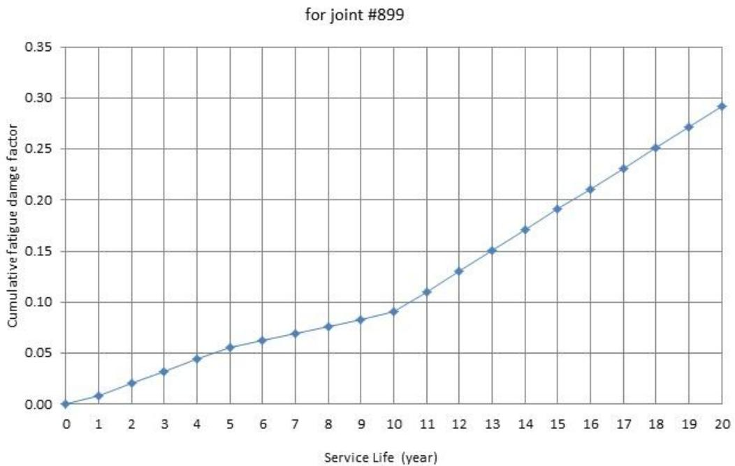
Figure 5.19 Cumulative damage facto versus service life for joint #899
