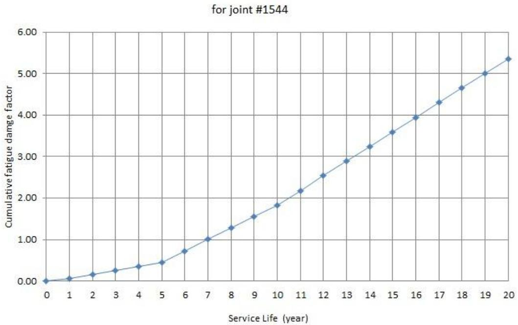
Figure 5.33 Cumulative damage facto versus service life for joint #1544
