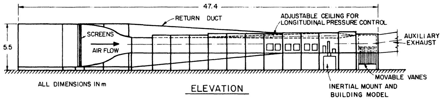
Figure 4. Meteorological Wind Tunnel
