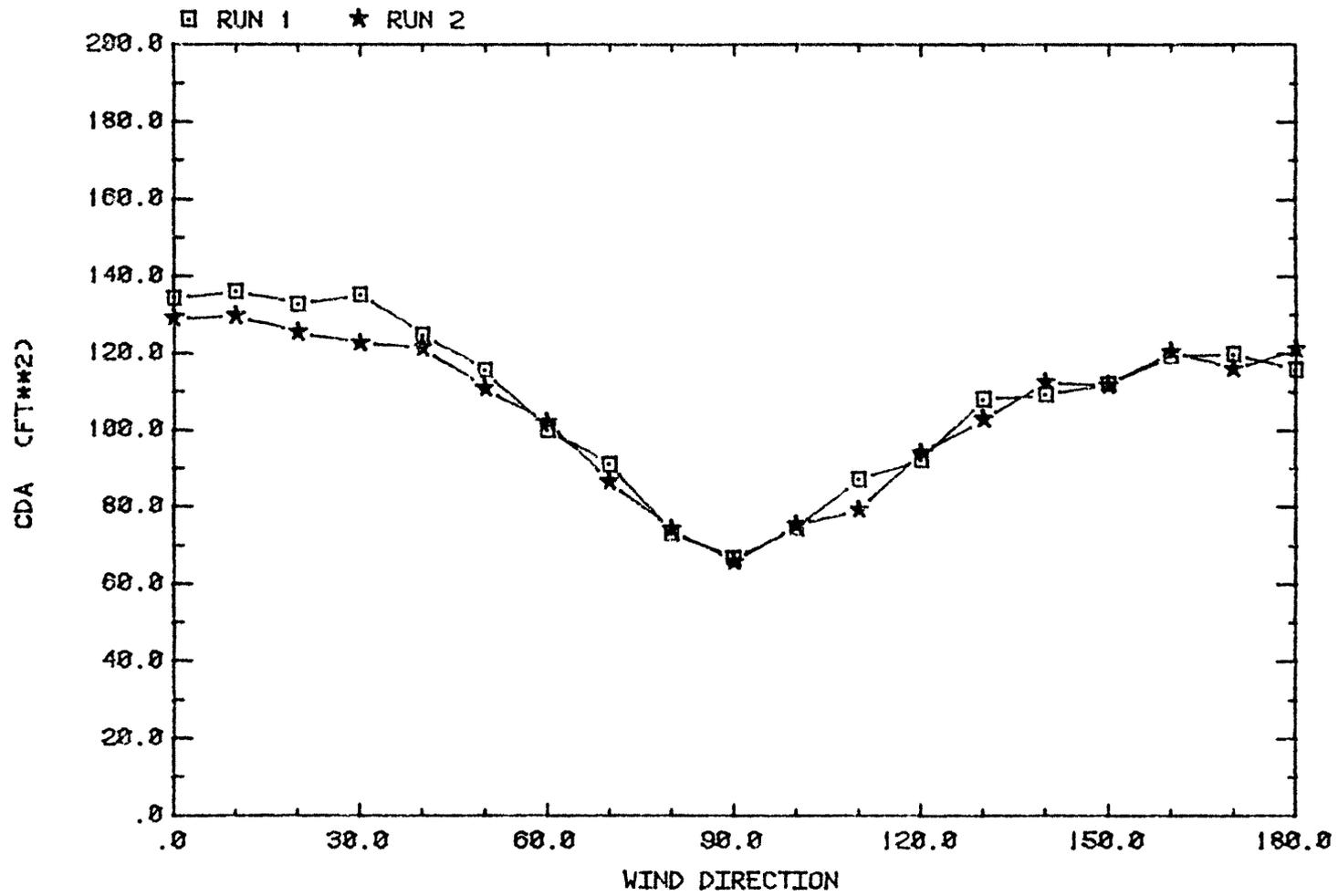
Figure 10.  $C_D A$  of Modified Gabriel Antenna--Run 1 and 2
