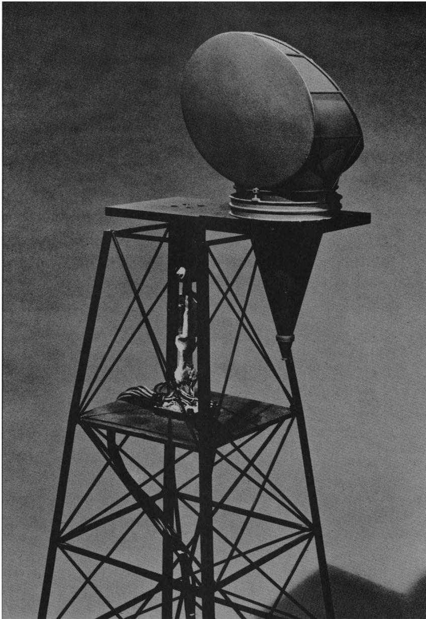
Figure 6. Conical Horn Antenna Cluster
