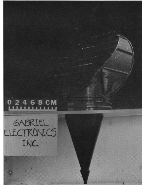
Figure 1. Conical Horn Antenna - Gabriel UHR10 D (Original Model)
