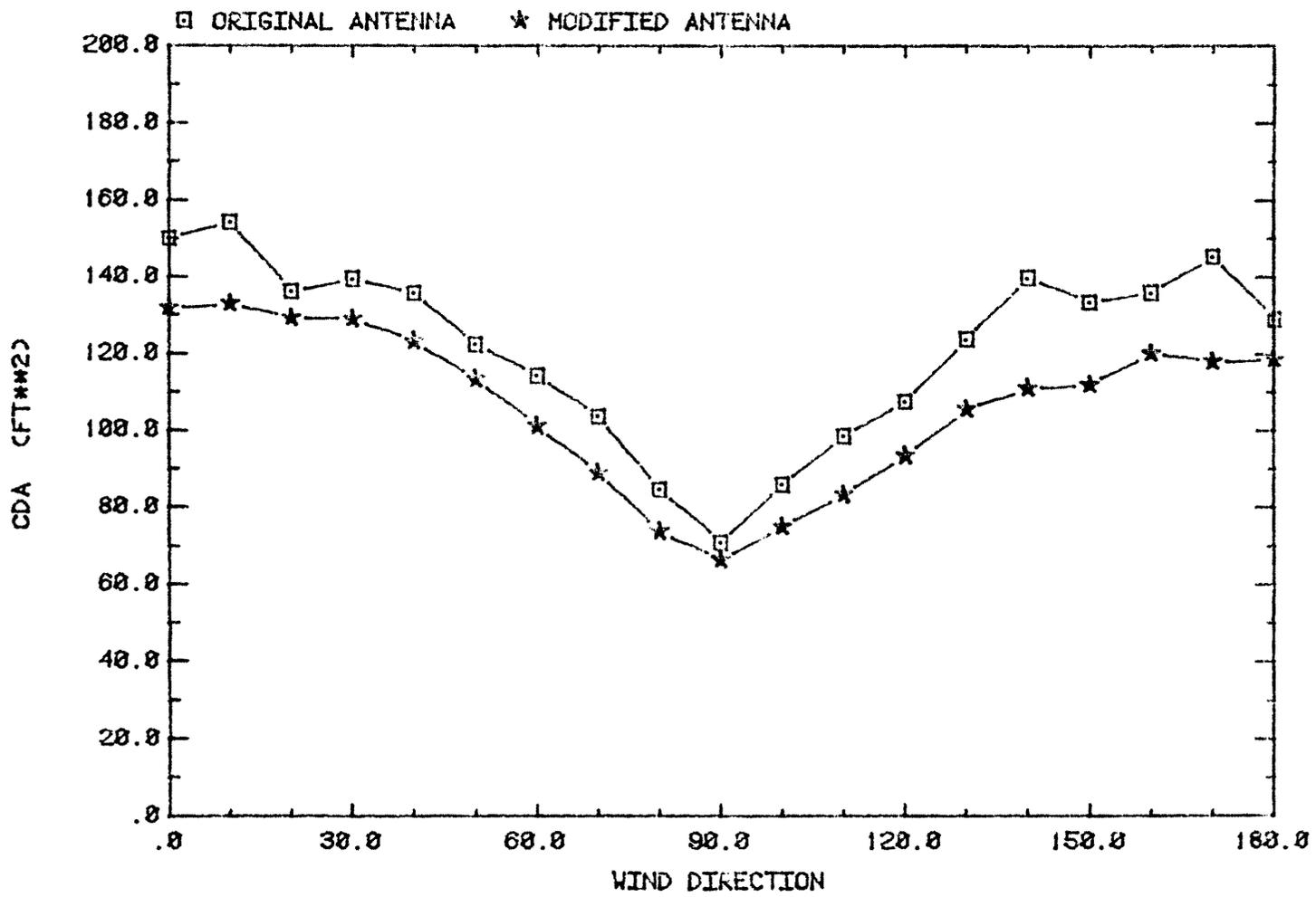
Figure 12.  $C_D A$  of Modified and Original Gabriel Antenna
