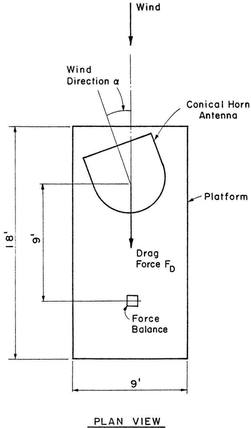
Figure 3. Definition of Drag and Wind Direction
