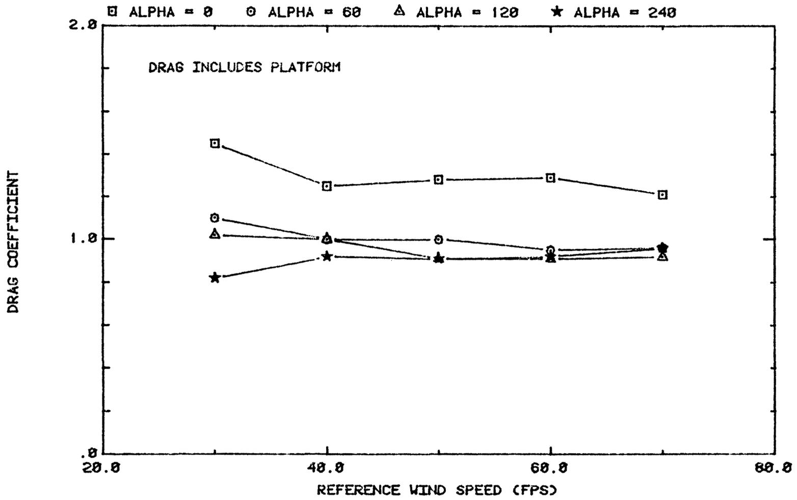
Figure 2. Effect of Wind Speed on the Drag of Conical Horn Antenna (Ref. 5)
