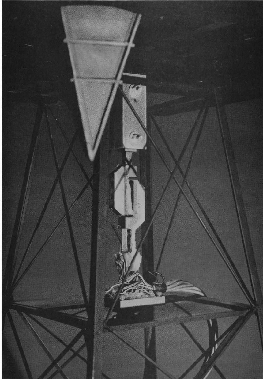
Figure 7. Force Balance Setup
