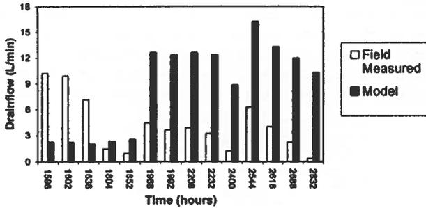
Fig. 12. Comparison of modeled and field drain flows
