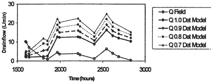
Fig. 16. Observed Drain Discharge Compared to Simulated Values for Four  $D_a$  Levels
