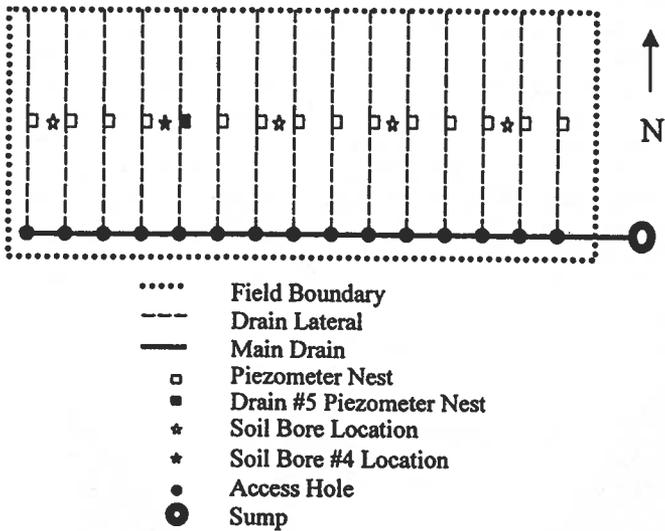
Fig. 4. Site Plan of NARC
