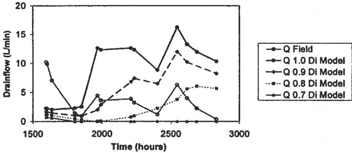
Fig. 15. Observed Drain Discharge Compared to Simulated Values for Four  $D_i$  Levels
