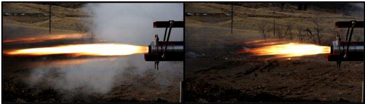
Figure 36. 3.45 MPa: Flame pre (left) and post (right) phase change.
