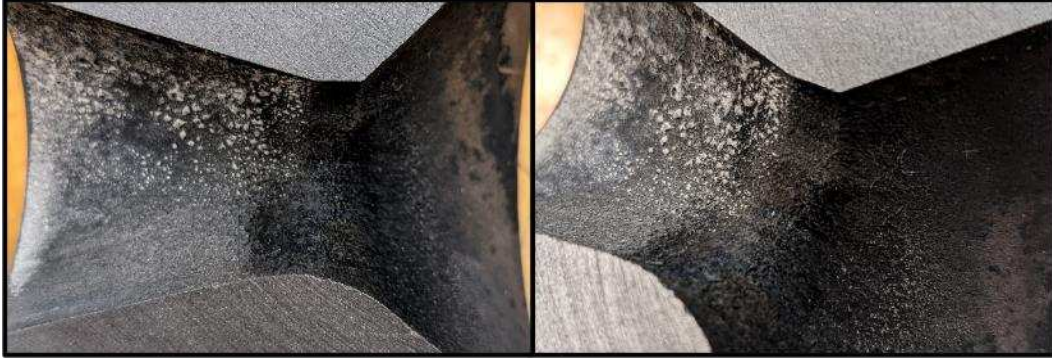
Figure 52. Two perspectives, frontal cross-section (left) and close-up of the throat (right), of the nozzle post burn.
