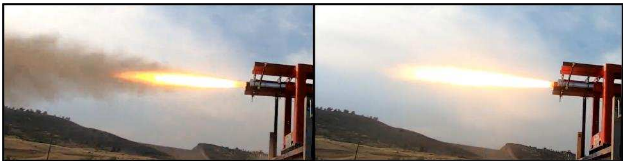
Figure 32. 4.83 MPa: Flame pre (left) and post (right) phase change.
