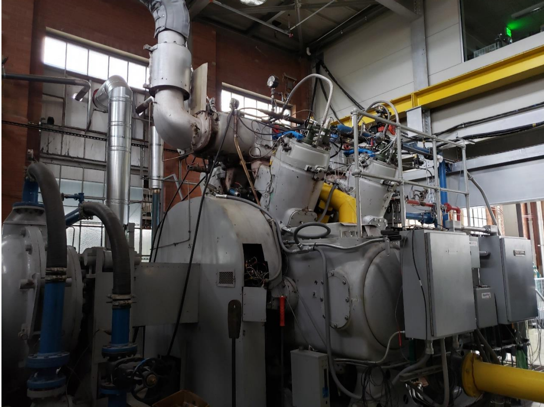
Figure 2-1. Cooper-Bessemer GMV-4 at the CSU Engines and Energy Conversion Laboratory (EECL).
