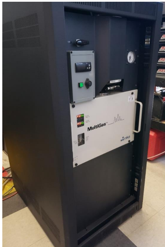
Figure 2-12. MKS Instruments, Inc. Model No. 2030 FTIR.
