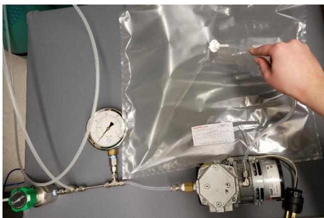
Figure 2-15. Tedlar bag sampling system.
