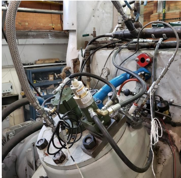
Figure 2-17. Engine/ Woodward HPFI system installed on the GMV-4 engine.
