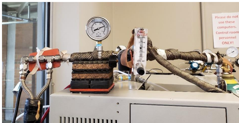
Figure 2-14. Sample manifold and Tedlar bag setup on top of the HP 5890 Series II GC.
