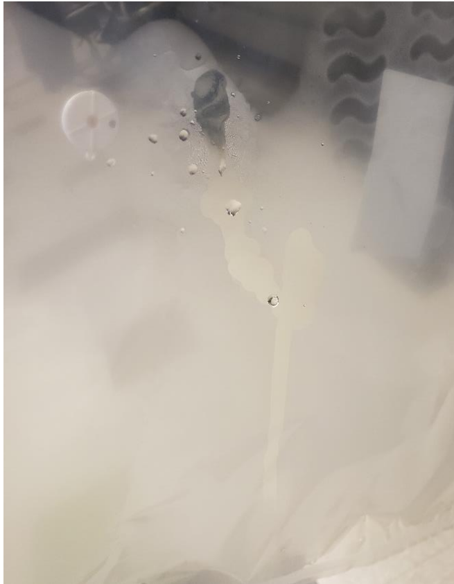
Figure 4-22. Tedlar bag showing water condensation on the inner surface immediately after exhaust gas was filled.
