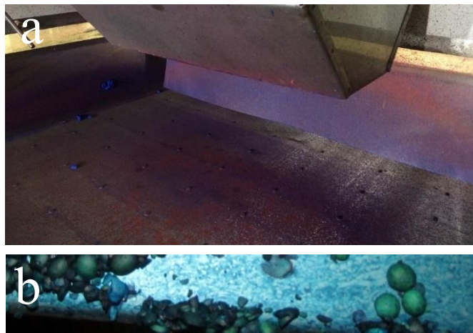
Figure 4.1. a) Seed treatment dryer with seed dressing buildup. b) Seed agglomeration in seed treatment hopper after 3 hours of operation.
