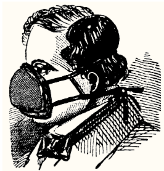
Figure 1.2: Dr. Stenhouse’s respirator featuring hollow wire gauze (Youmans, 1863)
