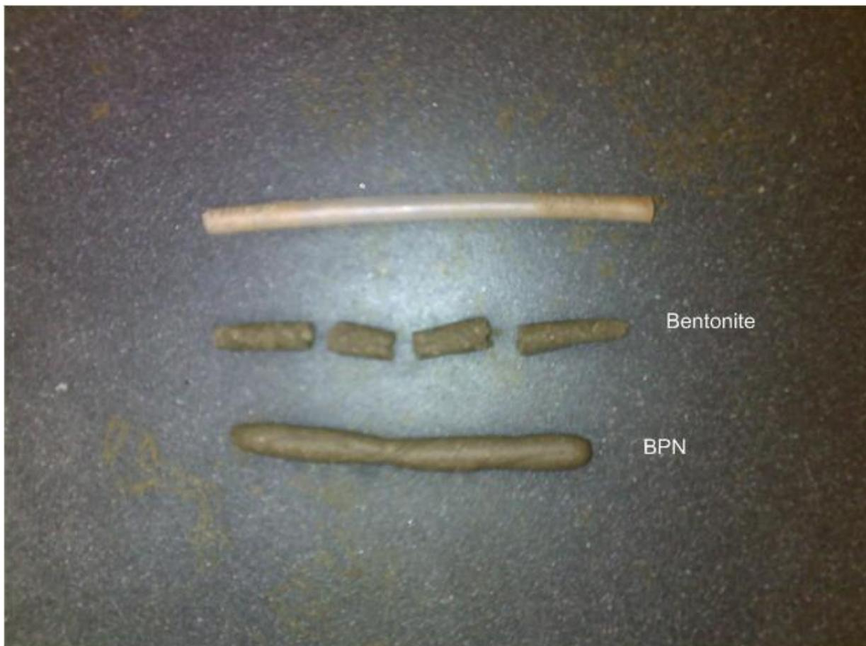
Figure 3.2. Photograph of traditional bentonite and bentonite polymer nanocomposite (BPN) plastic limit "worms."
