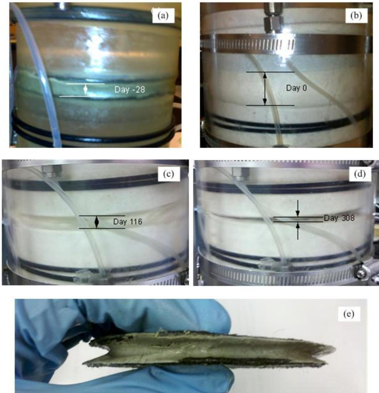
Figure 5.11. Photographs depicting BPN specimen volume change during membrane testing in a flexible-wall cell: (a) before circulation of DIW; (b) after circulation of DIW but before circulation of 5 mM  $\text{CaCl}_2$ ; (c) during circulation of 10 mM  $\text{CaCl}_2$ ; (d) after circulation of 20 mM  $\text{CaCl}_2$ ; (e) after termination of test.
