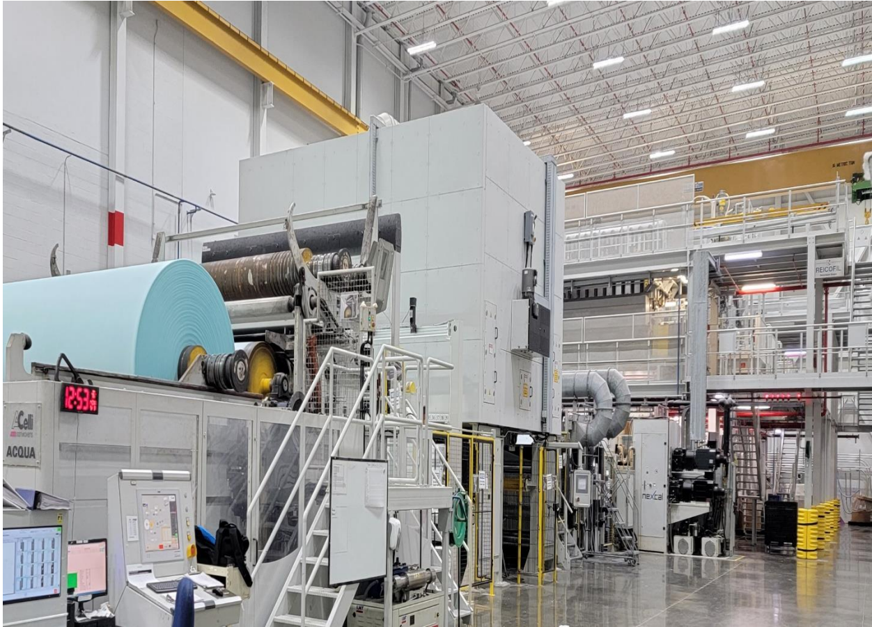
Figure 4.9 Reicofil-IV SMS Production system. BERRY©
