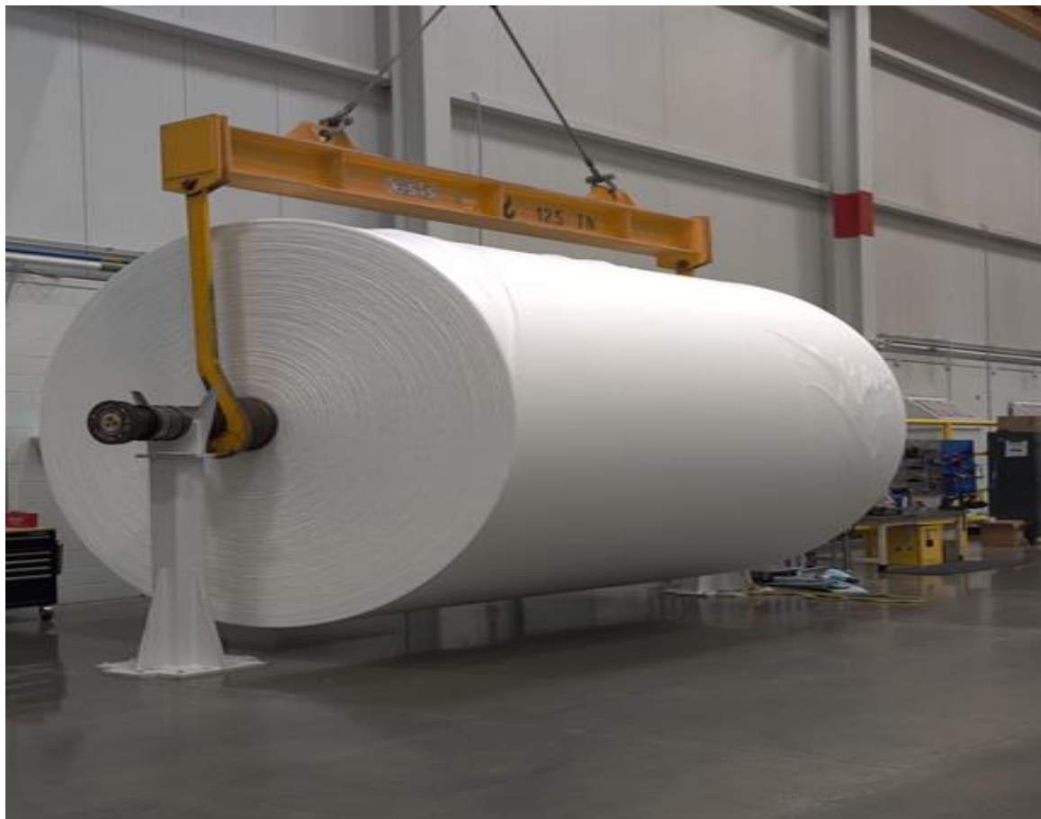
Figure 1.4 S-M-S Nonwoven on a winder mandrel lifted by 12.5-ton crane.
