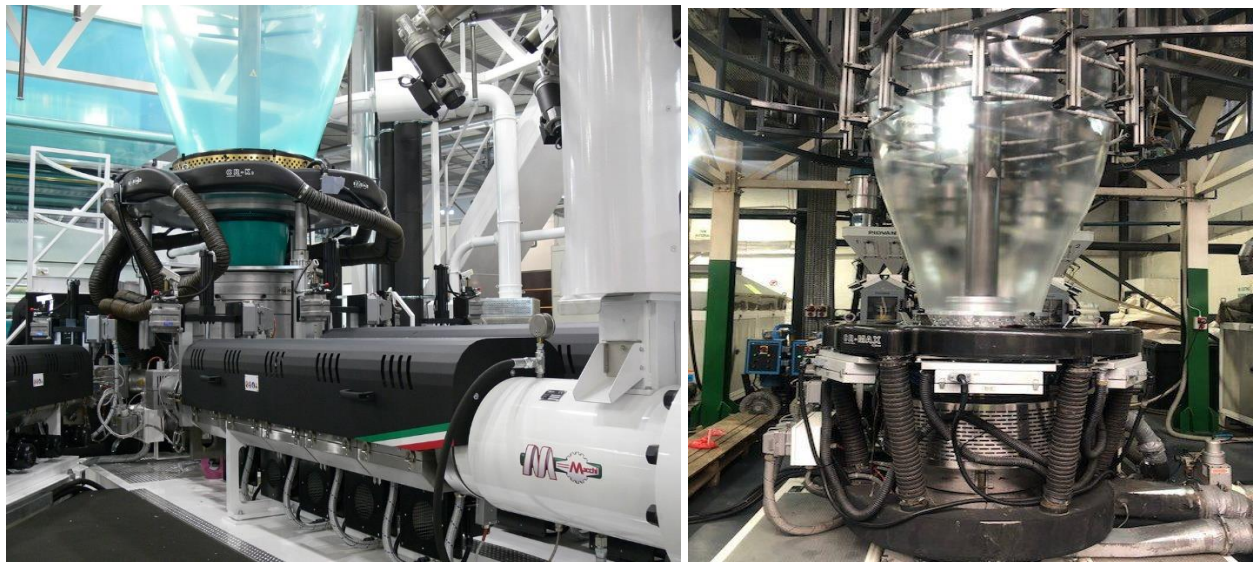
Figure 5.5 Formation of plastic film bubbles. BERRY©
