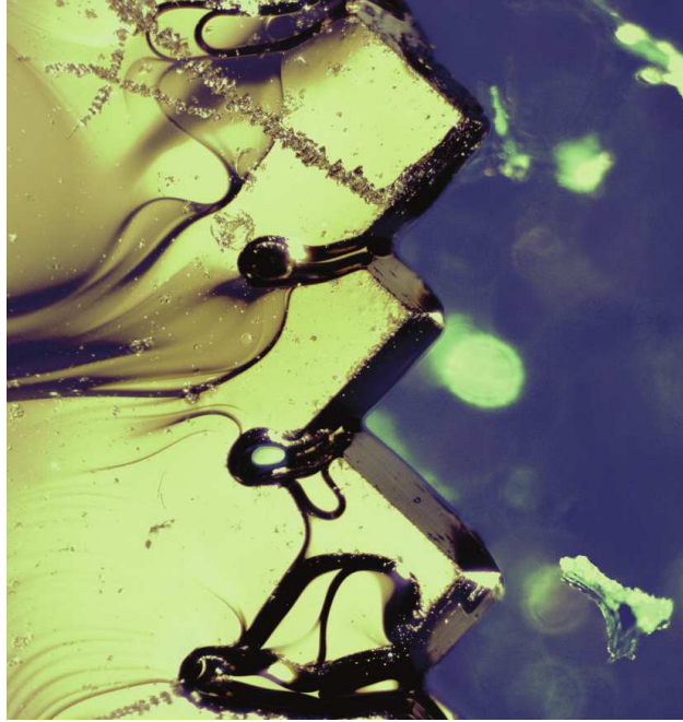
Figure 2: A crystal of CaFe 2 As 2 utilized in a nanoindentation study of plastic deformation [26].
