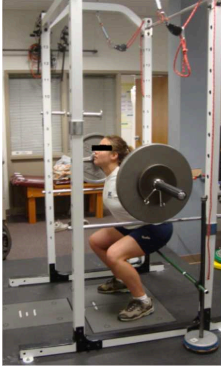
Figure 3.1: Squat cage positioned over force platforms with visible safety pins and depth bar. Also visible is the 3 rd force platform utilized for hopping tests. Note: Spotters normally stood at each end of the bar.
