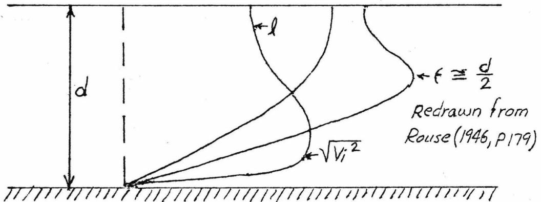
Fig. 5 - Velocity Distribution in Turbulent Flow
