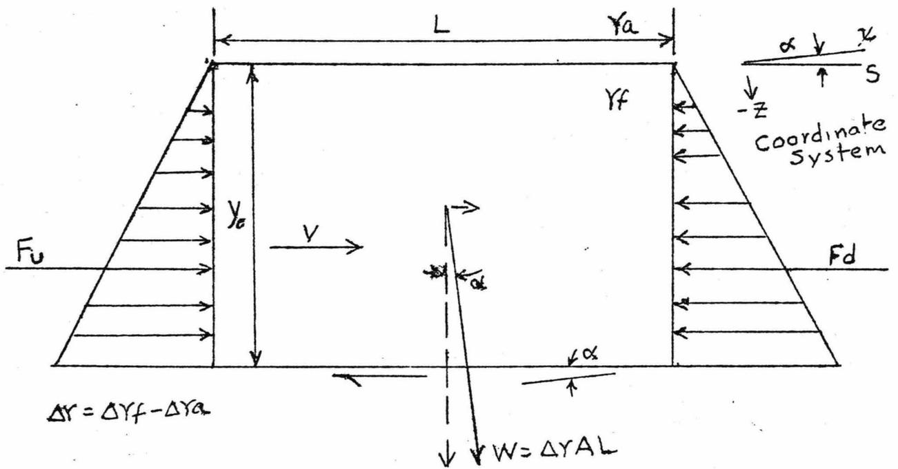
Fig. 9 - Free-body Diagram of Segment of Open Channel Flow
