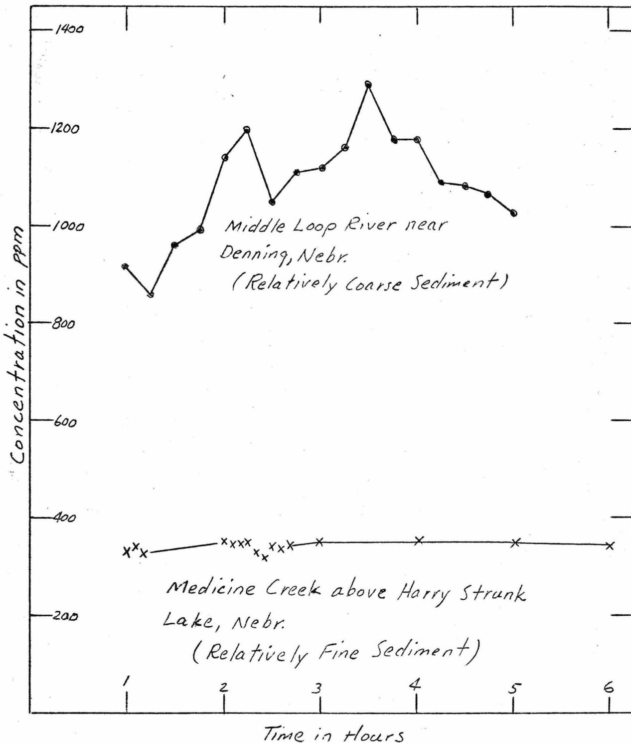
Fig. 15. -- Variations in suspended sediment concentration of samples with time for two streams having relatively fine and coarse sediment.
