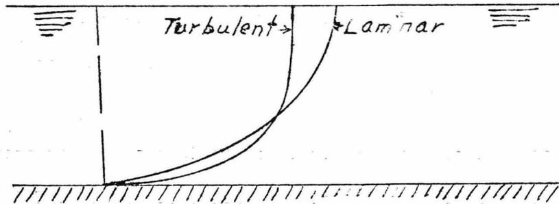
Fig. 4-Comparison of Velocity Distribution in Laminar and Turbulent Flow.
