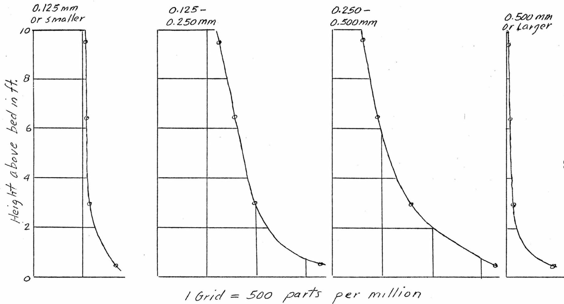
Fig. 13. -- Particle size of suspended sediment with depth at a single vertical on the Niobrara River near Cody, Nebraska on April 27, 1951, at the contracted section.
