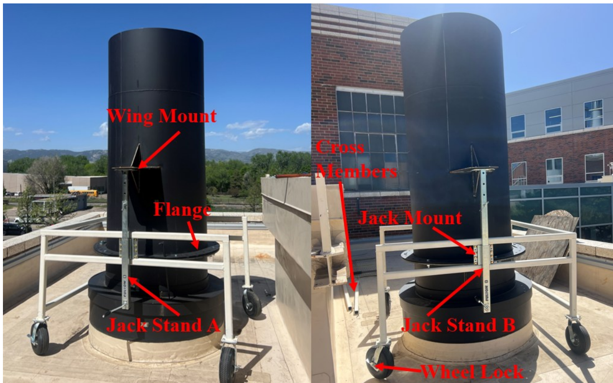
Figure 90: Exhaust stack and mobile cart assembly installed in the firing assembly. The chimney stack can be raised and lowered by cranking jack stands A and B in synchrony until the desired height is achieved. The jack stands will self lock, and will not “self crank” or unwind
