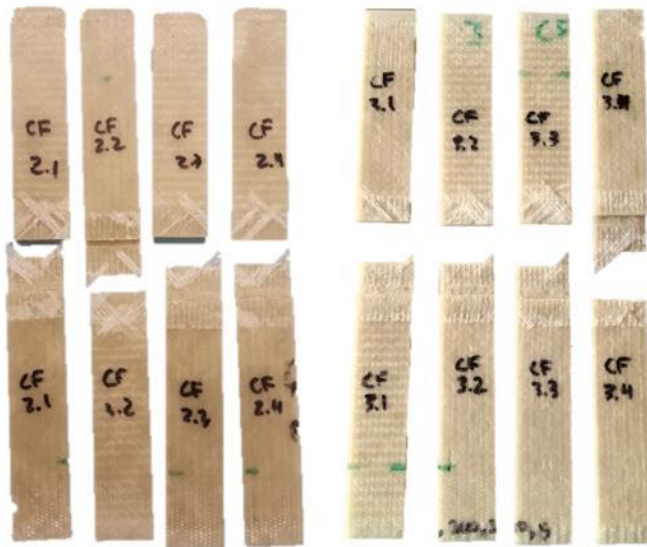
Figure 44: Compoflex® trials CF2 and CF3 all exhibiting cohesive fiber tear failure
