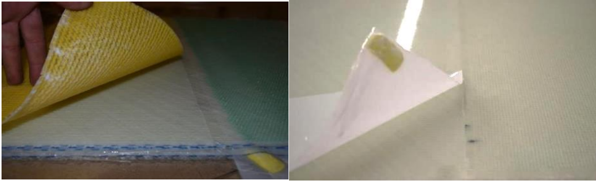
Figure 26: Comparison of Compoflex® (Left) Peel Ply (center) and G-FLOW™ (right) surface textures
