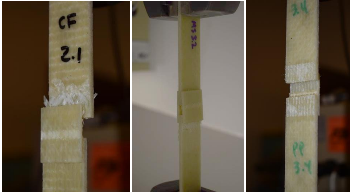
Figure 49: Compoflex®, Mold Surface, and Peel ply coupons illustrating fiber tear during failure
