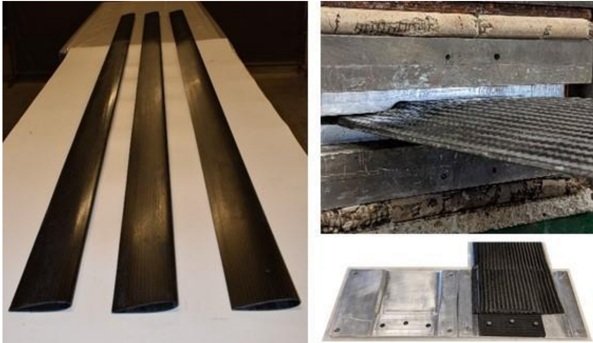
Figure 70: Fusion bonding process showing a) 129" infused airfoils b) compression molding mounting tabs c) completed fusion bond within tooling
