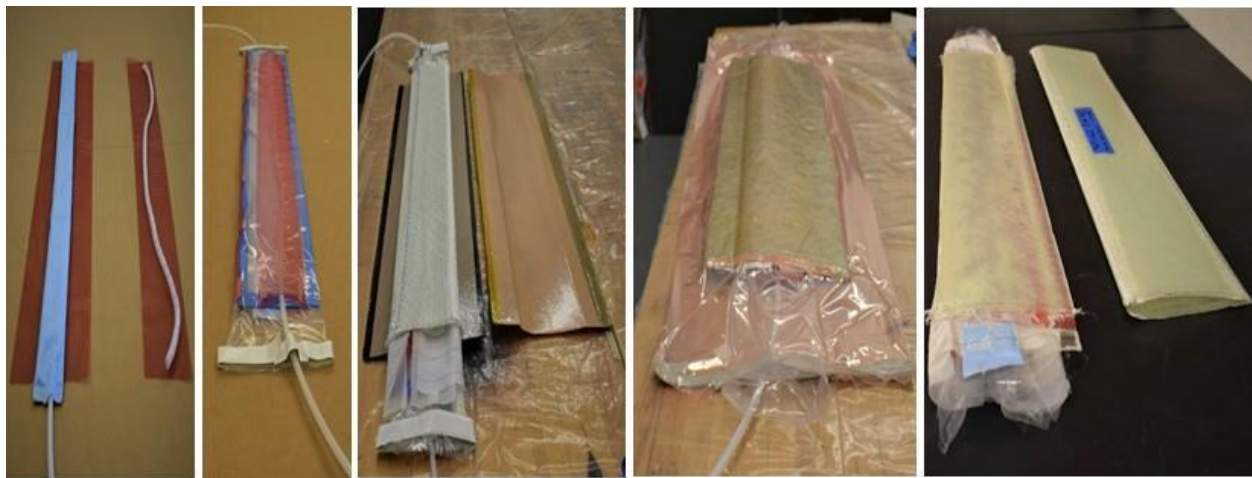
Figure 15: Initial manufacturing process to infuse a 32"-long hollow airfoil cross section
