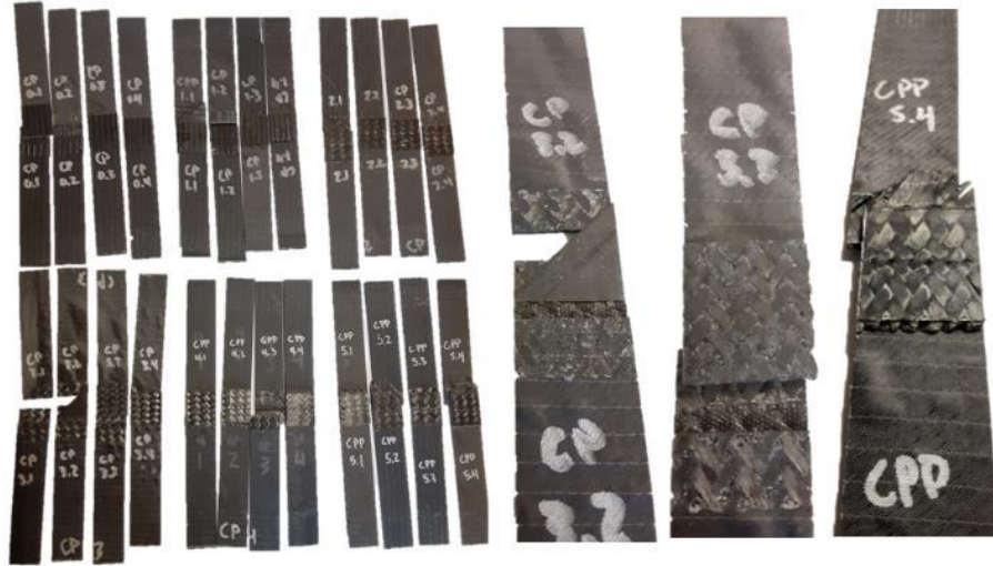
Figure 62: Carbon double lap shear failed adherends
