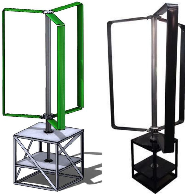
Figure 73: As designed versus as manufactured VAWT prototype
