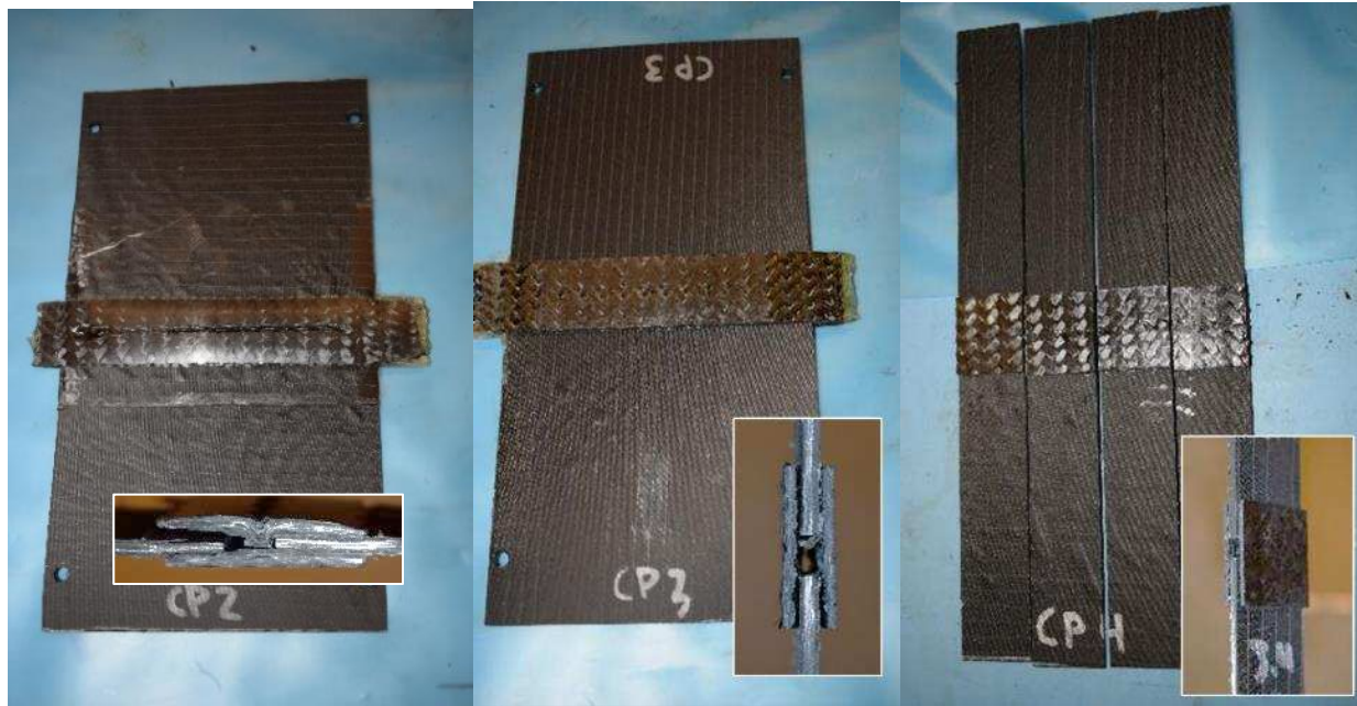
Figure 63: Bonded Carbon Fiber Peel Ply Double lap shear samples and cross section of bonded joint
