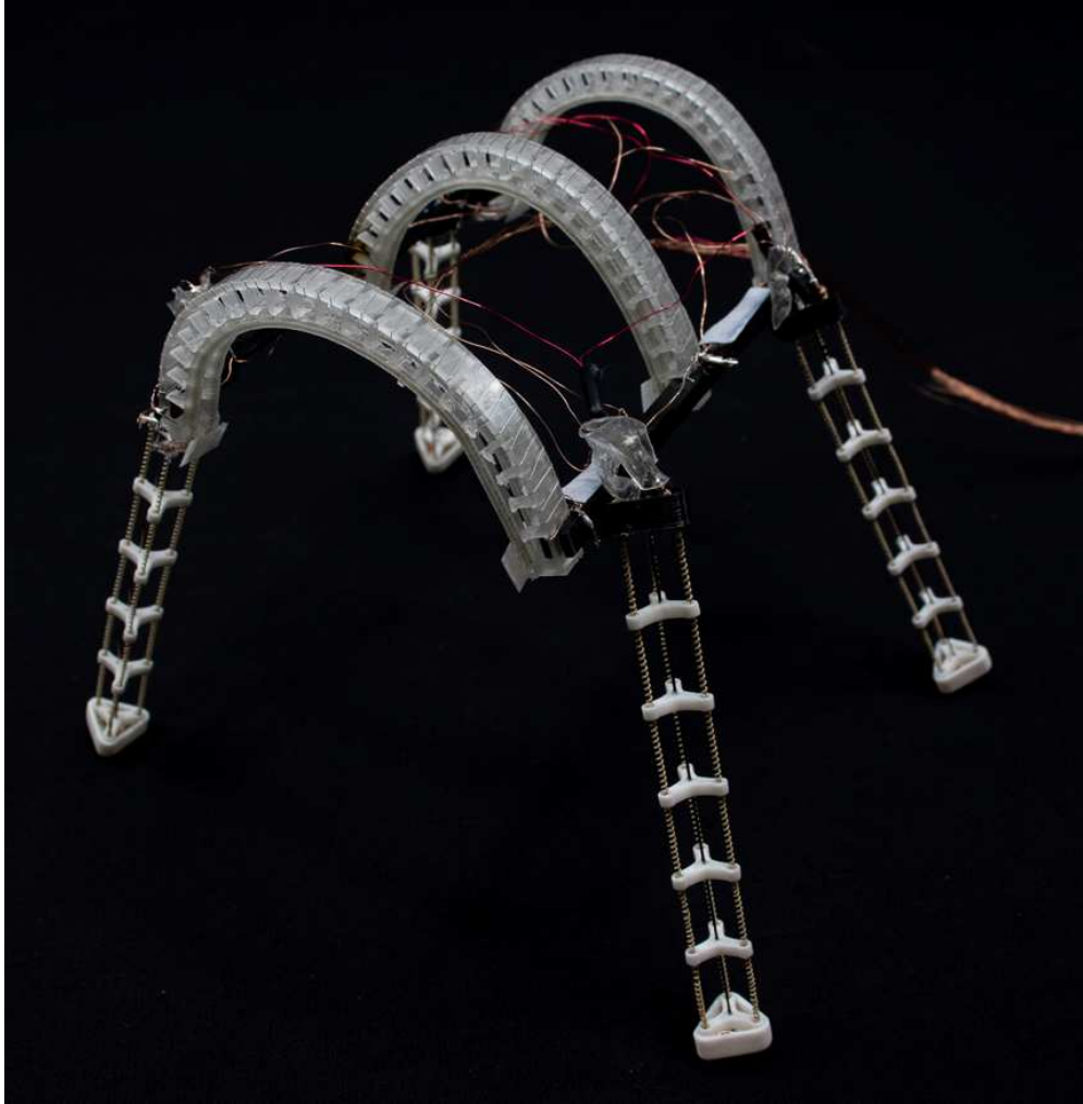
Figure 4.13: The multimodal shape morphing robot in a standing body configuration. The bending angle of the SMM body is approximately 145^\circ , which provides an adequately large base that prevents the robot from toppling over while walking.
