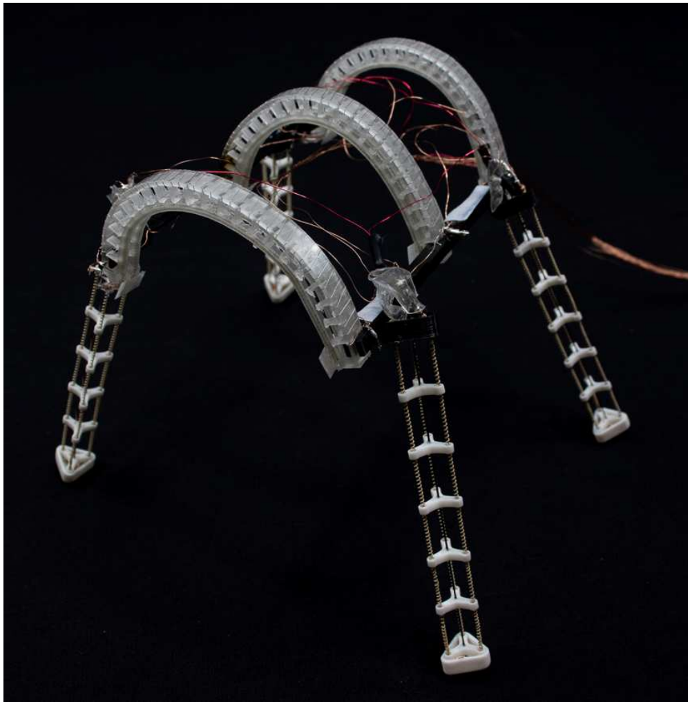
Figure 1.6: The fully assembled modular, multimodal shape morphing robot.
