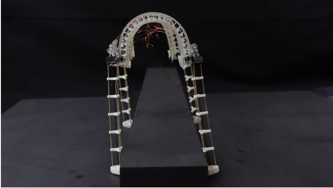
Figure 4.15: The robot gripping a beam in order to realize climbing. The bending angle shown here is approximately 190^\circ so the the robots legs effectively grip the beam.
