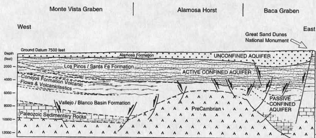
**Figure 3-2 Geologic cross section of the San Luis Valley, Colorado, showing generalized geology and aquifers (Modified from Hanna and Harmon, 1989)**
