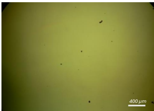
Figure 3.6.3. - Optical microscopy image of the a -SiO 2 thin film after annealing at 600 °C under high humidity conditions.
