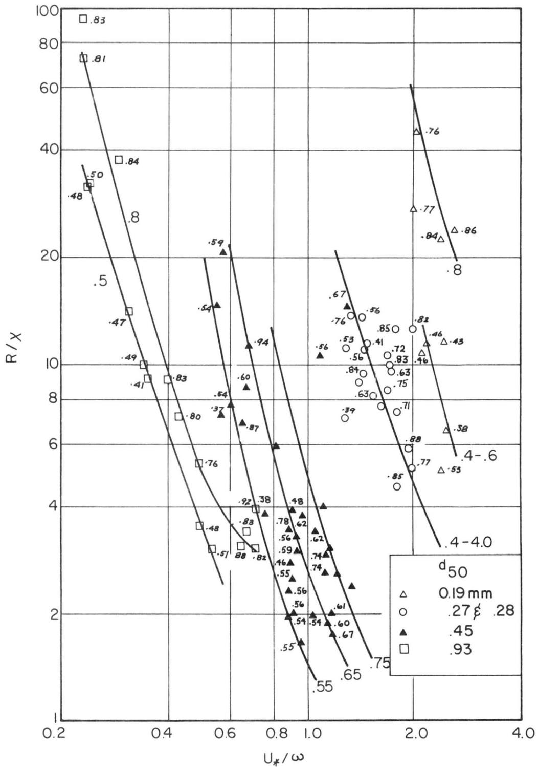
Fig. 25 Variation of  $R/X$  with  $U_*/\omega$  for the dune bed. Hydraulic radius is the third variable.
