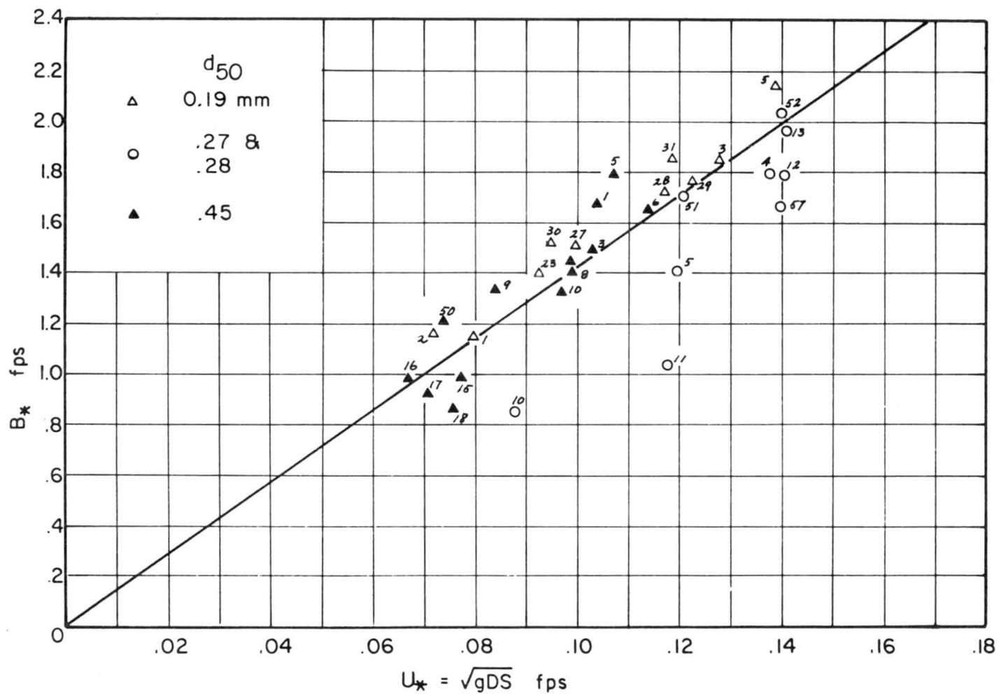
Fig. 12. Relation between the intercept  $B_*$  of the velocity distribution in the vertical and the shear velocity  $U_*$  for the ripple bed configuration. Third variable is run number.
