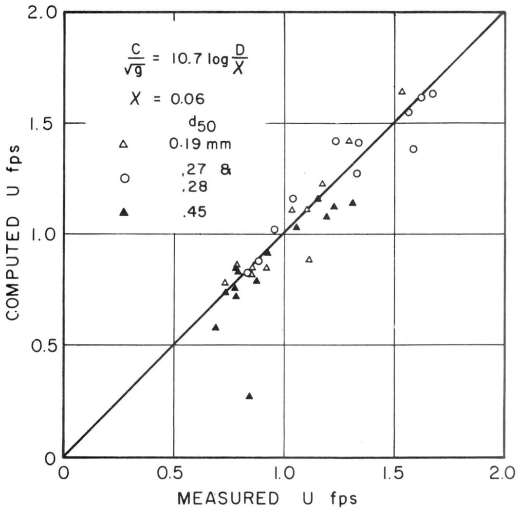
Fig.21 Comparison of the computed velocity with the measured velocity for ripples. (Eq.42)
