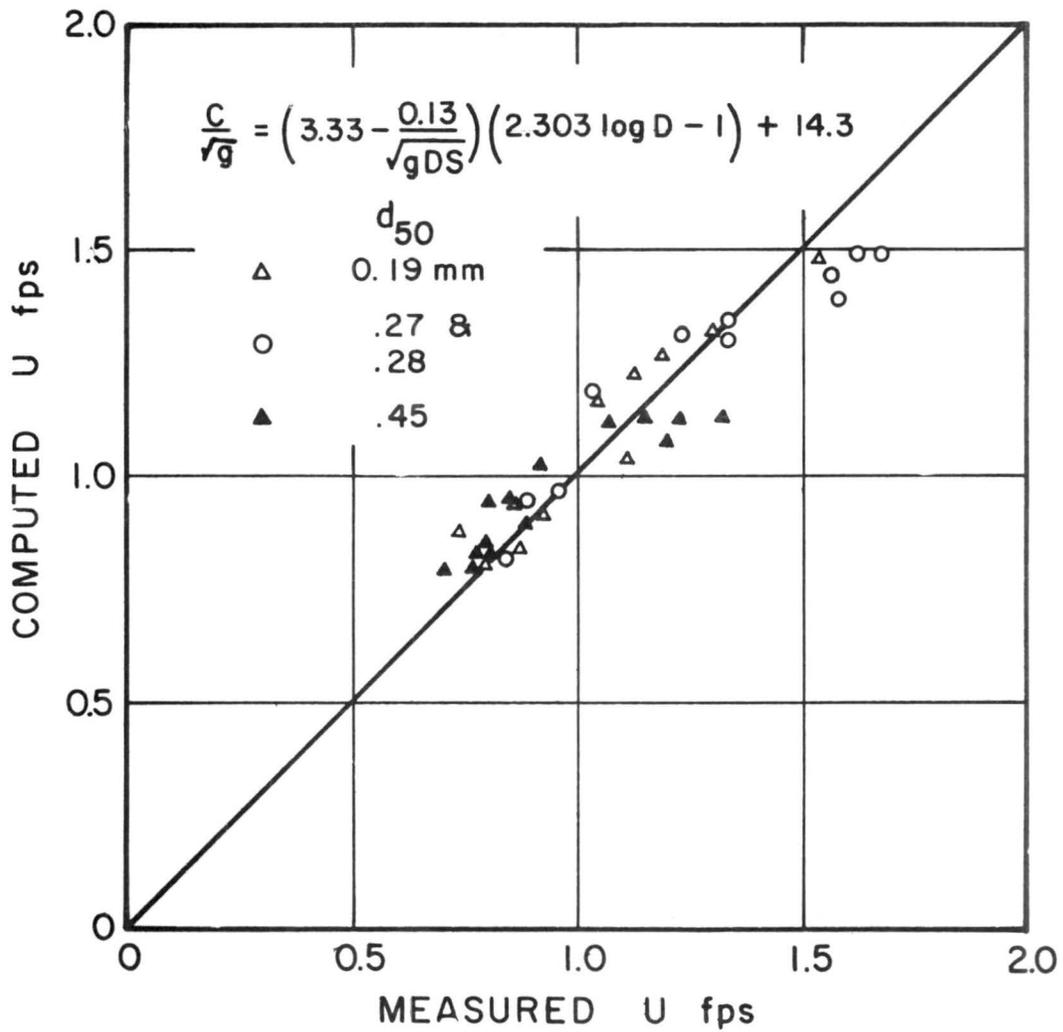
Fig.20 Comparison of the computed velocity with the measured velocity for ripples. (Eq.41)
