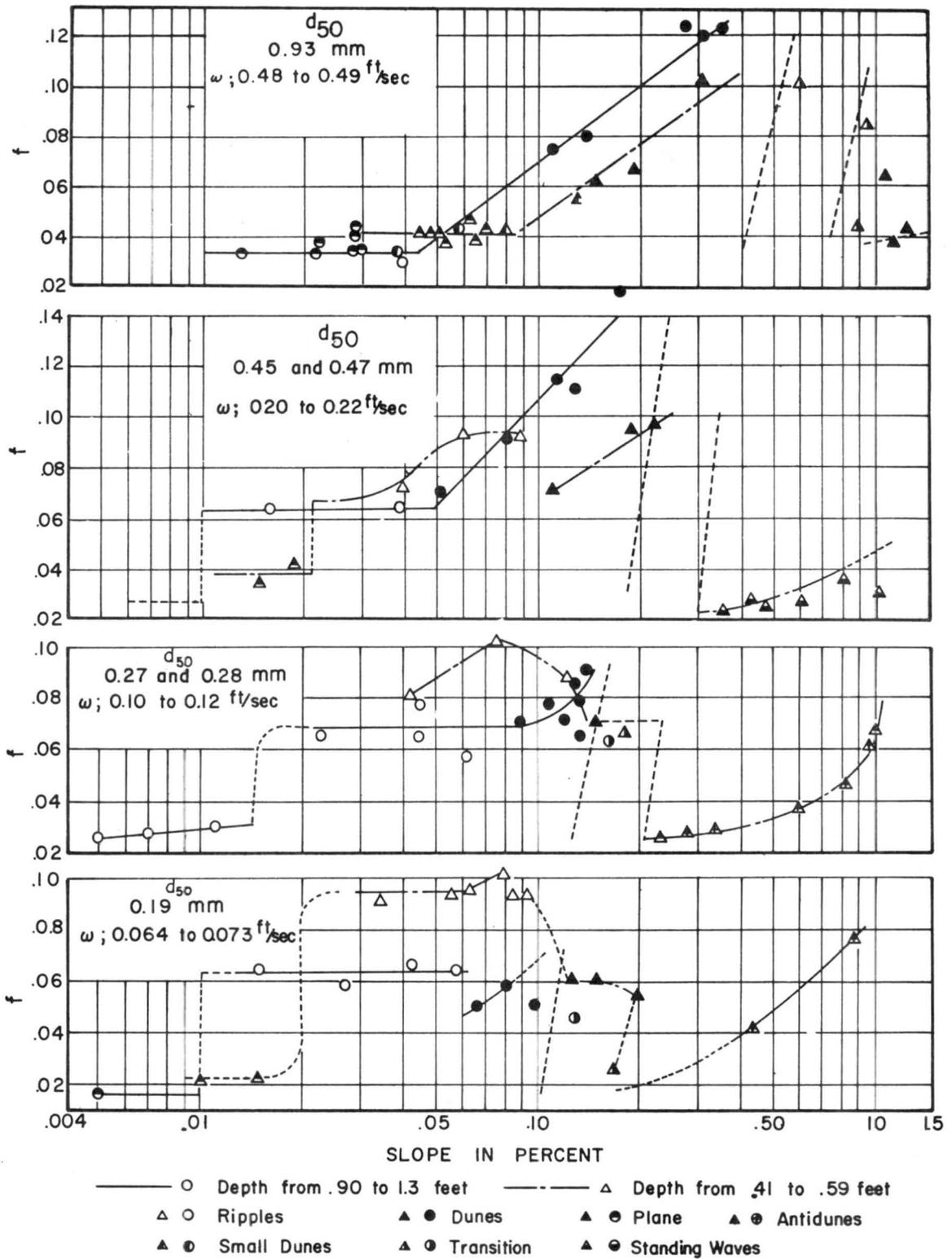
Fig. 4 Change in Darcy-Weisbach  $f$  with slope, depth and fall velocity of the bed material, 8 ft. flume data. ( $f = 8 / (C/\sqrt{g})^2$ )
