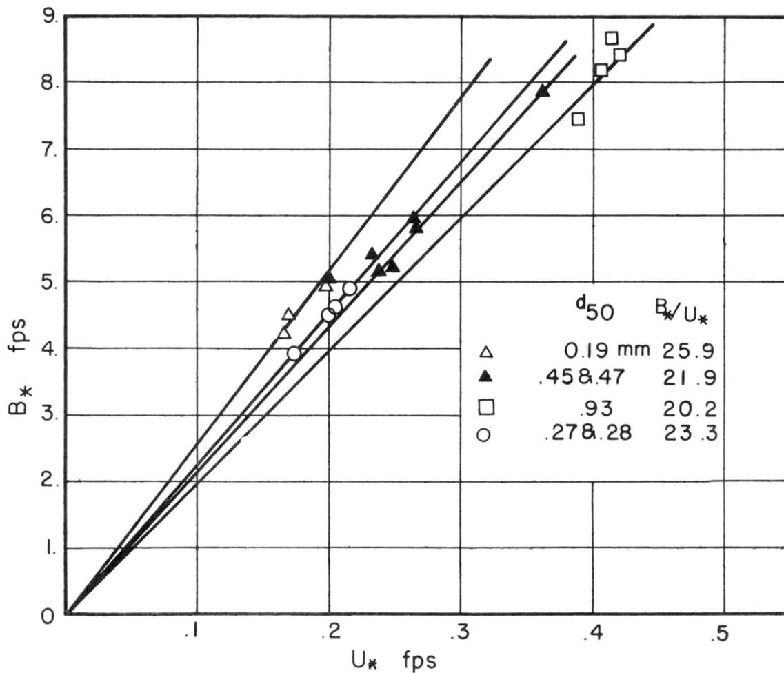
Fig. 8 Relation between the intercept  $B_*$  of the velocity distribution in the vertical with  $U_*$  for plane bed flow with sediment movement
