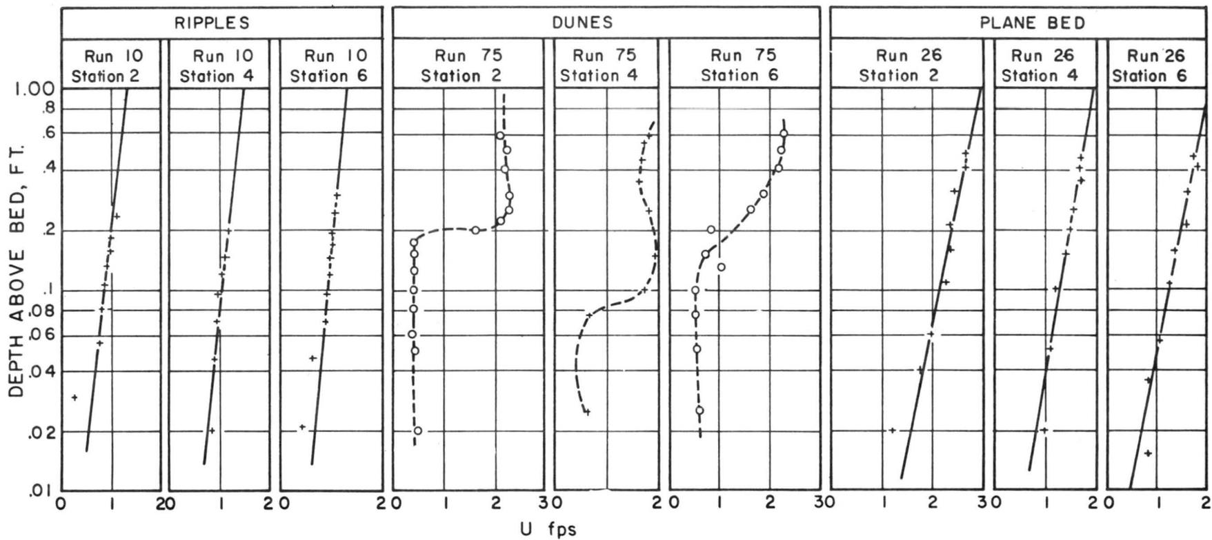
Fig. 6 Typical velocity distribution curves.
