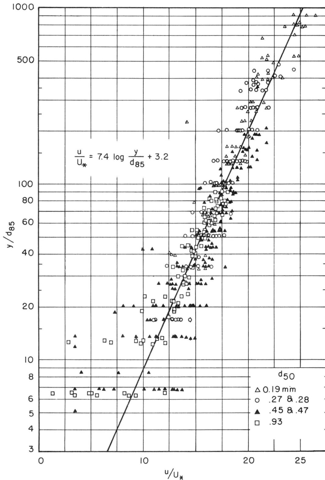
Fig.9 Relation between  $u/U_*$  and  $y/d_{85}$  for the plane bed with sediment transport in the 8ft. flume
