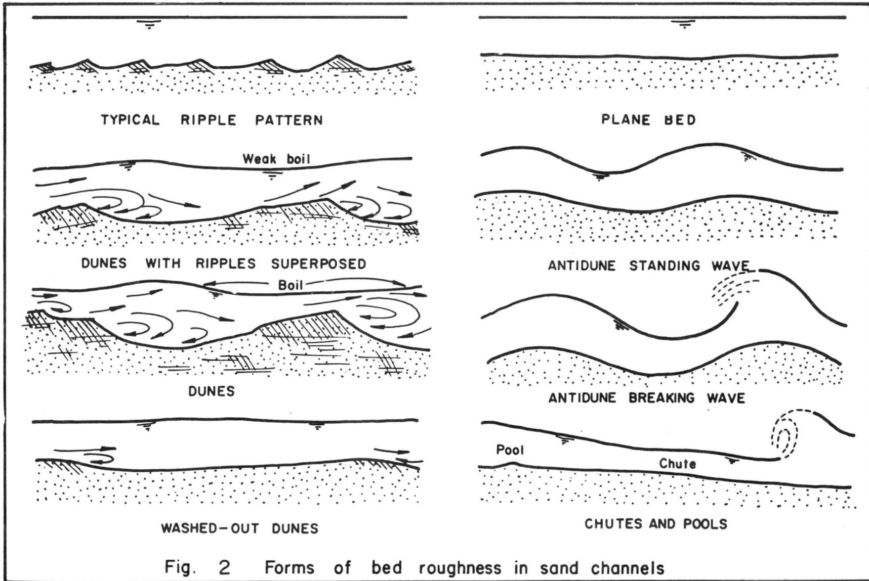
Fig. 2 Forms of bed roughness in sand channels
