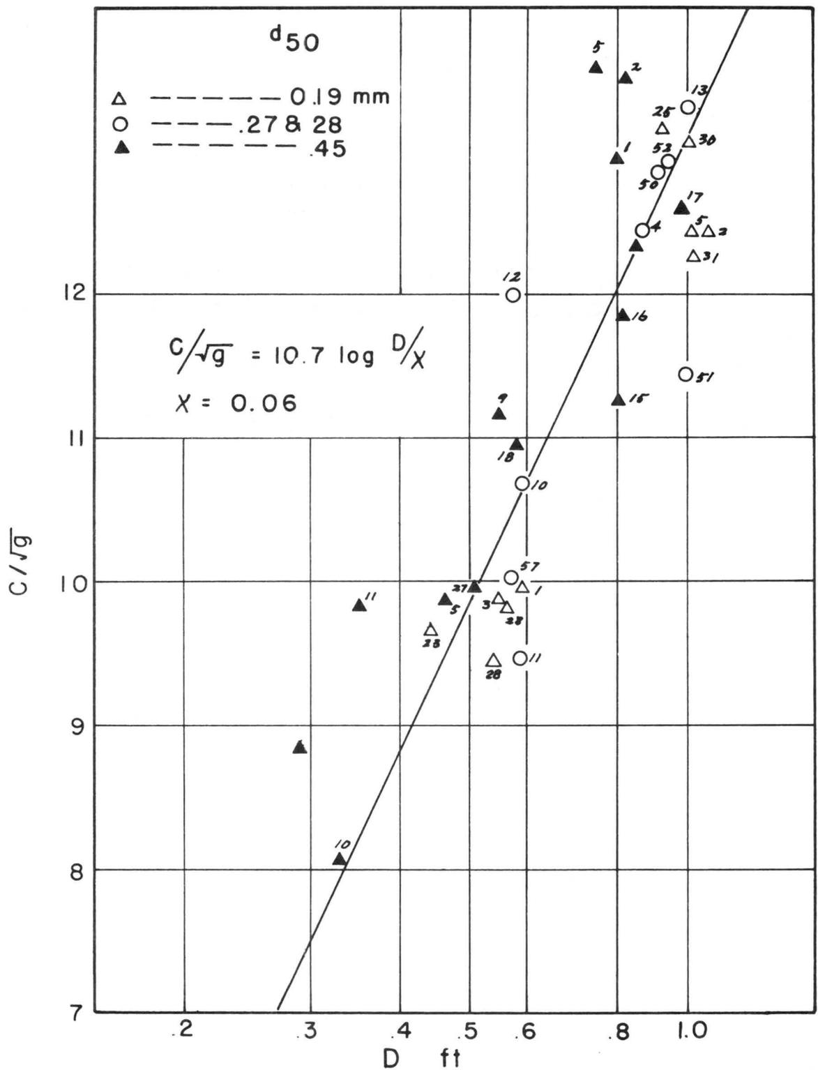
Fig. 13. Variation of  $C/\sqrt{g}$  with depth of flow for the ripple bed configuration. Third variable is run number.
