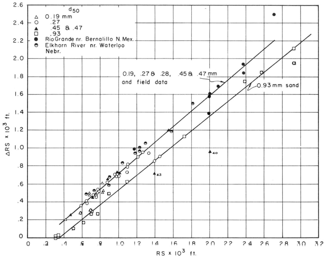
Fig.27 Relation between  $\Delta RS$  with  $RS$  for the 8 ft. flume and field data.
