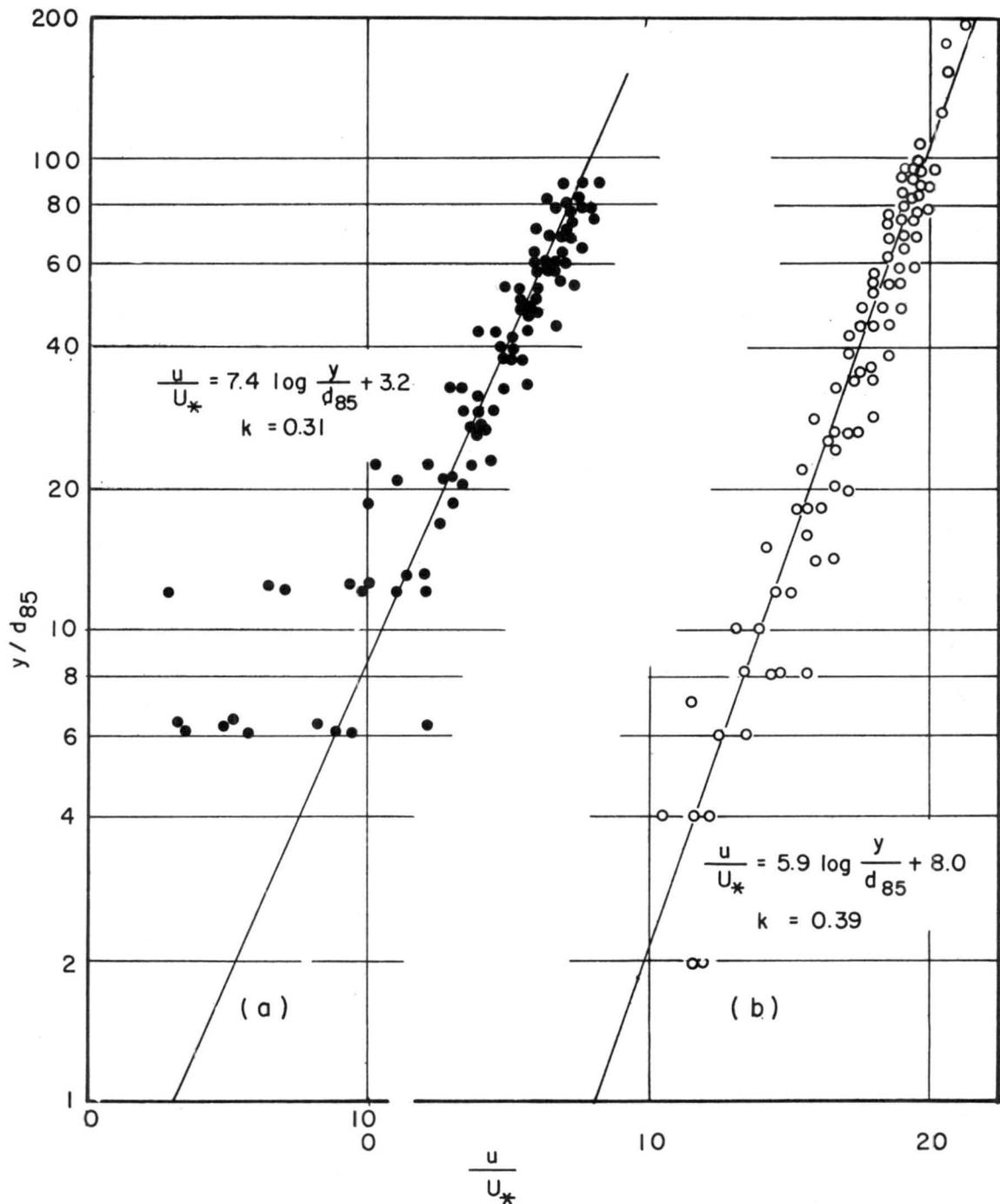
Fig. 10 Comparison of the relation between  $u/U_*$  and  $y/d_{85}$  for plane bed flow with (a) and without (b) appreciable sediment movement (0.93 mm sand)
