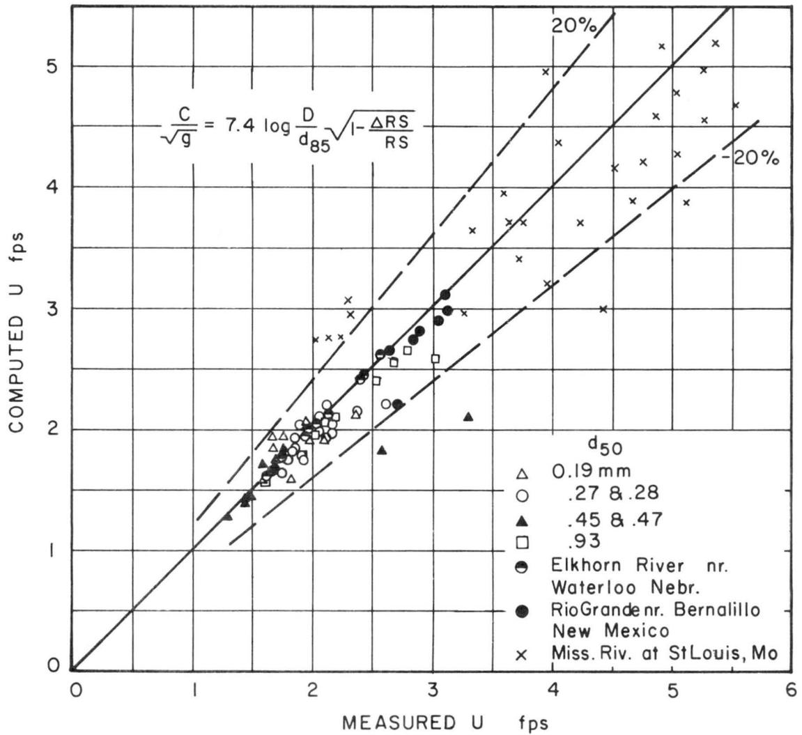
Fig.29 Comparison of computed velocity with the measured velocity for dunes using the  $\Delta RS$  method.
