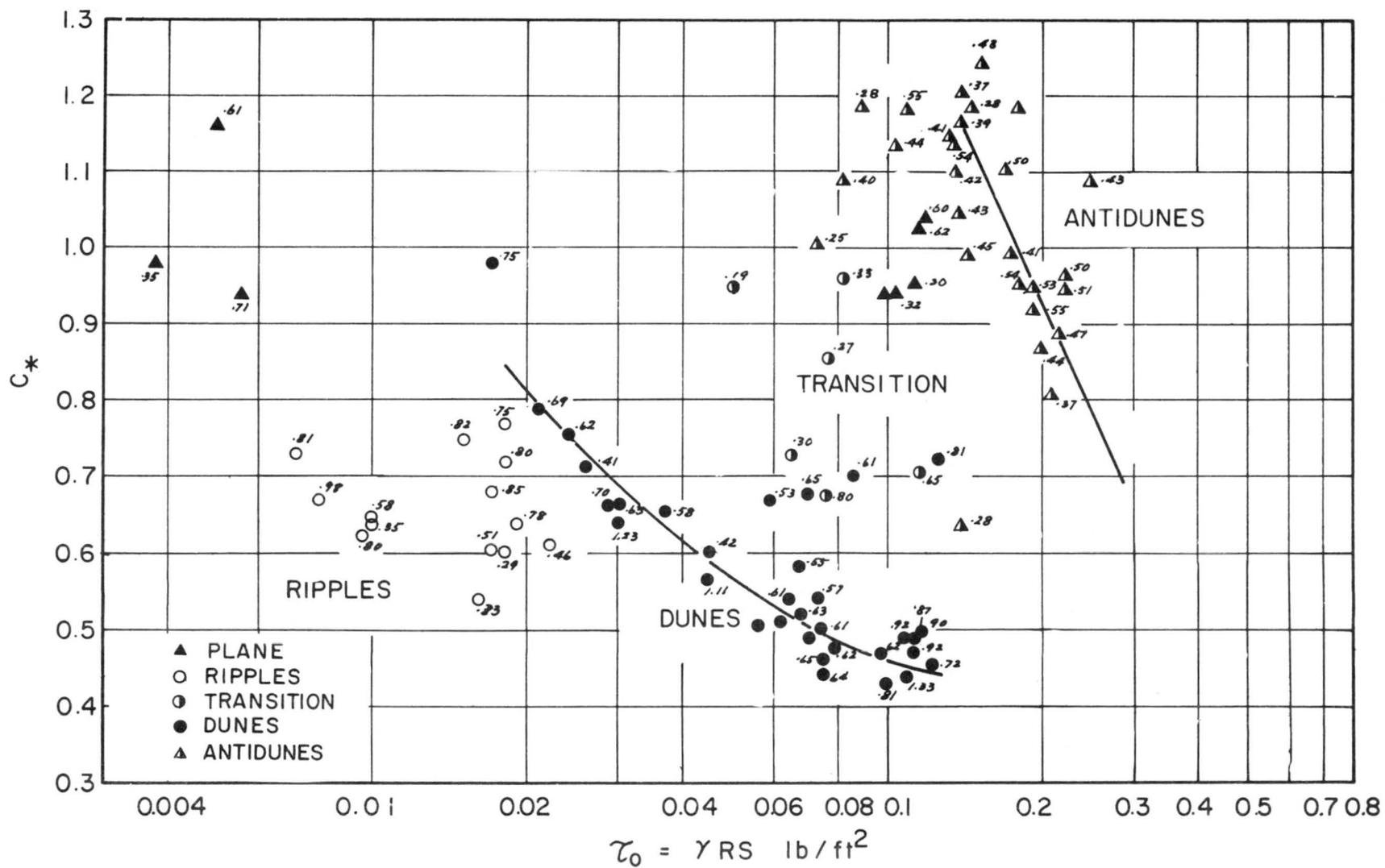
Fig. 17. Relation between  $C_*$ ,  $\tau_0$  and depth for 0.45 and 0.47 mm sand. Third variable is depth of flow.
