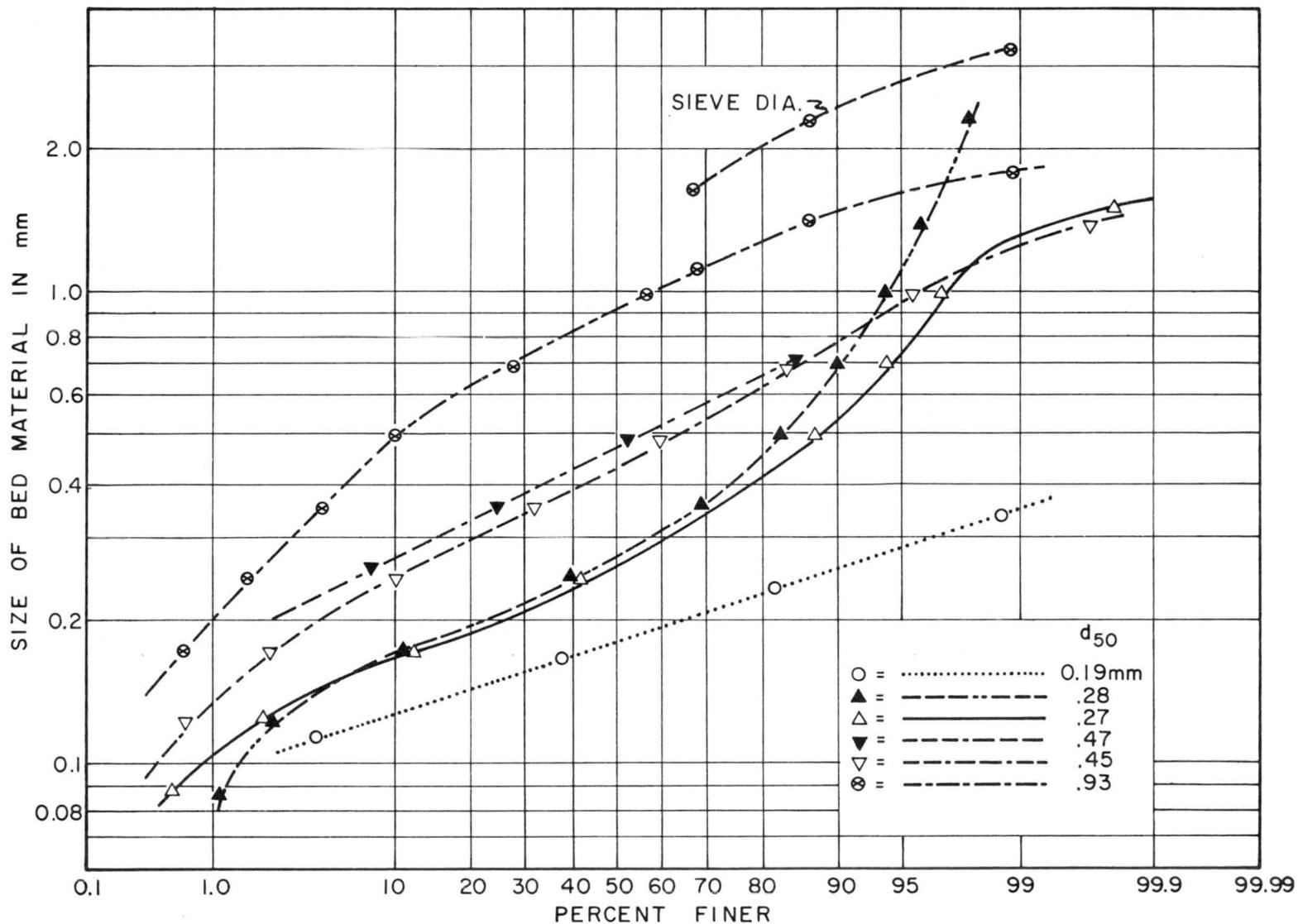
Fig. 1 Size distribution curves for the sands used in the 8ft flume.
