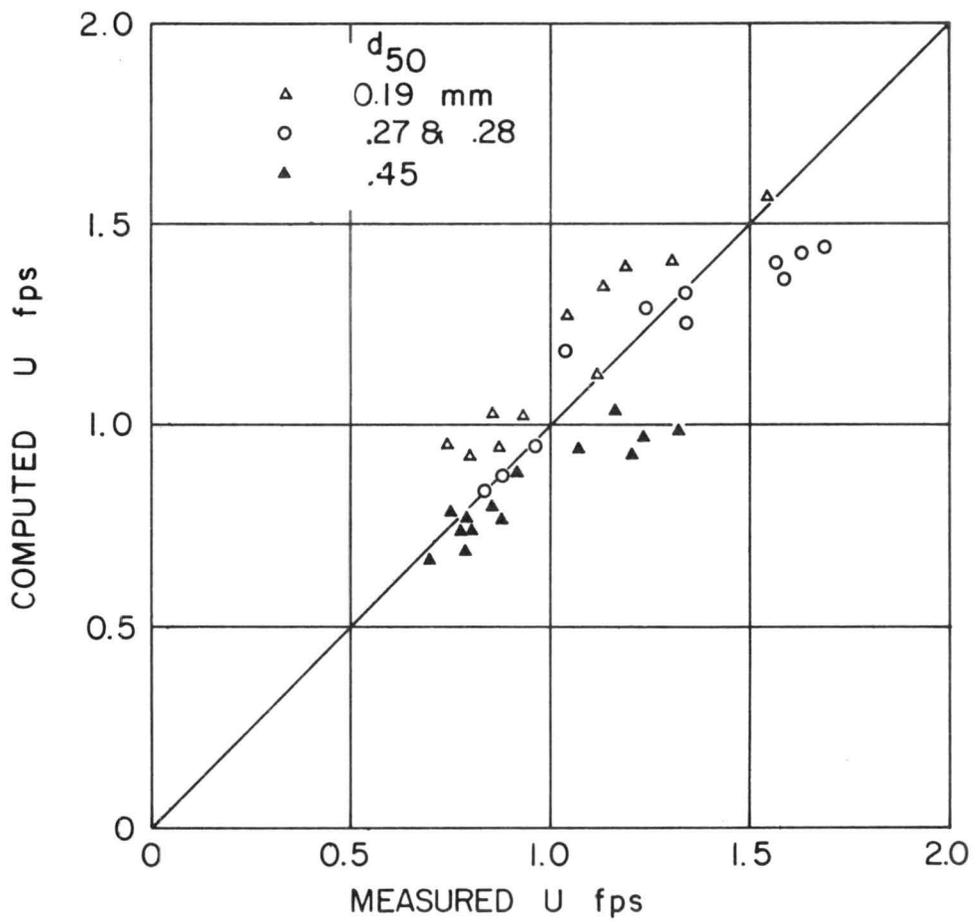
Fig. 23 Comparison of the computed velocity with the measured velocity (eq. 36)
