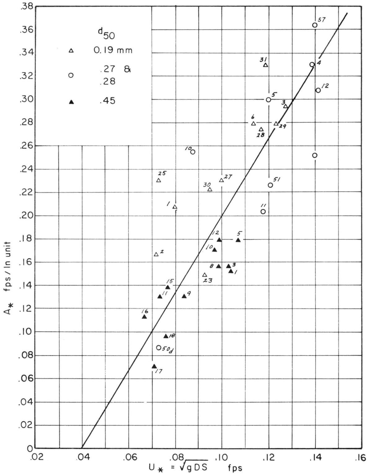
Fig. 11. Relation between the slope  $A_*$  of the velocity distribution in the vertical and the shear velocity  $U_*$  for ripple bed configuration. Third variable is run number.
