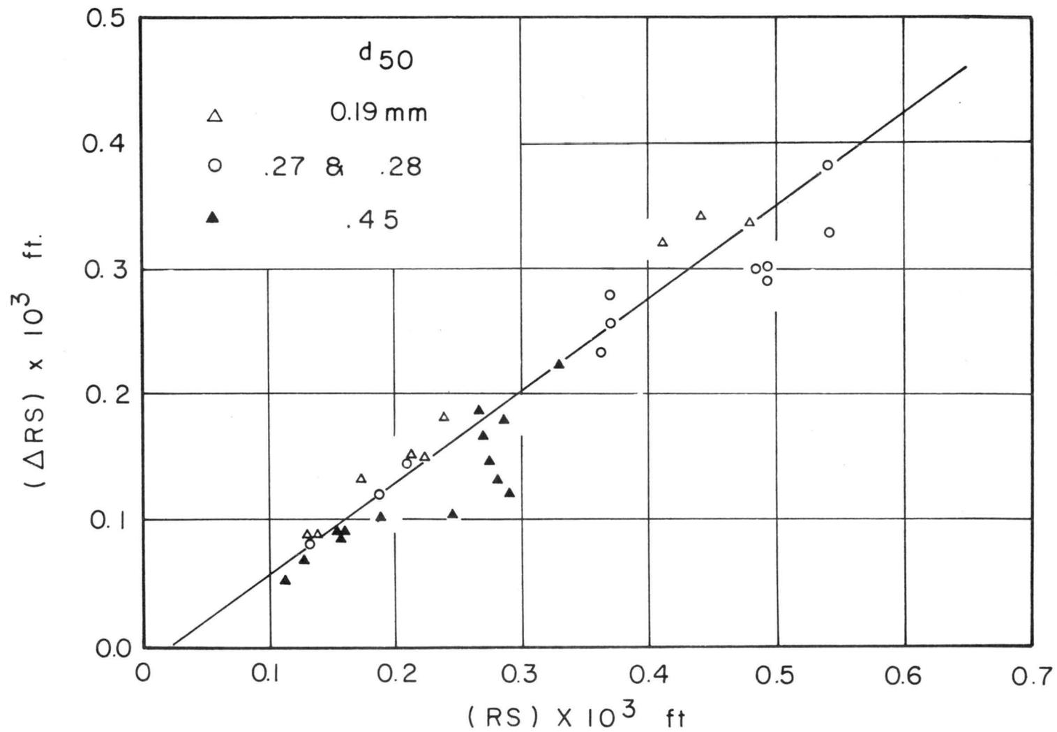
Fig. 22 Relation between  $\Delta RS$  and  $RS$  for ripples
