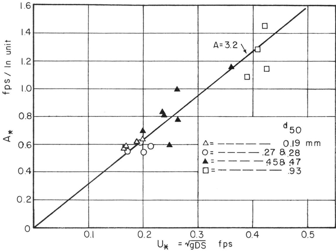
Fig.7 Relation between the slope  $A_*$  of the velocity distribution in the vertical and the shear velocity  $U_*$  for plane bed flow with sediment movement.
