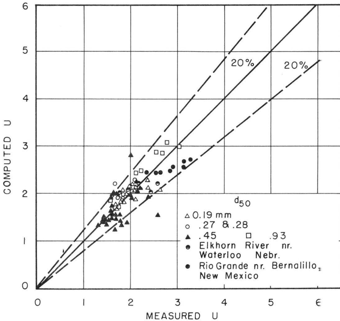
Fig 26 Comparison of the computed velocity with the measured velocity. (eq. 43)
