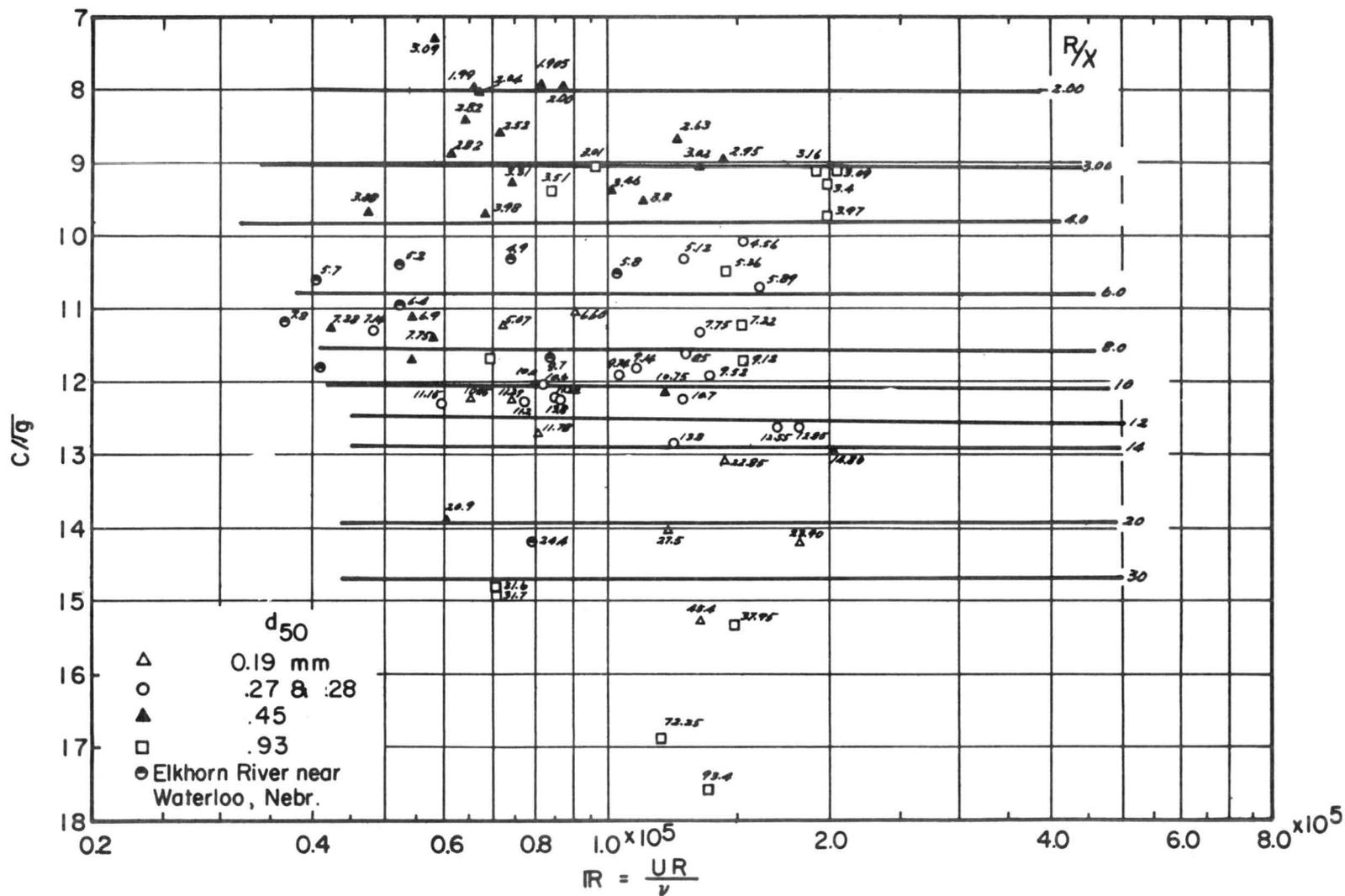
Fig. 24 Relation between  $C/\sqrt{g}$ ,  $IR$  and  $R/x$  when  $C/\sqrt{g} = 5.75 \log R/x + 6.25$ .
