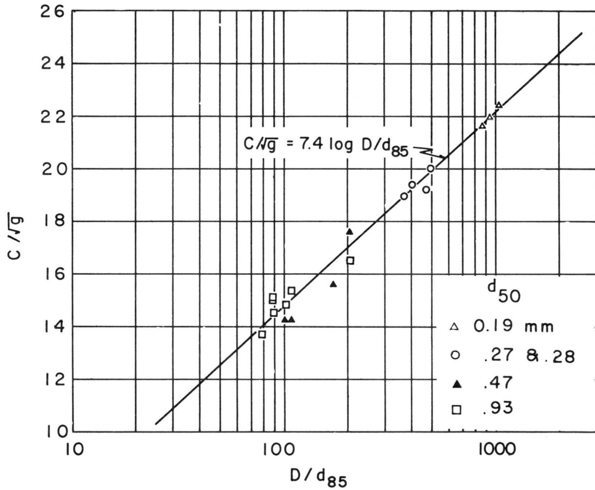
Fig. 19 Variation of  $C/\sqrt{g}$  with  $D/d_{85}$  for plane bed with sediment movement.
