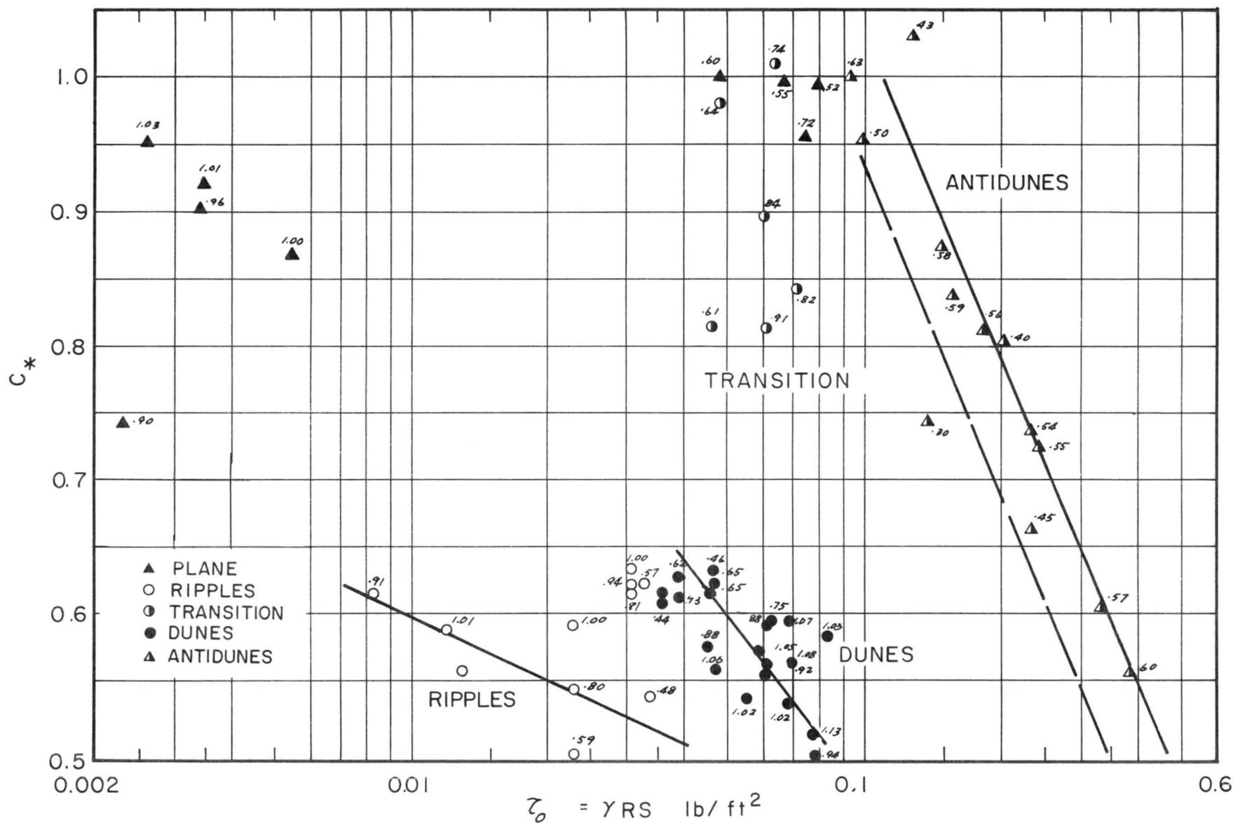
Fig. 16. Relation between  $C_*$ ,  $\tau_0$  and depth for 0.27 and 0.28 mm sand. Third variable is depth of flow.
