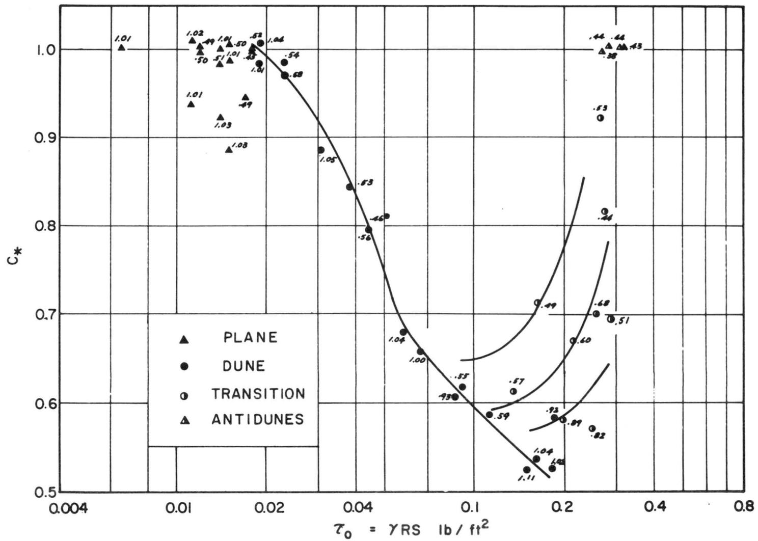
Fig. 18. Relation between  $C_*$  and  $\tau_0$  depth for the 0.93 mm sand. Third variable is depth of flow.
