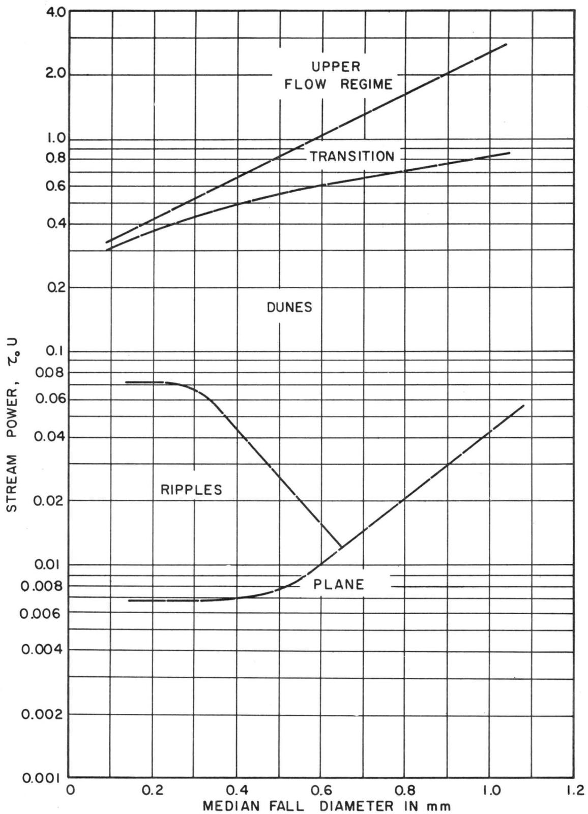
Fig. 5 Relation between stream power, median fall diameter and bed configuration.
