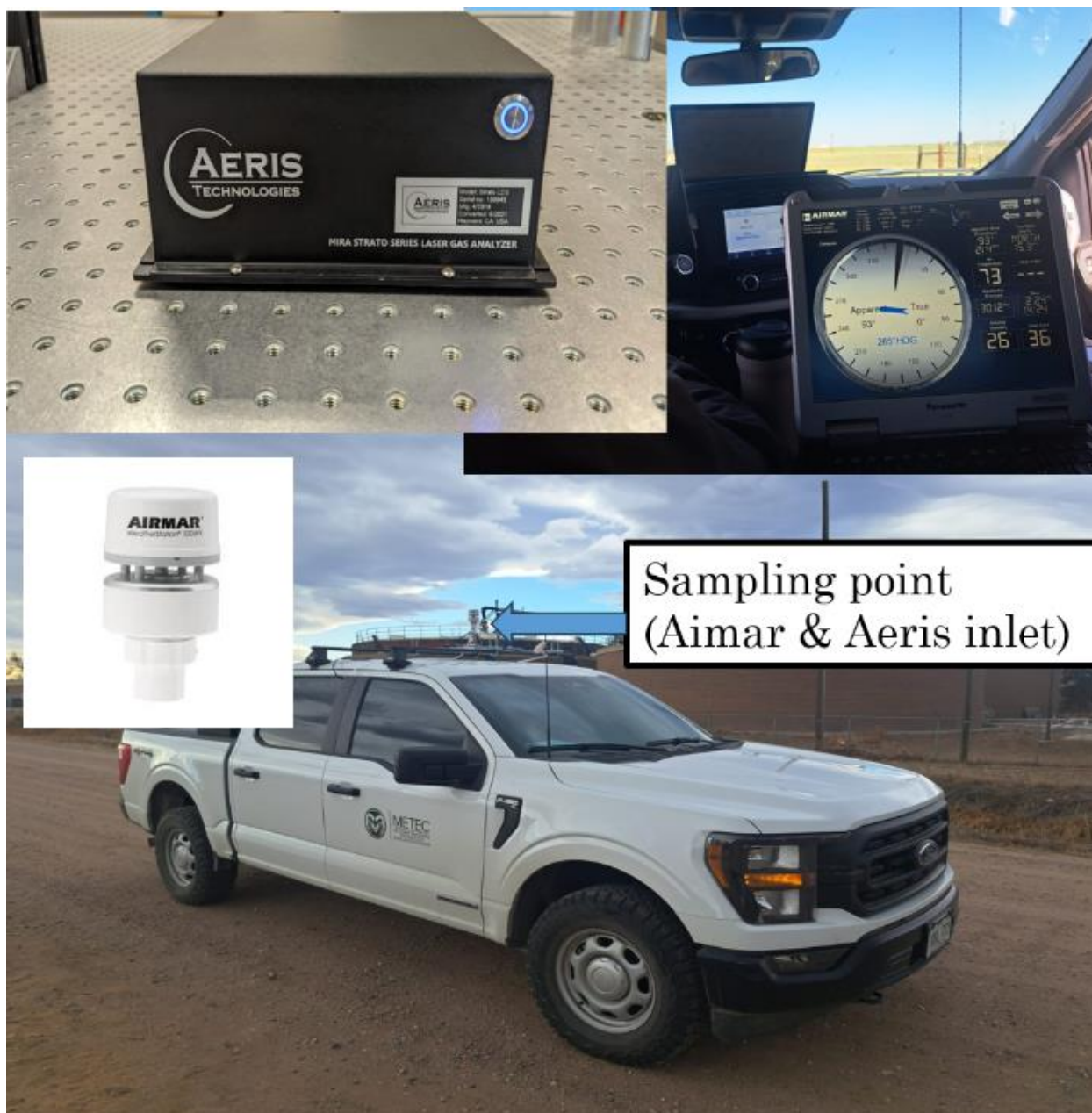
Figure A23. Instrument setup. Top left: AERIS Strato analyzer (sampling at 1 Hz). Top right: Airmar instrument software displaying meteorological conditions. Center: Airmar 150 WX instrument (sampling at 1 Hz). Bottom: METEC truck with the AERIS inlet tubing collocated with the Airmar instrument.
