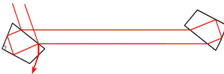
**Figure 6.1: Schematic of Brewster prism cavity.**
