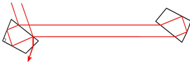
**Figure 6.1: Schematic of Brewster prism cavity.**
