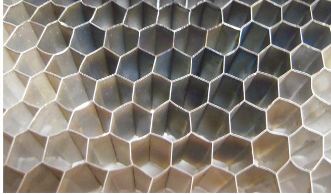
**Figure 3.8: Aluminum honeycomb structure.**
