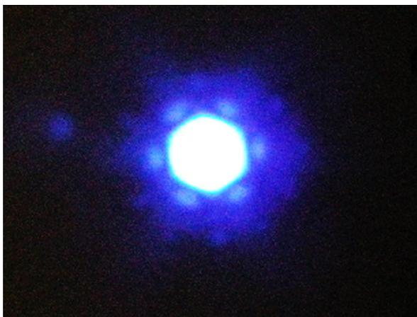
Figure 4.5: Photograph of single-mode output beam from PCF.
