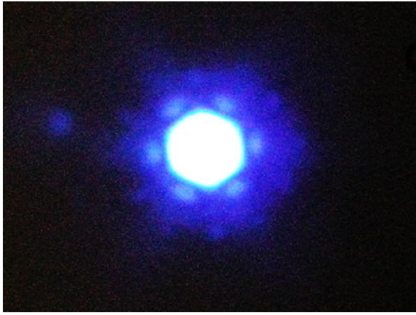
**Figure 4.5: Photograph of single-mode output beam from PCF.**
