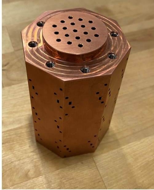
Figure 4.51: One machined waveguide feed horn block. These blocks are constructed with one inch sides to interface with the frequency converter modules. The blocks are 2.61" wide at their longest point, and 3.88" in height from their base to the top of the cylindrical extrusion.
