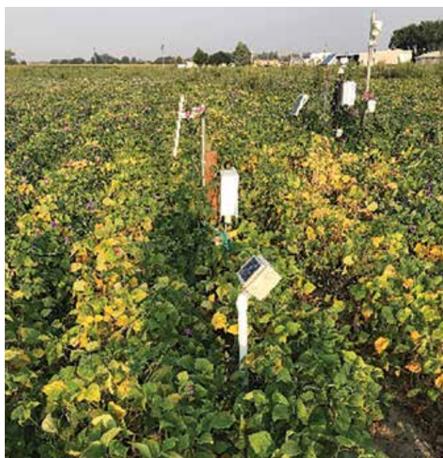
Soil moisture sensor instrumentation in a field of dry beans. Photo by Blake Osborn.
