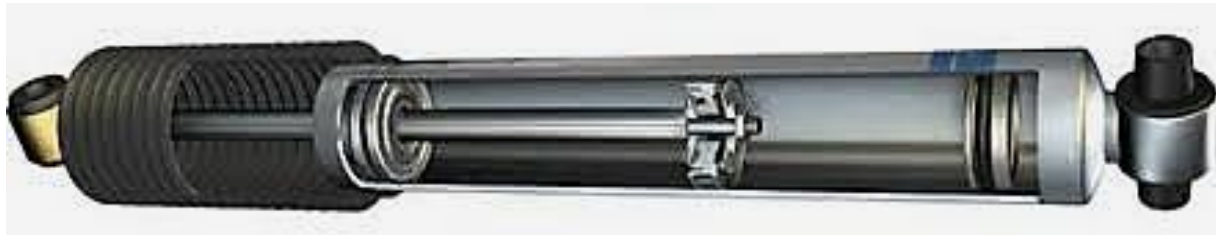
Figure 3. 2: Single Tube Conventional damper system[6]
