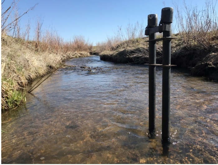
Figure 3-2 Photograph of piezometer nest deployed in stream.
