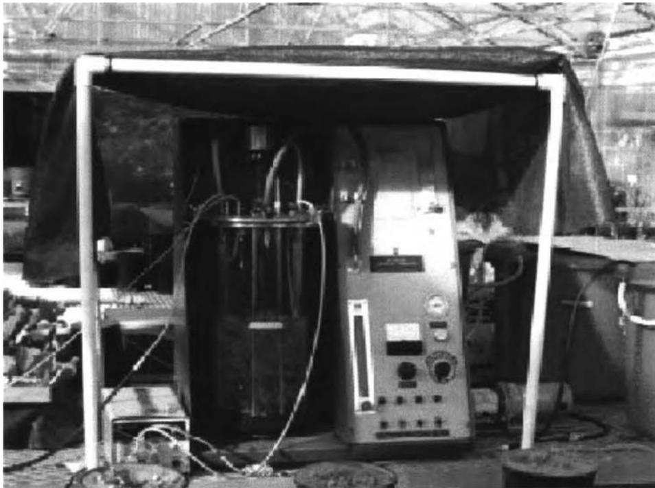
**Figure 5.** The 14-L continuous stirred tank reactor (CSTR) covered with a shade.
