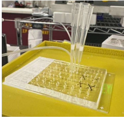
Figure 35: Droplet Collection Process Utilizing Cut, Gel-Loading Pipette Tips
