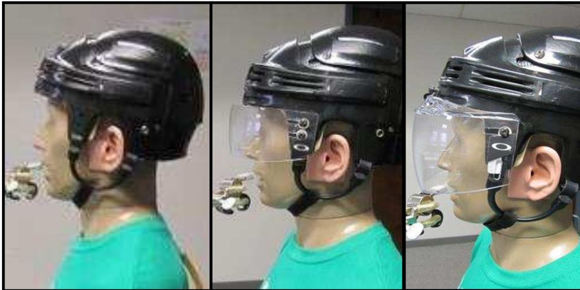
**Figure 5.6: Hockey helmet configurations (left to right): a. Bauer<sup>®</sup> 4500 hockey helmet without a visor; b. Bauer<sup>®</sup> 4500 hockey helmet with a 2.75" Oakley<sup>®</sup> VR904 modified straight small visor with slots; c. Bauer<sup>®</sup> 4500 hockey helmet with a 4.0" Oakley<sup>®</sup> VR924 CLE pro straight visor with vents**
