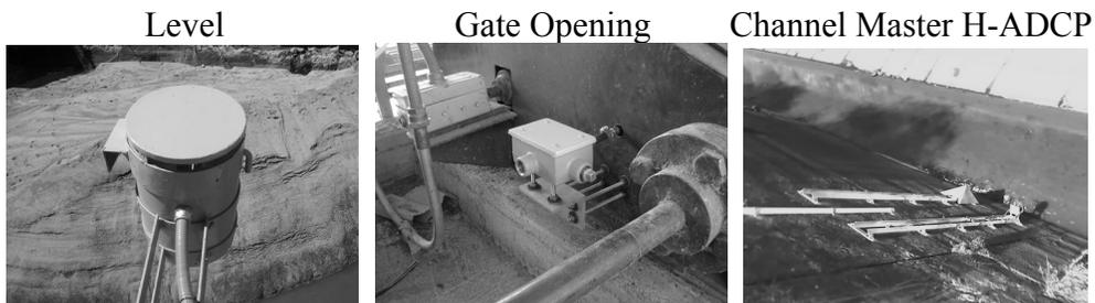
Figure 3. Level and Gate Position Sensors
