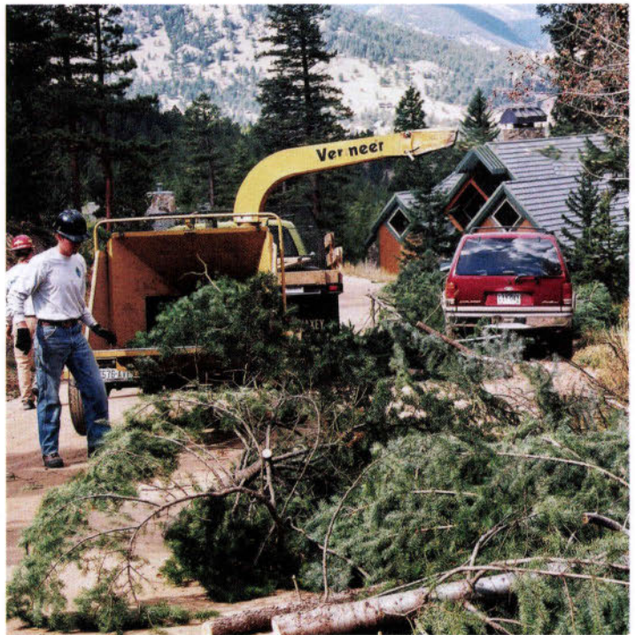
Chipping is an effective method of slash disposal, but it is very labor-intensive and expensive.
