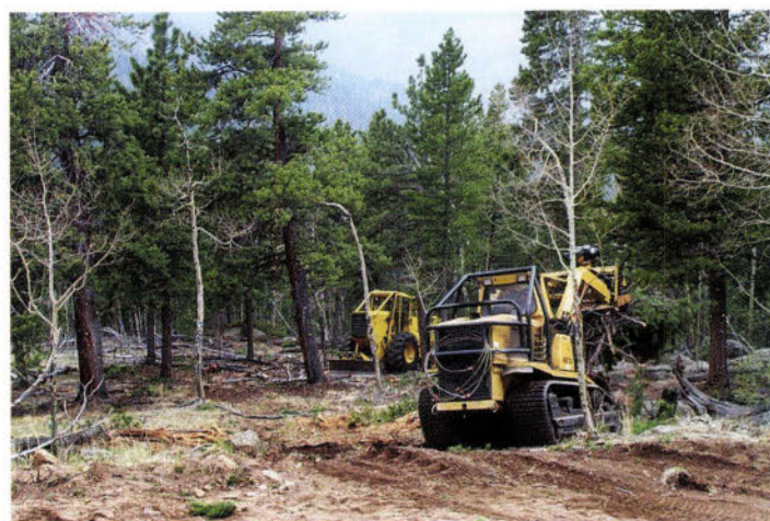
Where markets for timber do not exist or trees are too small, equipment can grind, mulch, or masticate trees to accomplish desired treatments.
