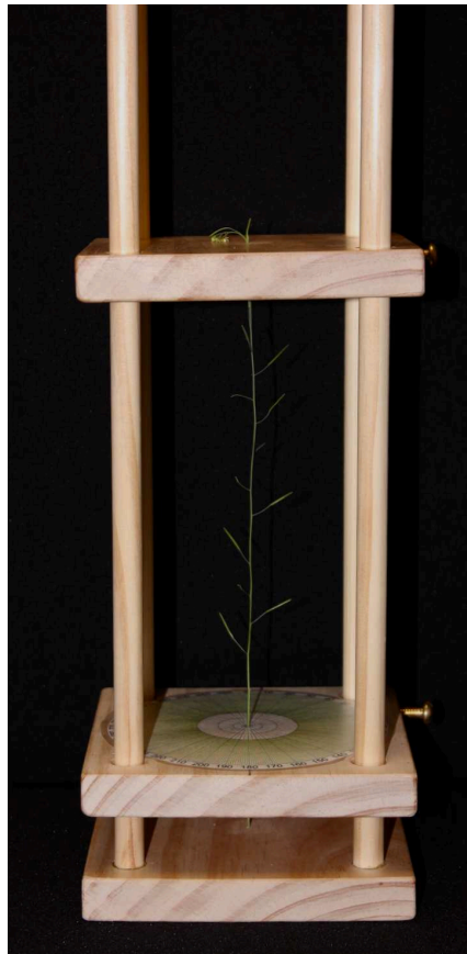
Figure 3.2: Device used to measure silique divergence angles for phyllotactic analysis.
