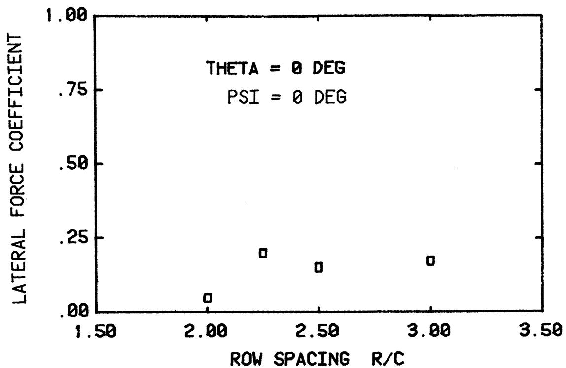
Figure 16a. Effect of row spacing on collector loads
