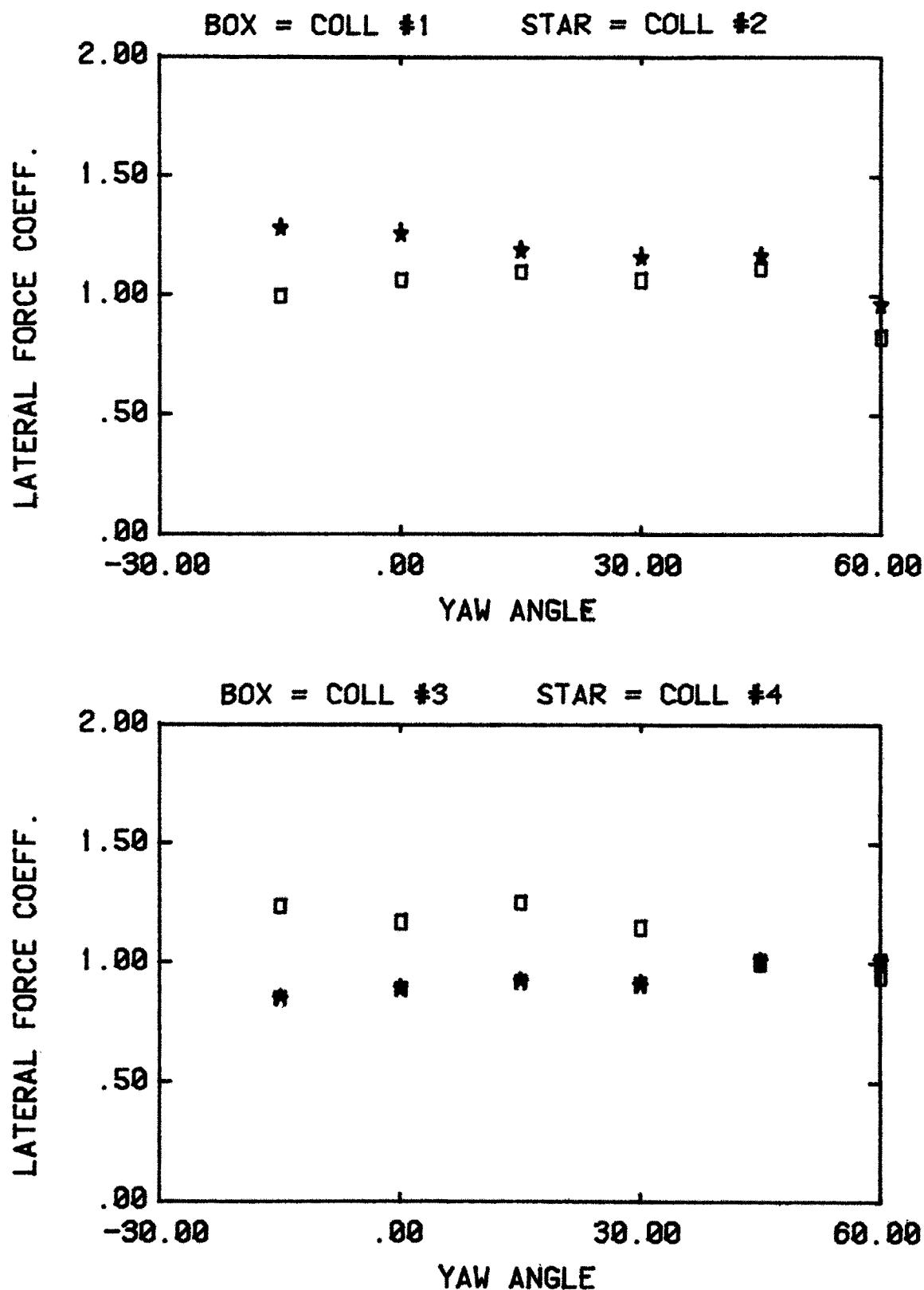
Figure 13b. Variation of single collector loads with yaw angle for HCL/C=K<sub>I</sub>, (configurations 1-4).
