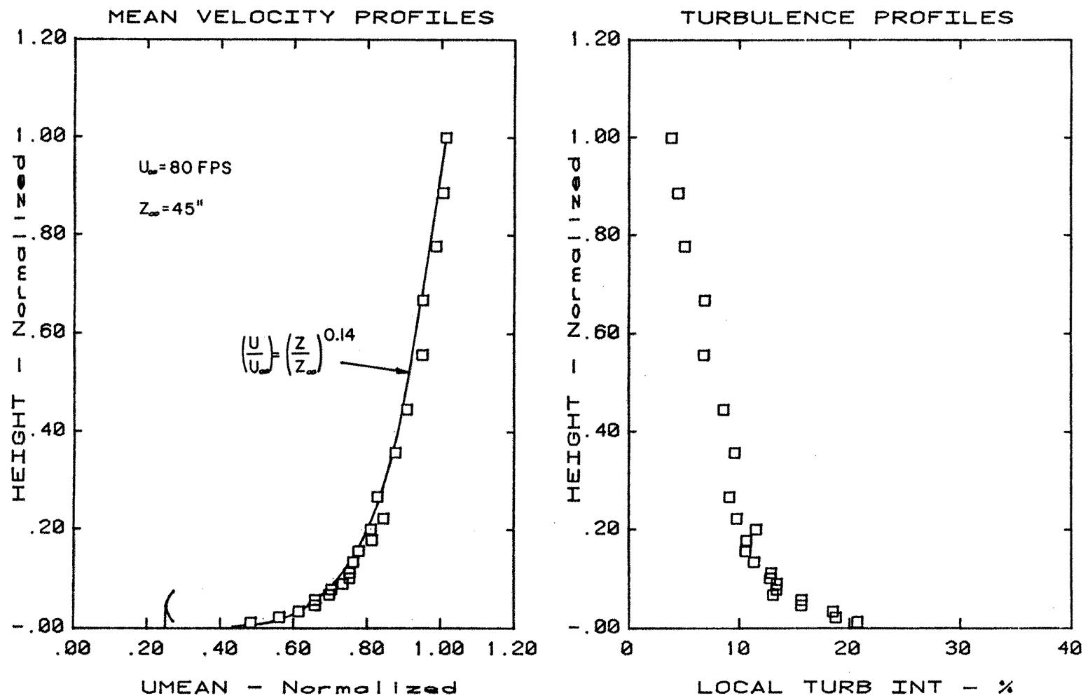
Figure 8. Approach velocity and turbulence profile.
