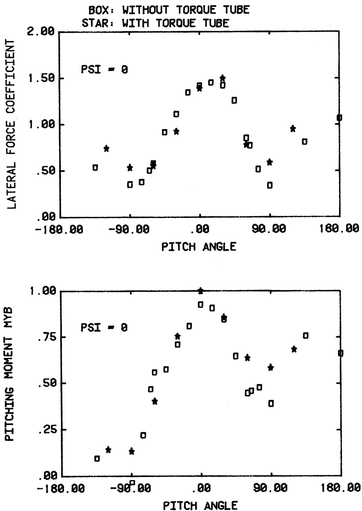
Figure 18a. Effect of torque tube on collector 1 loads.
