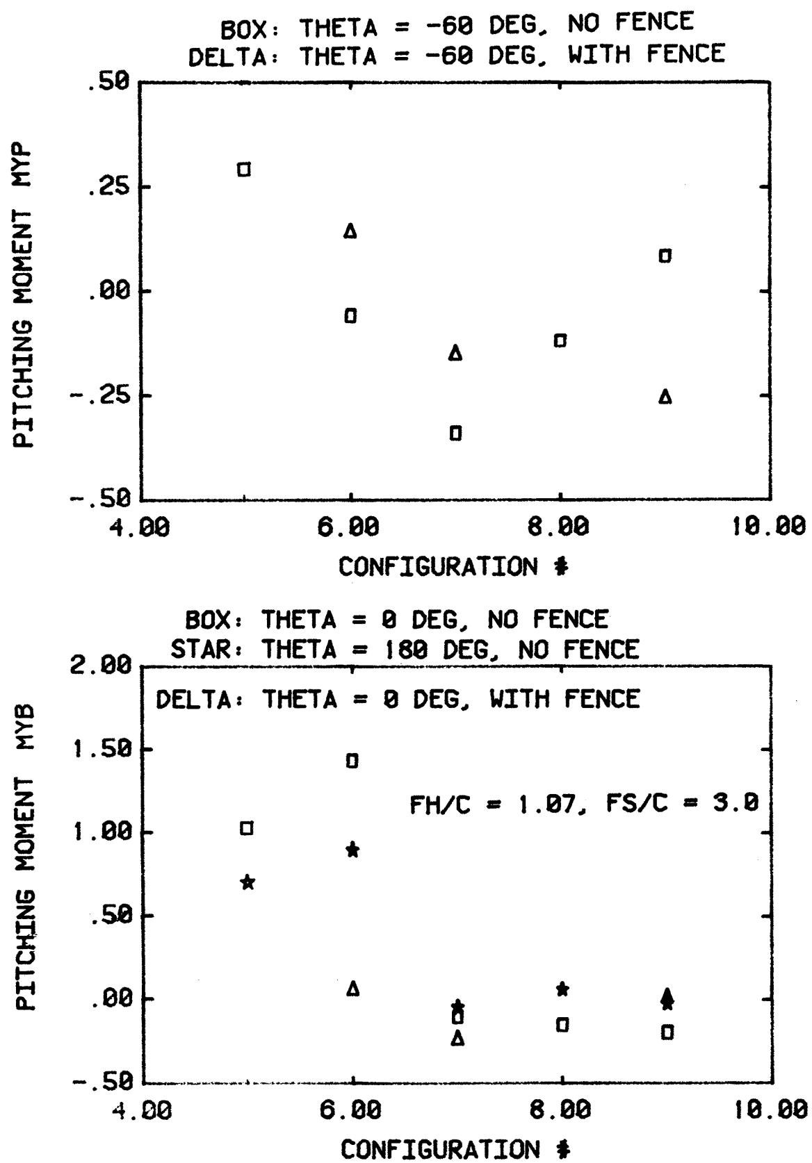
Figure 17c. Influence of array field configuration and fences on collector loads.
