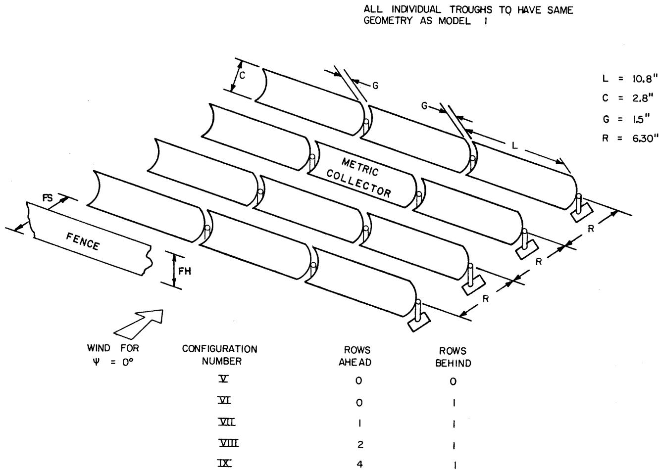
Figure 6 a. Collector in arrays for configurations 5-9.
