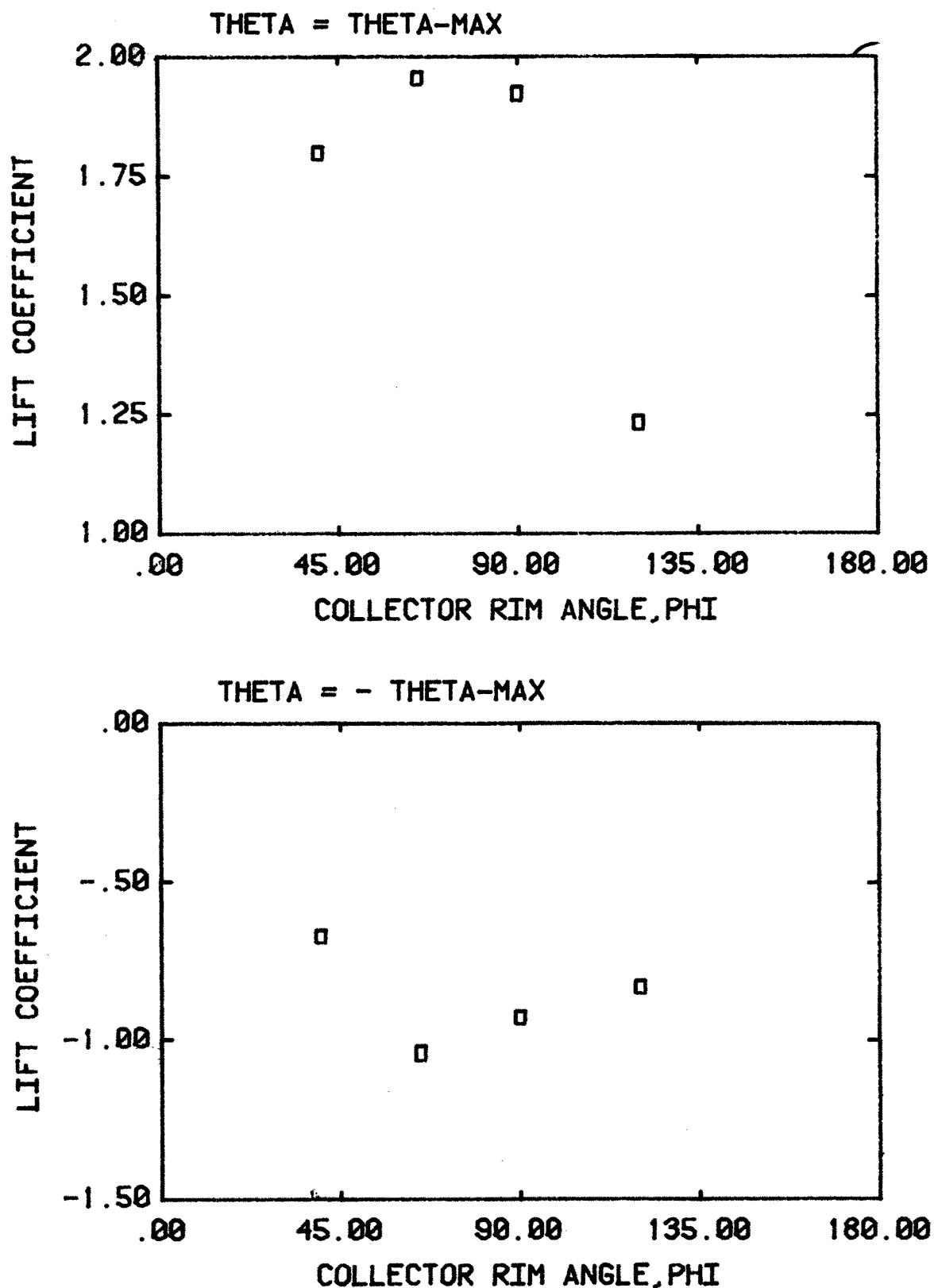
Figure 14b. Effect on the rim angle  $\phi$  on collector loads.
