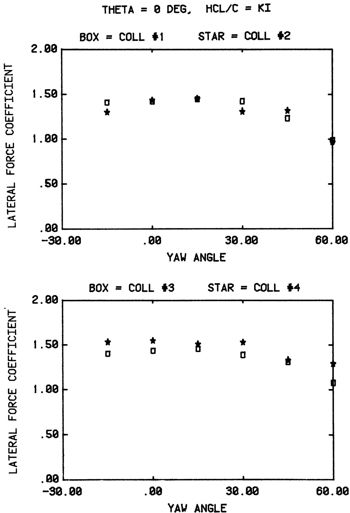
Figure 13a. Variation of single collector loads with yaw angle for  $HCL/C=K_I$ , (configurations 1-4).
