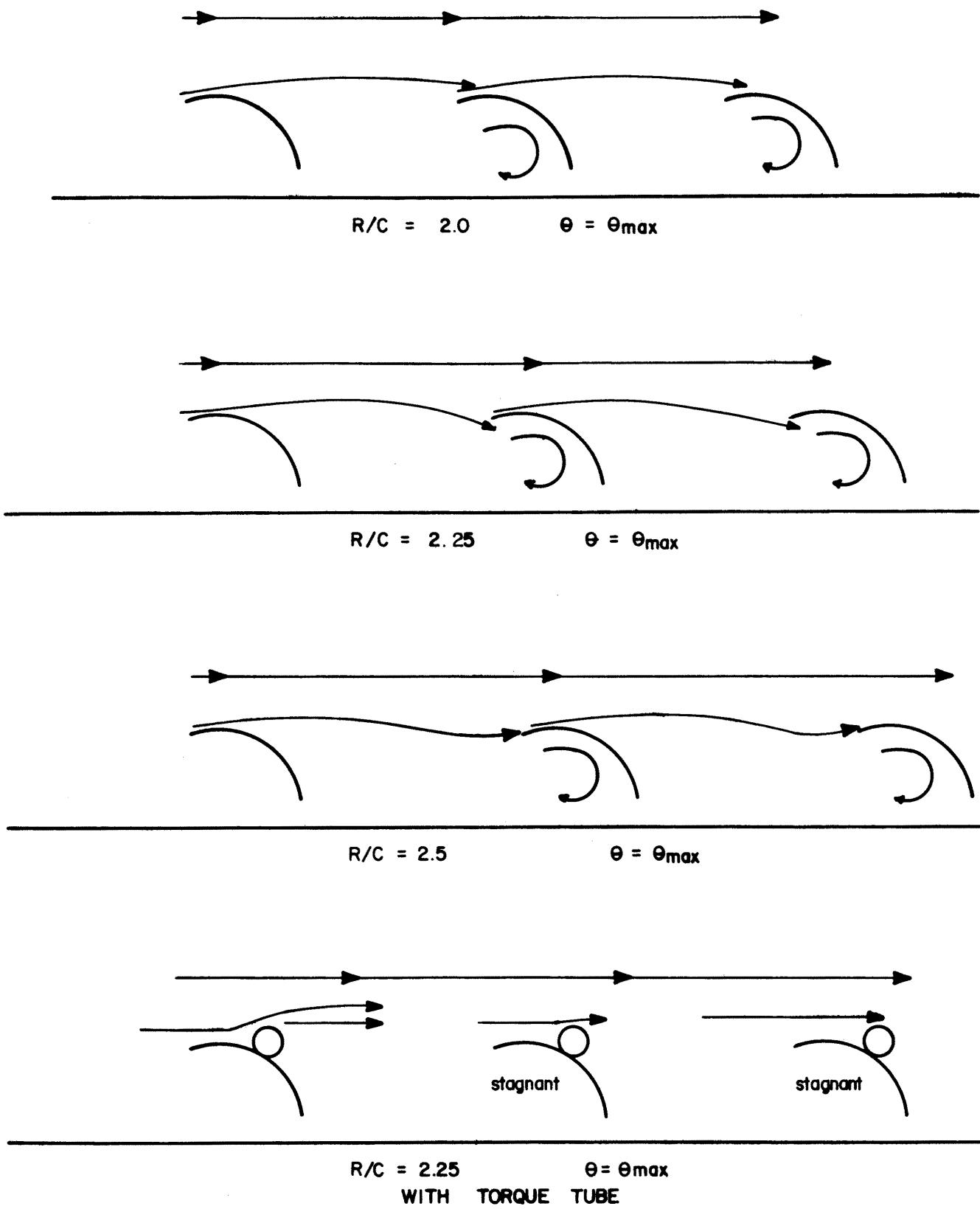
Figure 16c. Effect of the row spacing upon the flow pattern.
