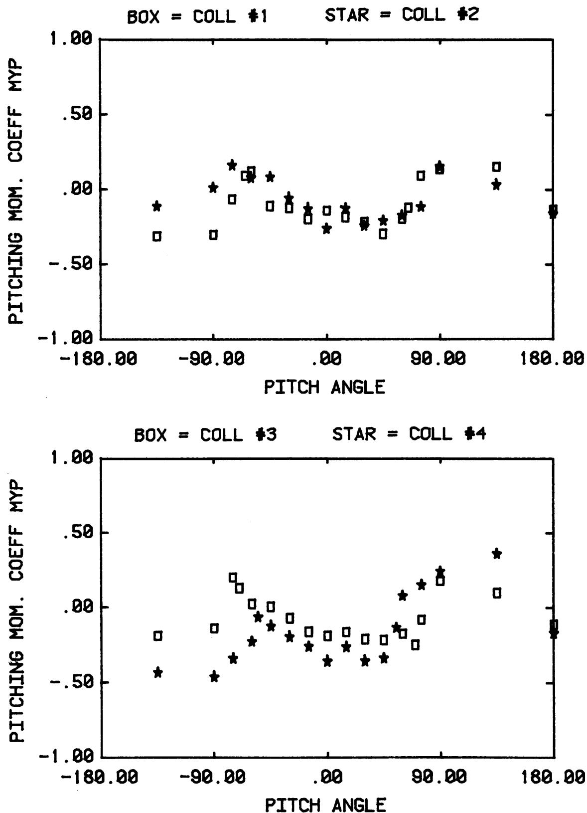
Figure 12c. Variation of single collector loads with pitch angle for HCL/C=K<sub>I</sub>,  $\psi = 0$  (configurations 1-4).
