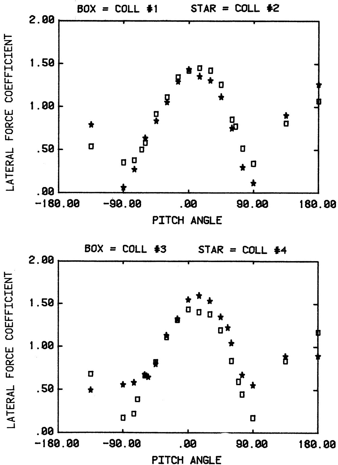
Figure 12a. Variation of single collector loads with pitch angle for  $HCL/C=K_I$ ,  $\psi = 0$  (configurations 1-4).
