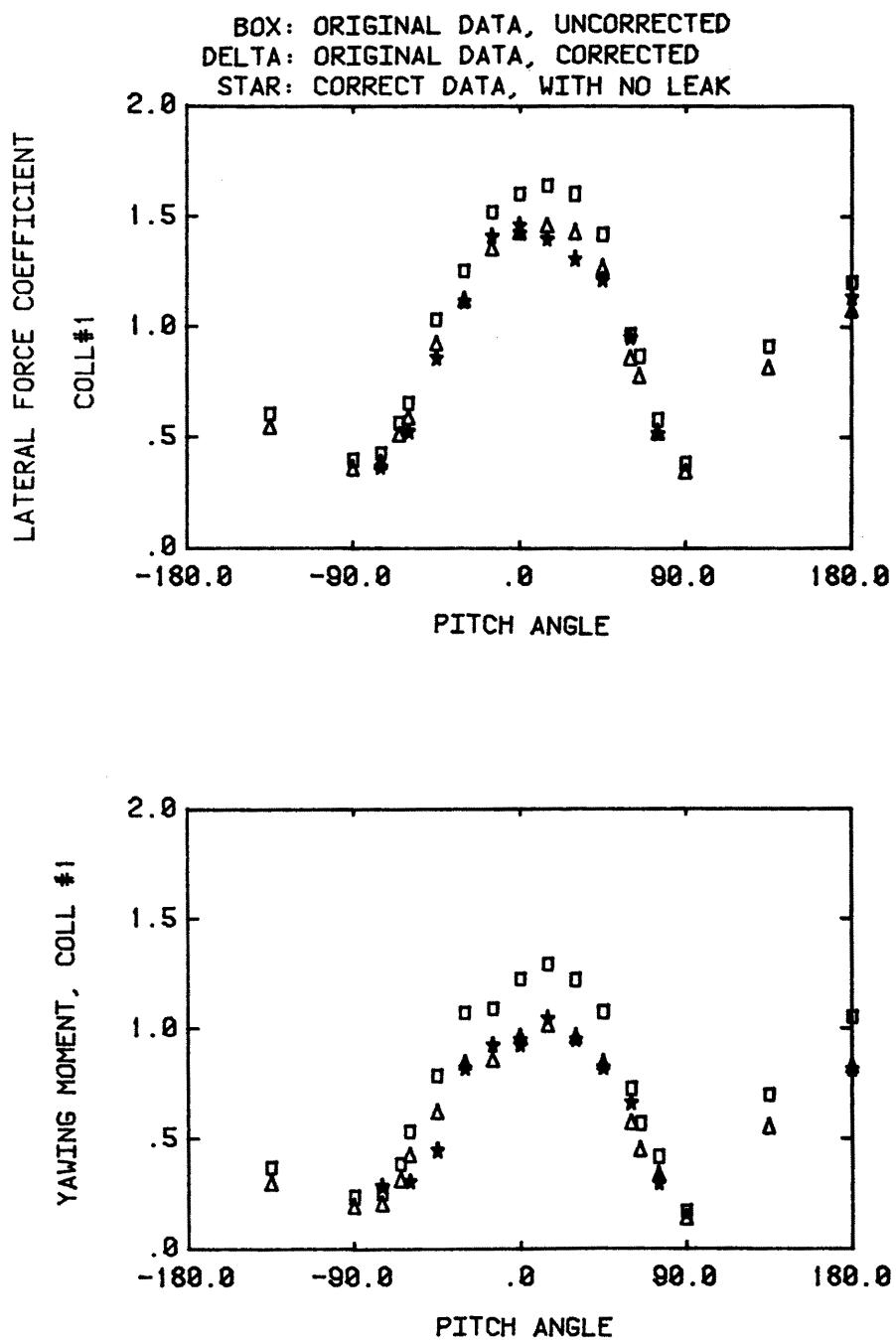
Figure 19. Effect of applying correction to collector 1.
