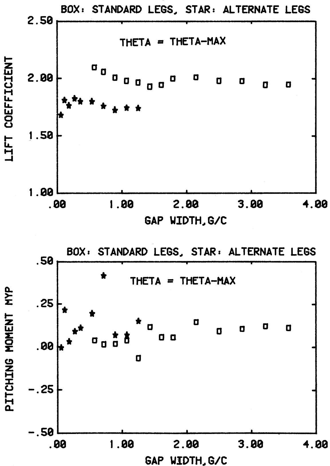
Figure 15b. Effect of gap width on loads for configuration 5.
