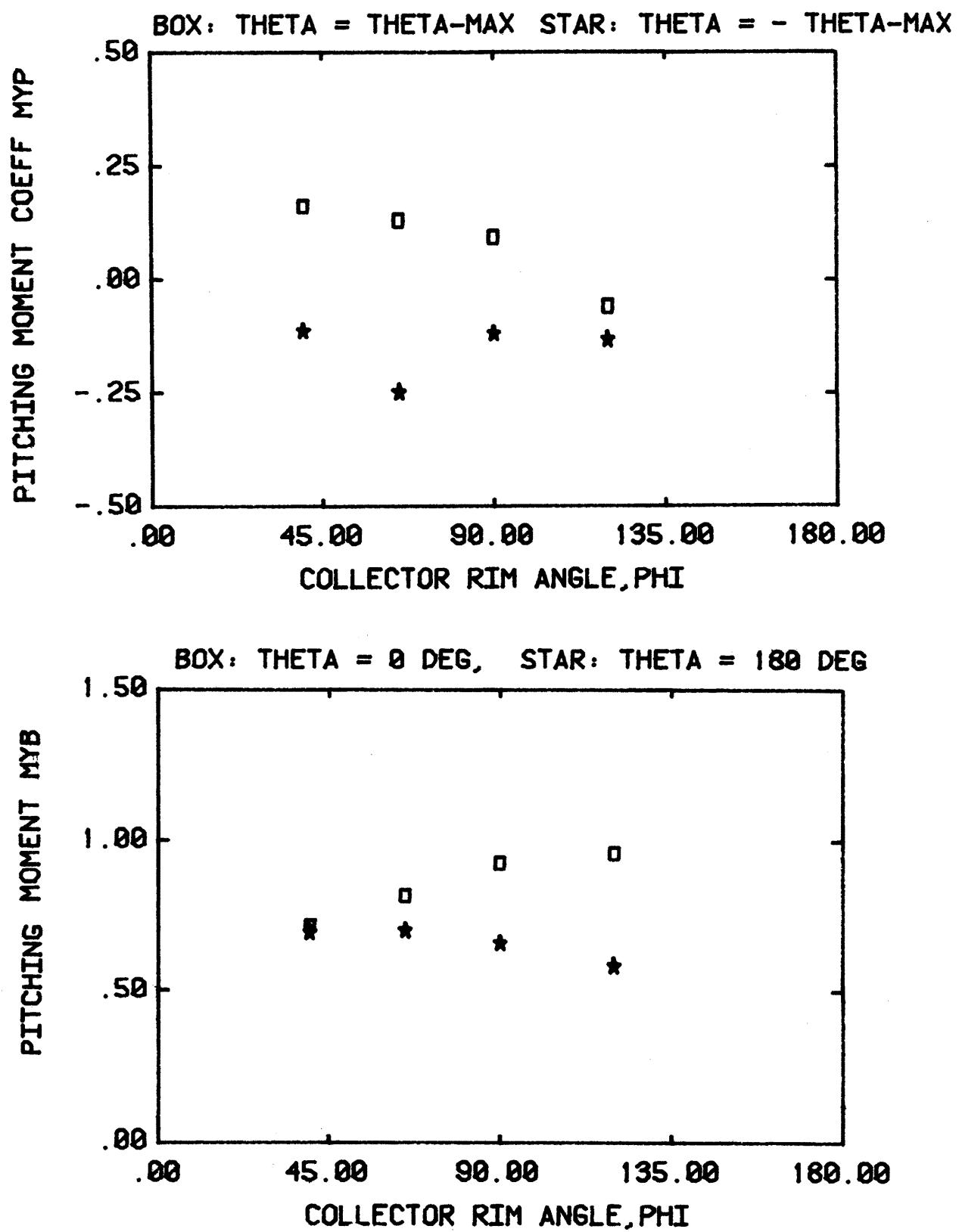
Figure 14c. Effect on the rim angle  $\phi$  on collector loads.
