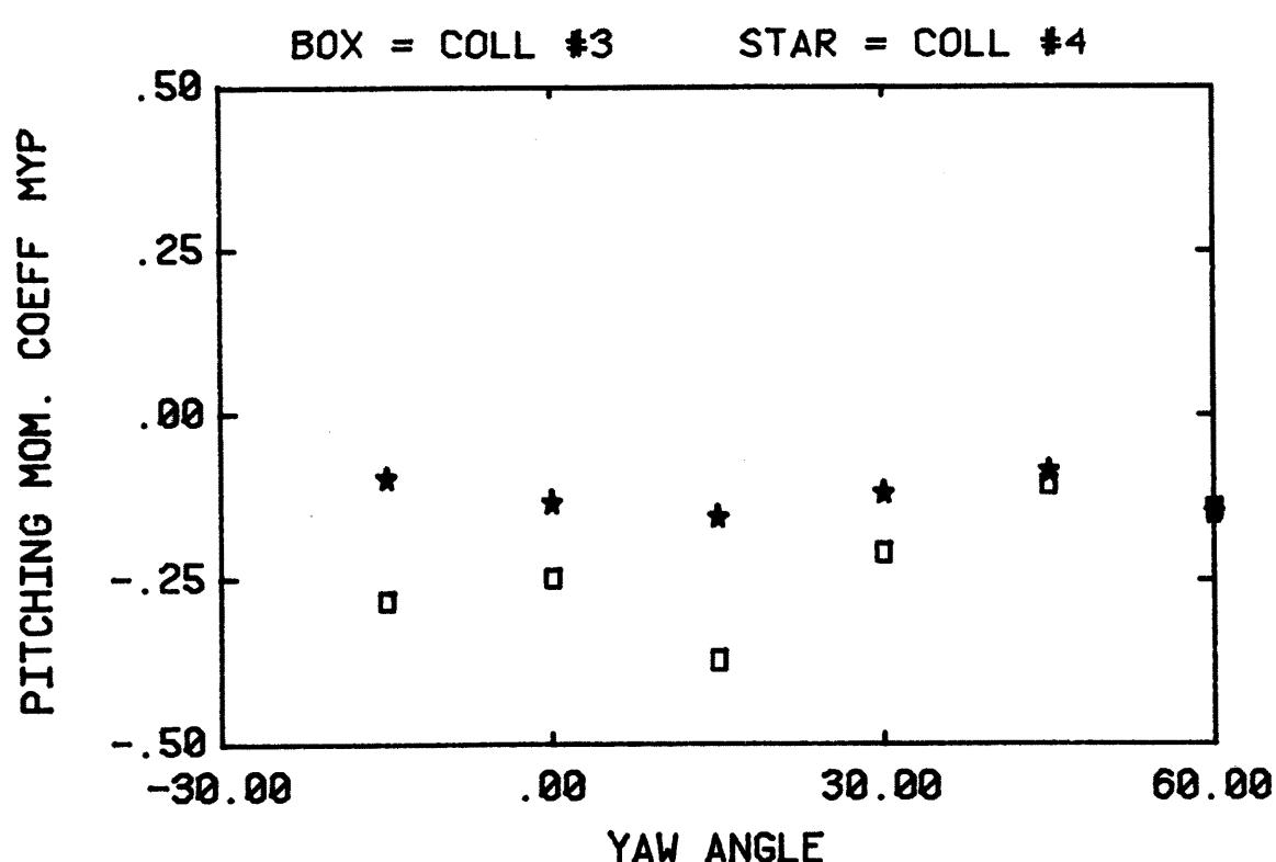
Figure 13h. Variation of single collector loads with yaw angle for HCL/C=K<sub>I</sub>, (configurations 1-4).
