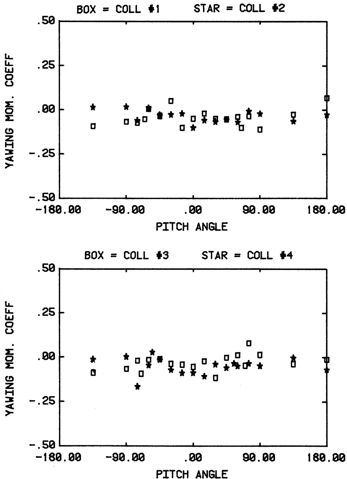
Figure 12e. Variation of single collector loads with pitch angle for HCL/C=K<sub>I</sub>,  $\psi = 0$  (configurations 1-4).
