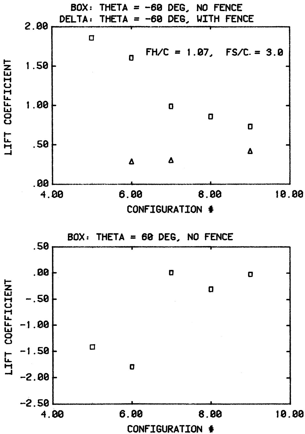
Figure 17b. Influence of array field configuration and fences on collector loads.
