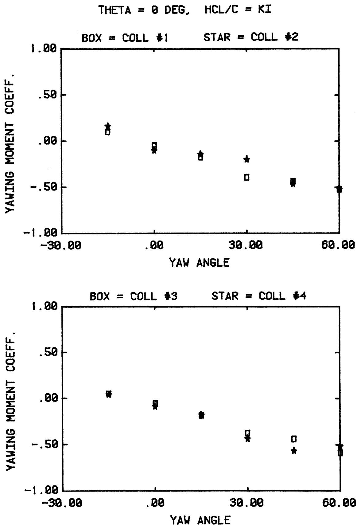
Figure 13c. Variation of single collector loads with yaw angle for HCL/C=K<sub>I</sub>, (configurations 1-4).
