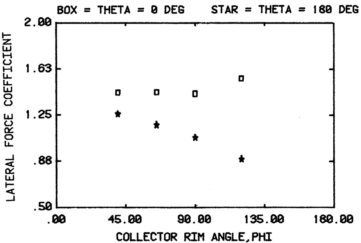
Figure 14a. Effect on the rim angle  $\phi$  on collector loads.
