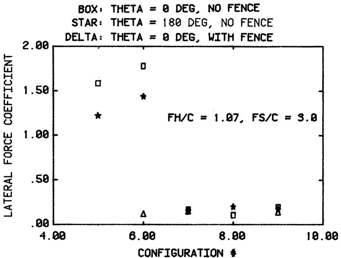
Figure 17a. Influence of array field configuration and fences on collector loads.
