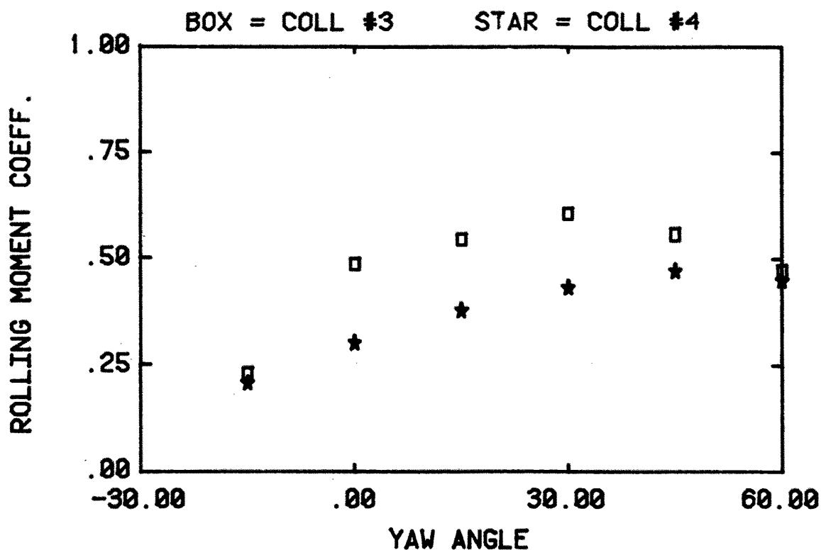
Figure 13i. Variation of single collector loads with yaw angle for HCL/C=K<sub>I</sub>, (configurations 1-4).
