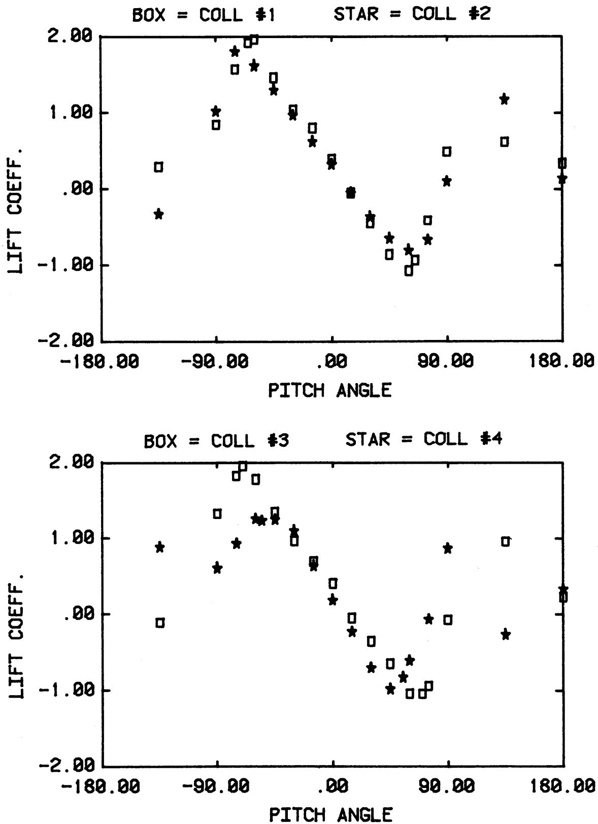
Figure 12b. Variation of single collector loads with pitch angle for  $HCL/C=K_I$ ,  $\psi = 0$  (configurations 1-4).
