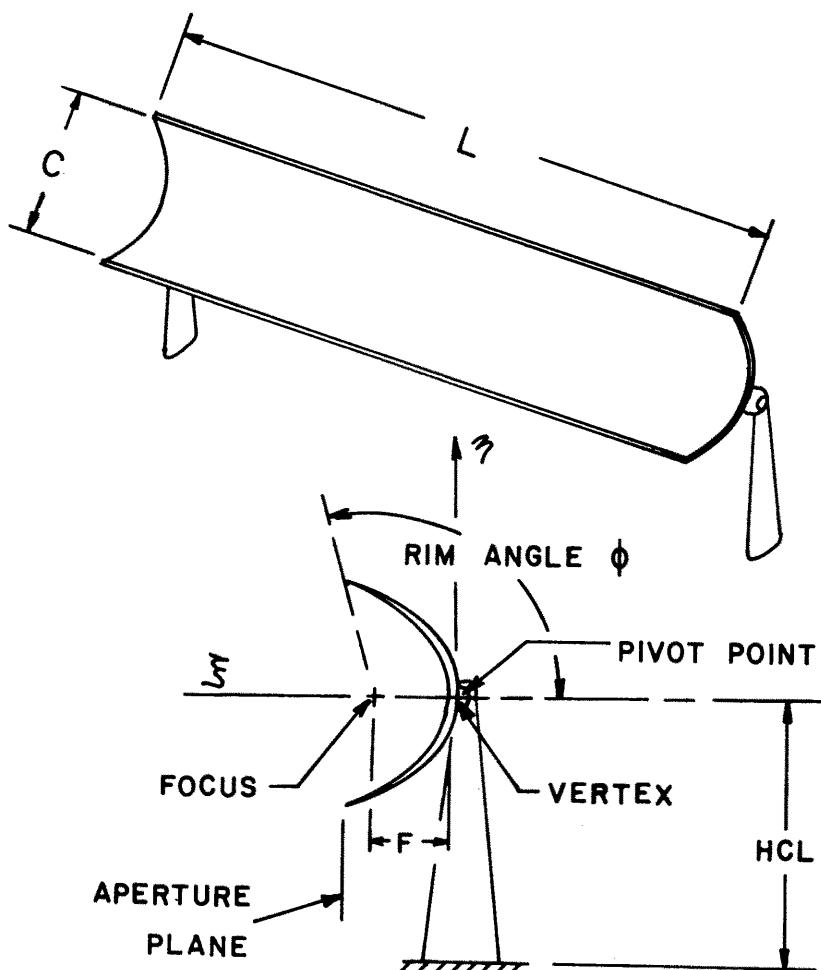
Figure 2a. Collector shapes for configurations 1-4.
