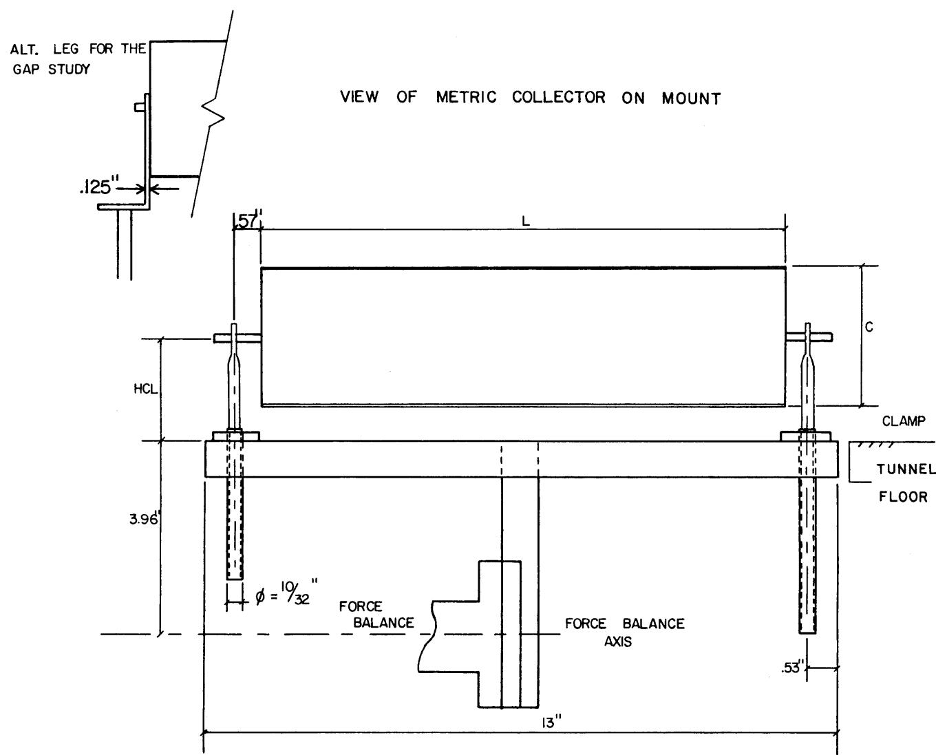
Figure 4. Collector and force balance mount.
