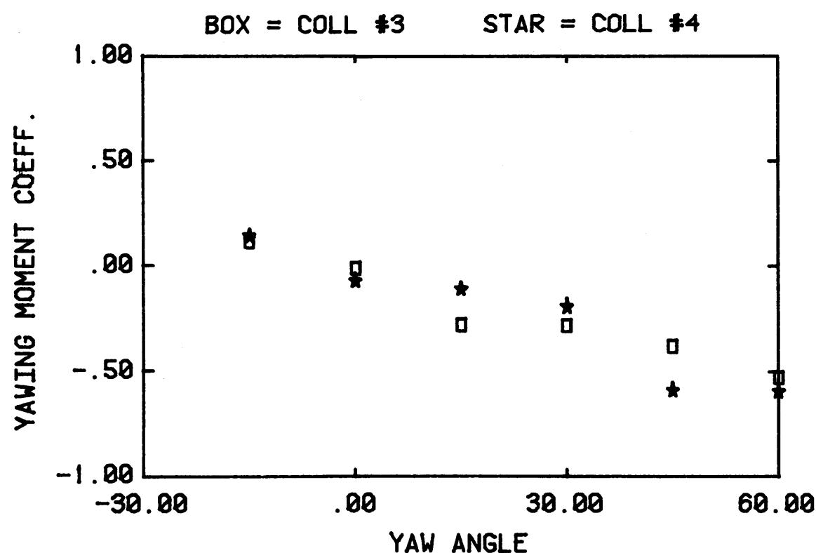
Figure 13d. Variation of single collector loads with yaw angle for HCL/C=K<sub>I</sub>, (configurations 1-4).
