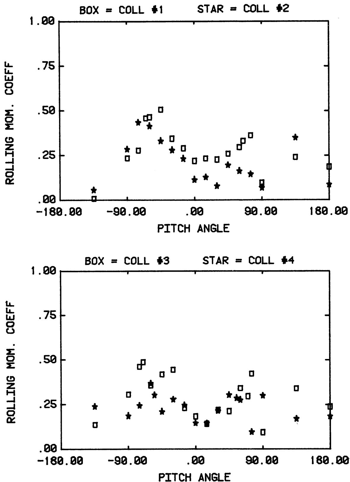
Figure 12f. Variation of single collector loads with pitch angle for  $HCL/C=K_I$ ,  $\psi = 0$  (configurations 1-4).
