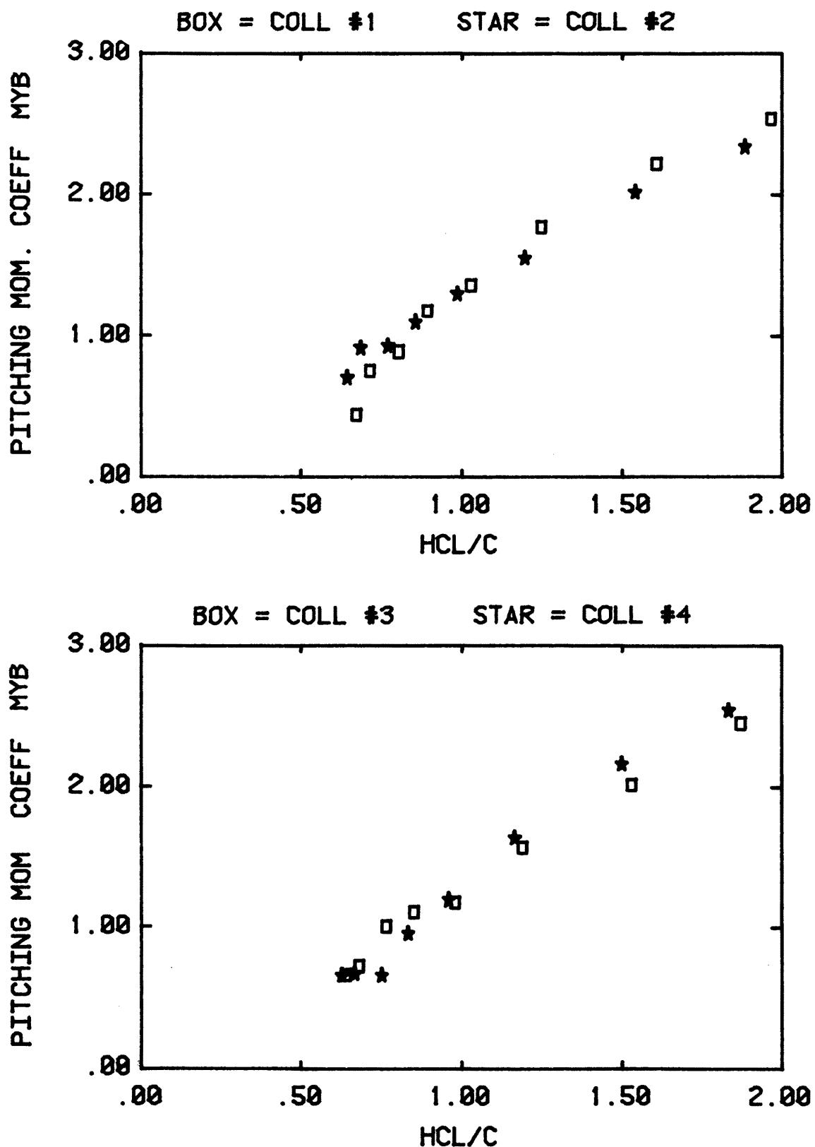
Figure 10c. Effect of height on coefficients at  $\theta = 0$ ,  $\psi = 0$  (configurations 1-4).
