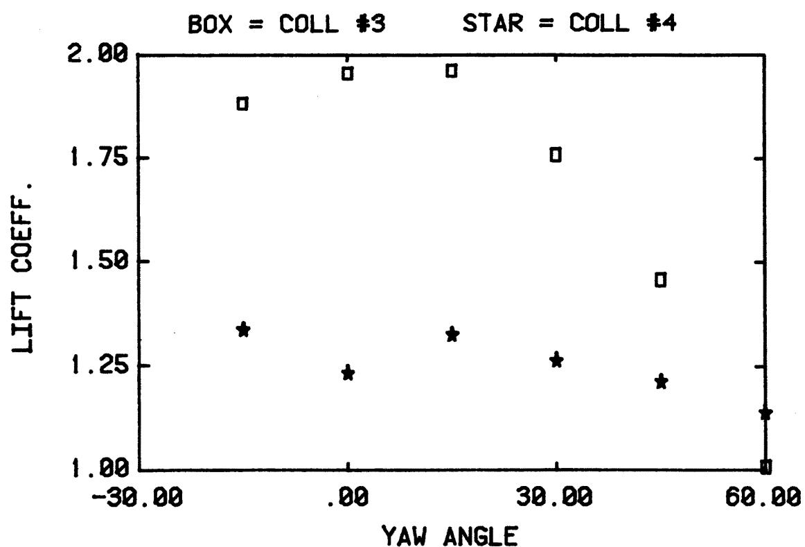
Figure 13e. Variation of single collector loads with yaw angle for HCL/C=K<sub>I</sub>, (configurations 1-4).
