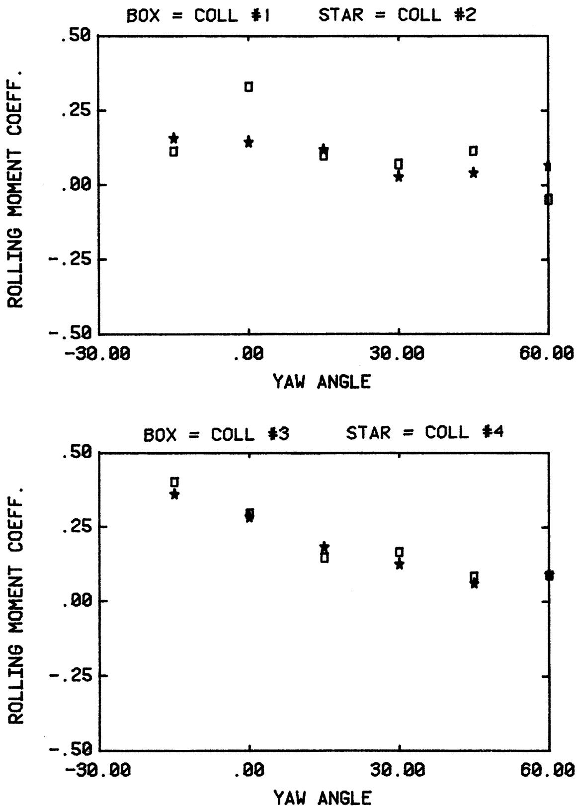
Figure 13j. Variation of single collector loads with yaw angle for HCL/C=K<sub>I</sub>, (configurations 1-4).
