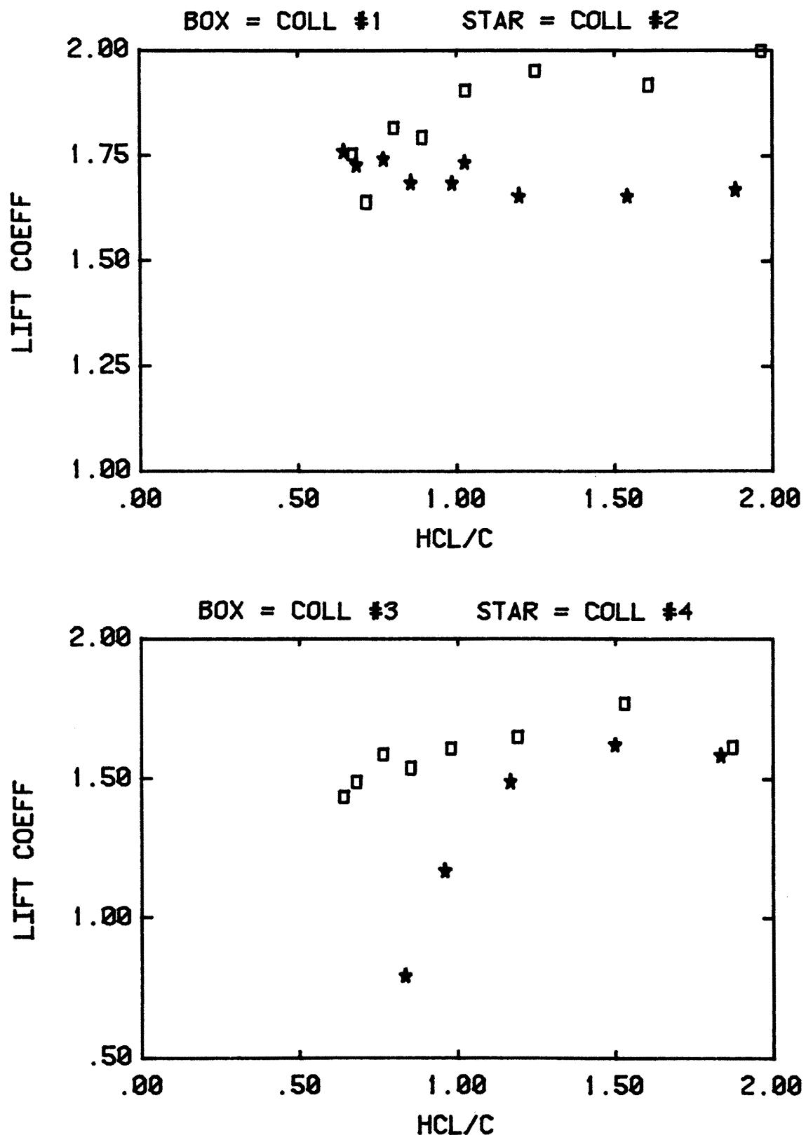
Figure 11. Effect of height on lift at  $\theta_{\max}$ ,  $\psi = 0$  (configurations 1-4).
