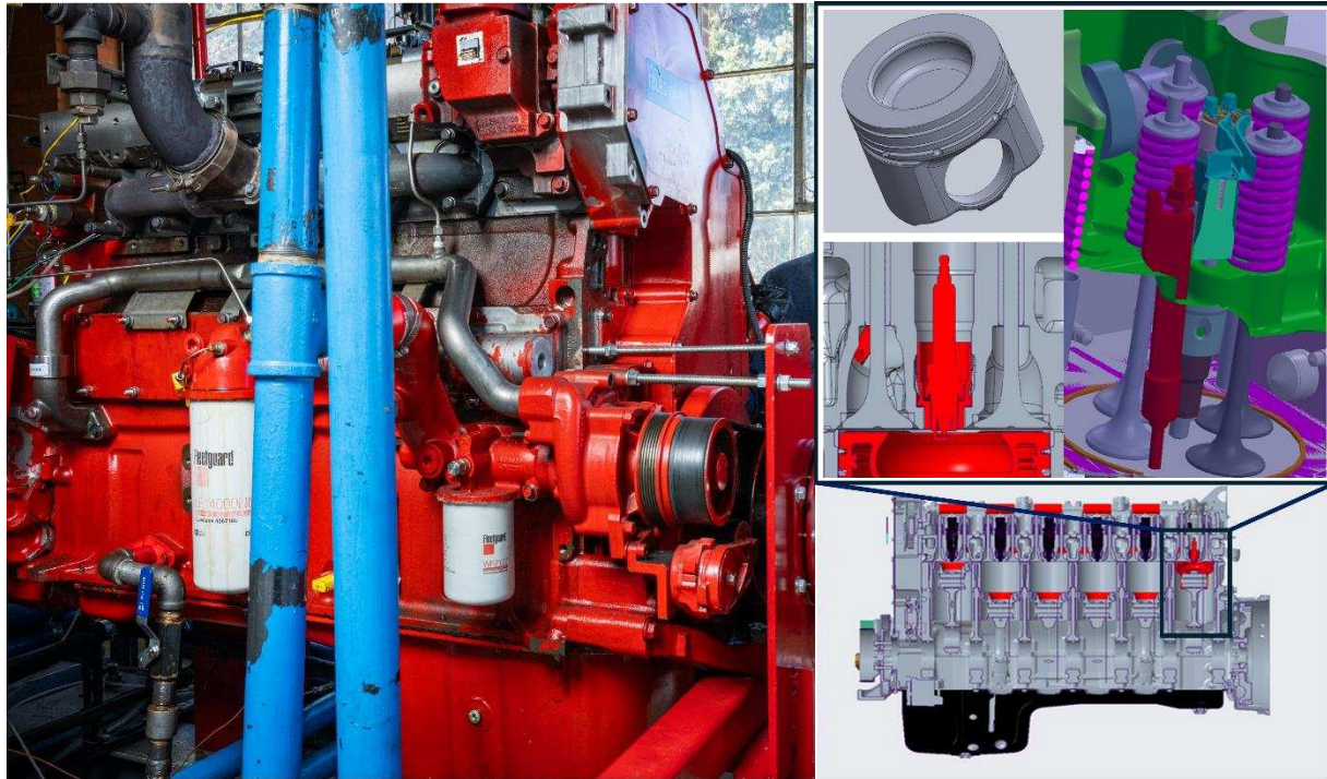
Figure 2.8. Left - X15 SCE; Top Right – Cut-out of key sections of the cylinder head showing the valves and the centrally located spark plug, off-center installed direct injector and baseline 9.3:1 piston; Bottom Right – CAD of the six-cylinder engine showing the active single cylinder, cylinder 6
