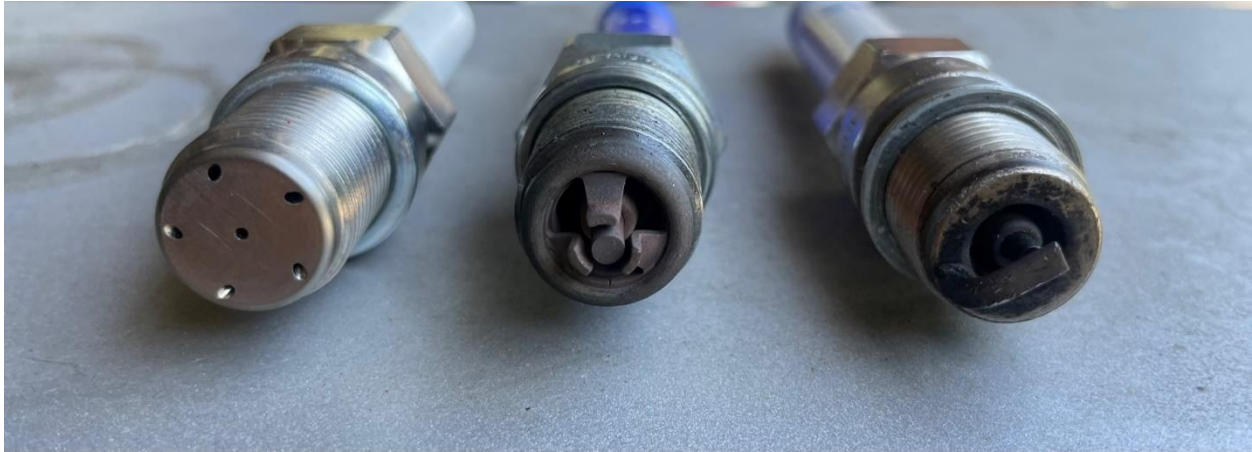
Figure 2.5. Spark plug options for the heavy-duty LPG engine operation Left: The Woodward Fast Turbulent Igniter (FTI) Pre-chamber sparkplug, Middle: The Altronic L1863B 3-prong massive nickel sparkplug, Right: The regular J-Gap sparkplug.
