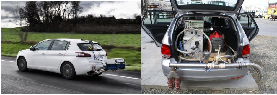
Figure 2.2: Examples of on-road sampling from light-duty vehicles with the PEMS placed in the trunk (left) and on a skid above the tailpipe (right). Courtesy: (Portable Emissions Measurement System)
