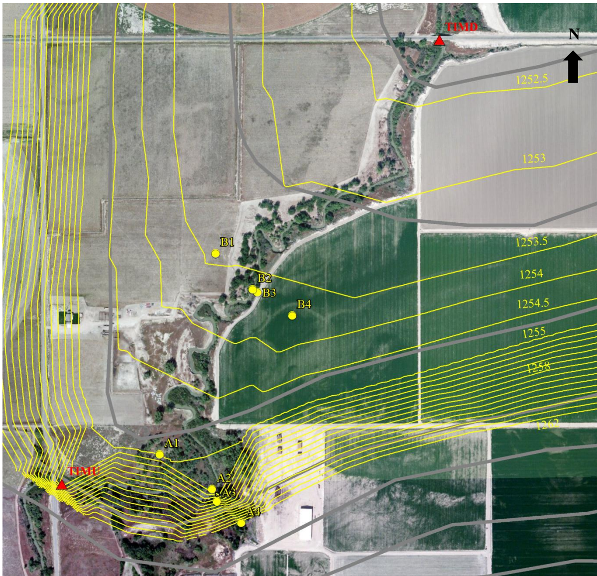
Figure 55. Water table contour plot from model results (grey lines) and Timpas Creek averaged field measurements in October (yellow lines).
