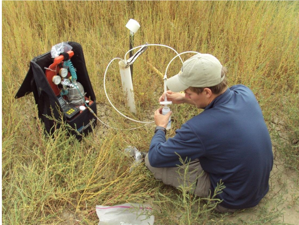
Figure 30. A researcher collects samples from a well. Pump tubing and CO 2 power pack are shown.
