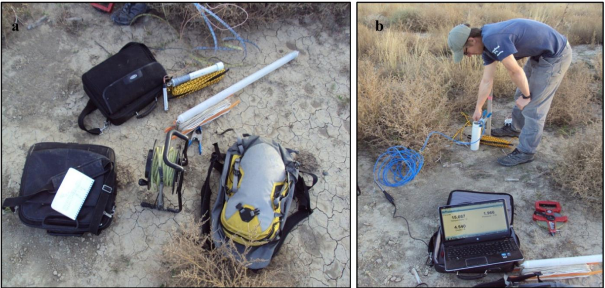
Figure B- 1. a) Materials required for slug testing procedure and b) a slug test in action.
