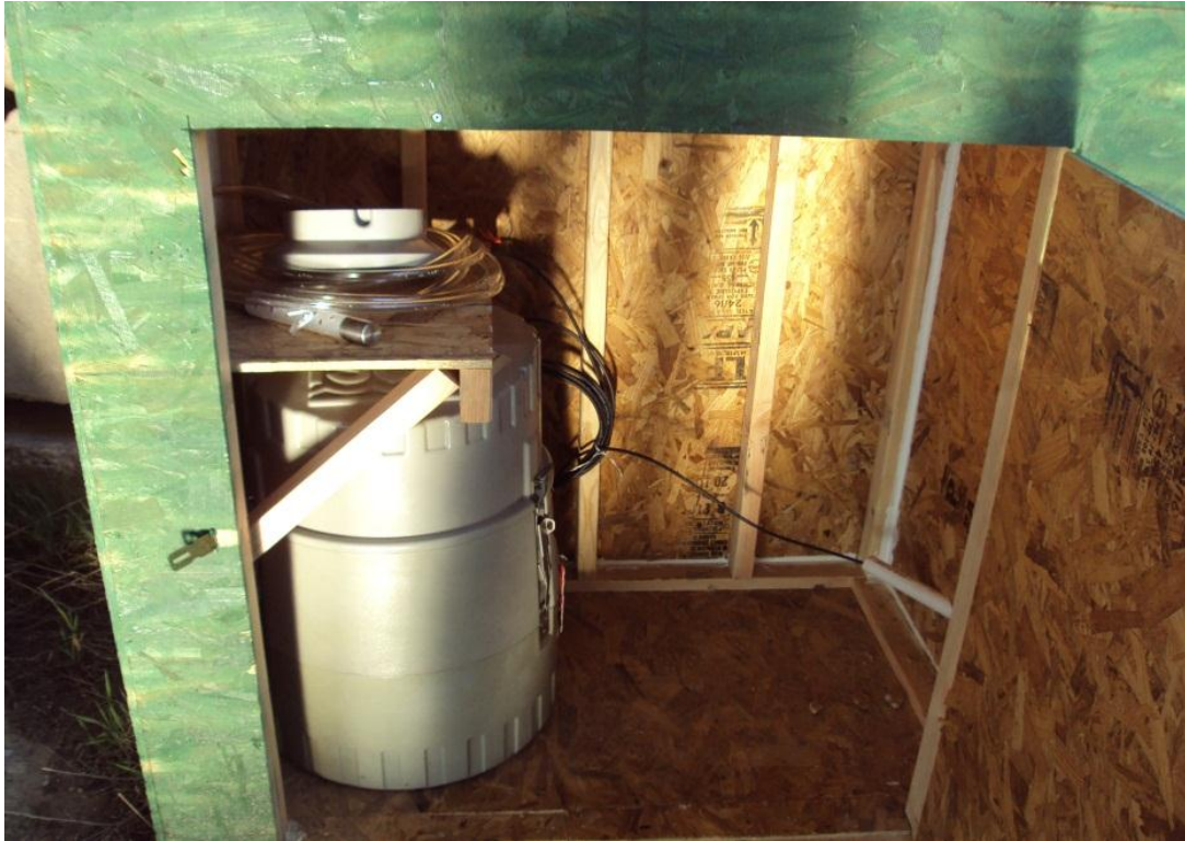
Figure 31. Shelter and auto-sampler setup at ARKU.
