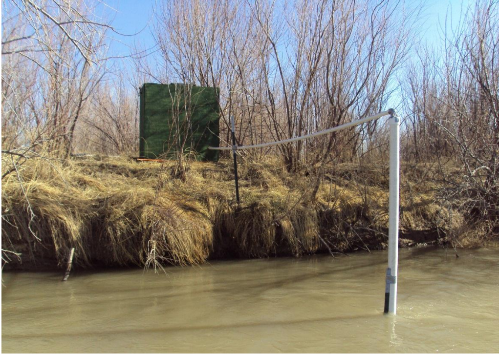
Figure 5. Aqua Troll housed in PVC pipe at ARKD monitoring station.
