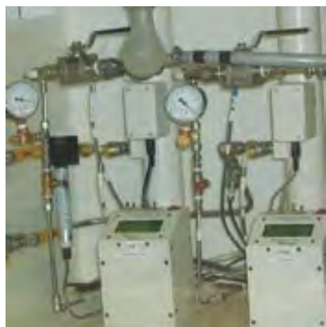
Figure 3, illustration of the specially configured Nephelometer for hygroscopicity measurements
