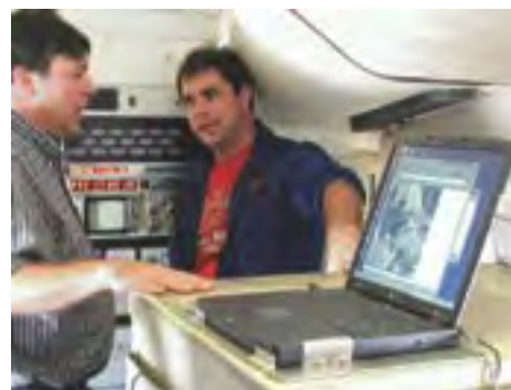
Figure 2, a laptop displaying the 42 kb water vapor JPEG image that was downloaded during a WP-3 flight into Tropical Storm Hanna on September 13, 2002. It took approximately 2 minutes to download the image. Also shown is Mike Black of HRD and Sean McMillan, a member of the Aircraft Operations Center NOAA-43 flight crew.
