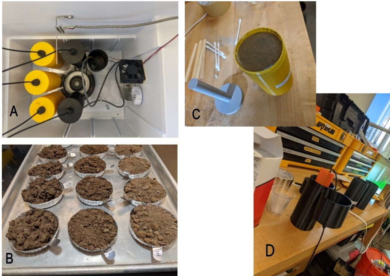
Figure 5. Four pictures demonstrate a run with: (A) five soil samples inside the custom temperature control chamber, (B) tins with three distinct soil water contents ready for the oven after a calibration run, (C) a 3D printed sensor container with a saturated sample alongside a packing tool, (D) and a sensor inserted with the container top-cap removed to see inside.
