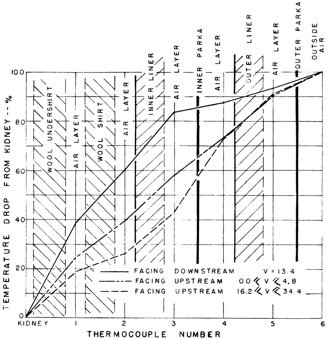
Fig. 7 Temperature drops through uniform.
