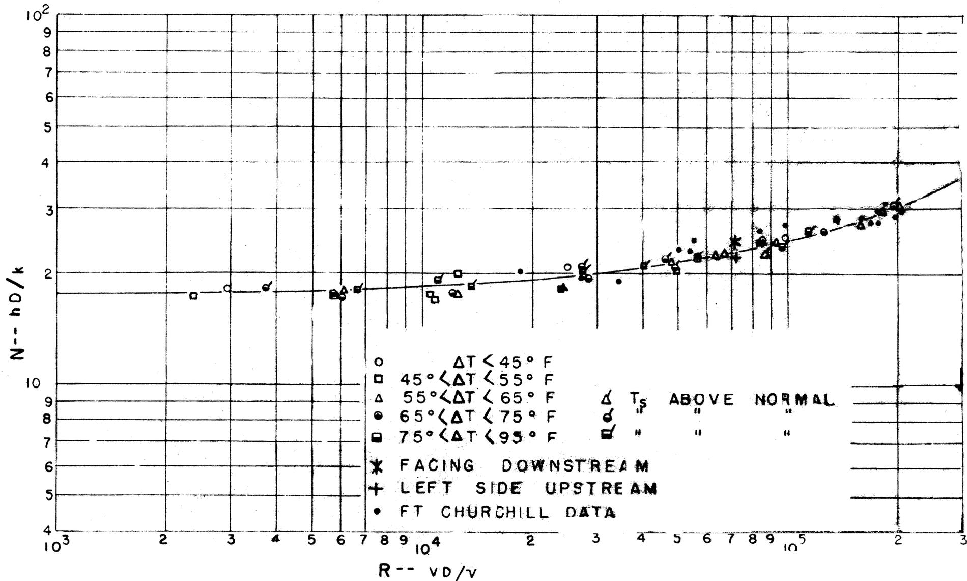
Fig. 5 Nusselts number as a function of Reynolds number for wind chill from a Copper Man in Ex-50 Arctic uniform.
