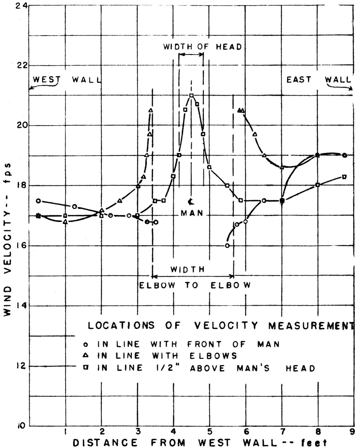
Fig. 2 Typical velocity distribution across section including the Copper Man.
