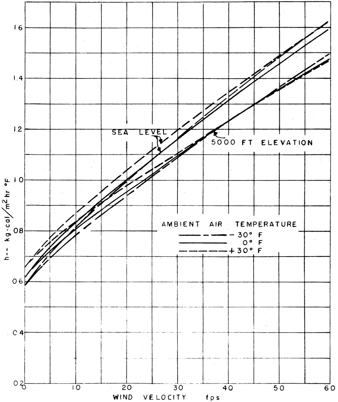
Fig. 8 Effects of ambient air temperature and elevation above sea level upon wind chill.
