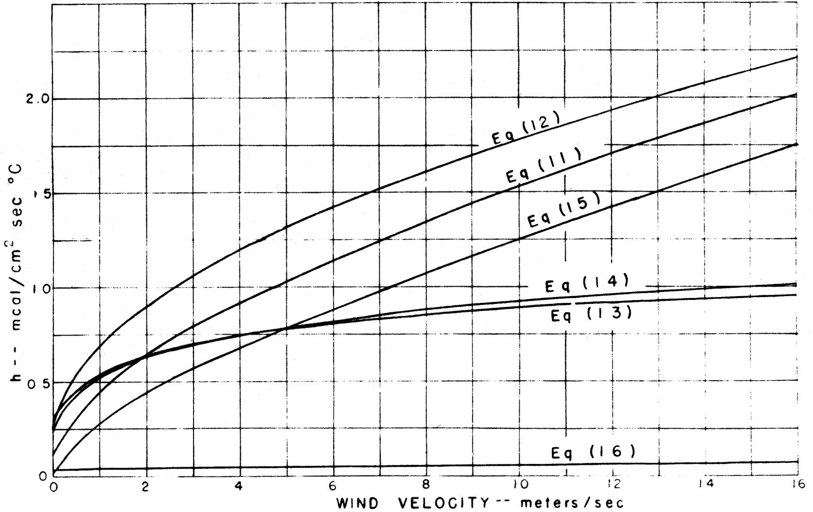
Fig. 9 Comparison of various wind chill formulae.
