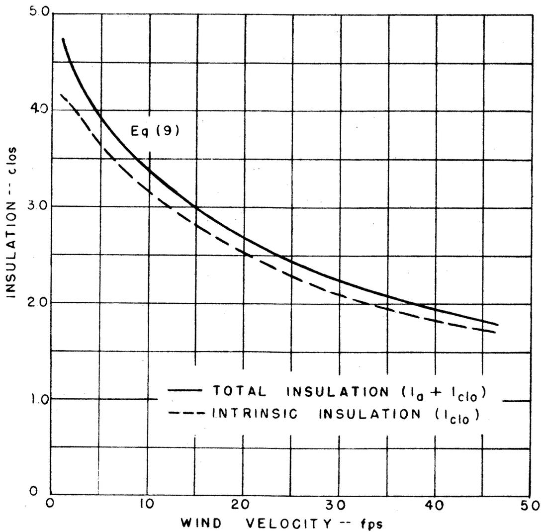
Fig. 6 Insulation values for the Ex-50 Arctic uniform.
