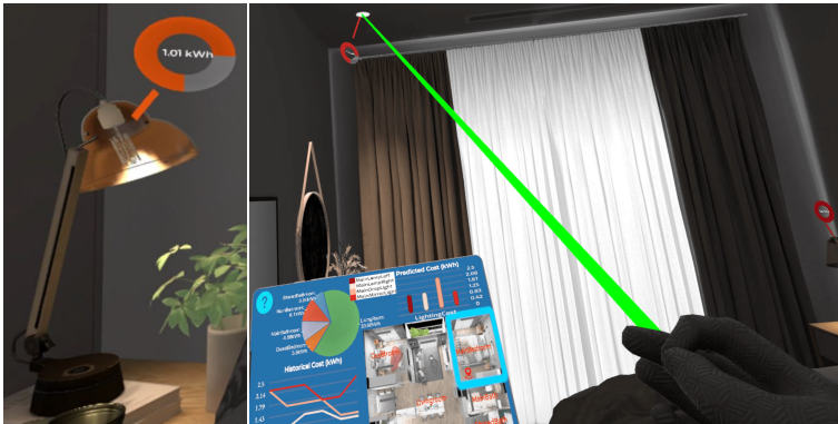
Fig. 3. Left: An example of an embedded visualization (referred to as EmbVis) that is attached to a bedside lamp. Right: The user points at a light with their right controller and presses the trigger to adjust the brightness level at incremental stages.
