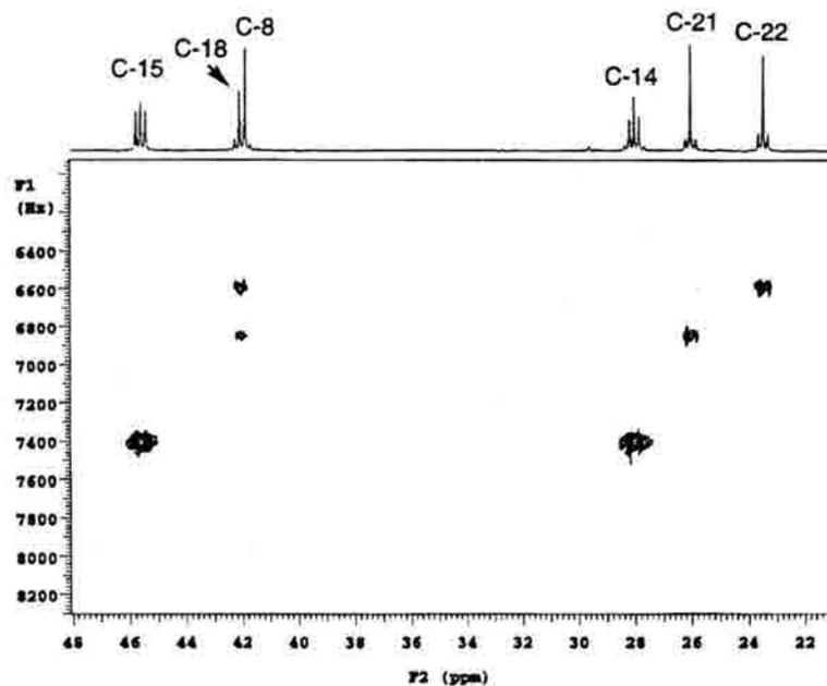
Figure 5. Portion of the INADEQUATE spectrum of austamide (21) derived from a  $^{13}\text{C}_2$ -acetate feeding experiment exhibiting the coupling between the geminal methyl groups and C-18. The corresponding portion of the  $^{13}\text{C}$ -spectrum is shown at the top.
