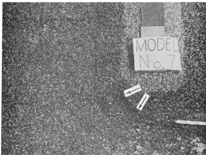
Fig. 33 - Photograph of the abutment after draining the flume
