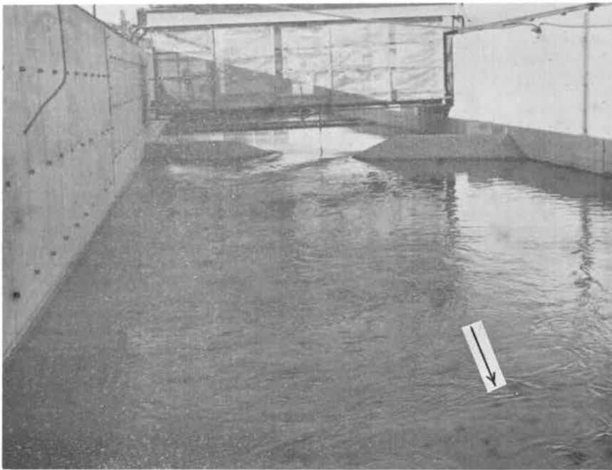
Fig. 22 - Photograph of the water surface characteristics for a skewed model at Q = 11.1 cfs
