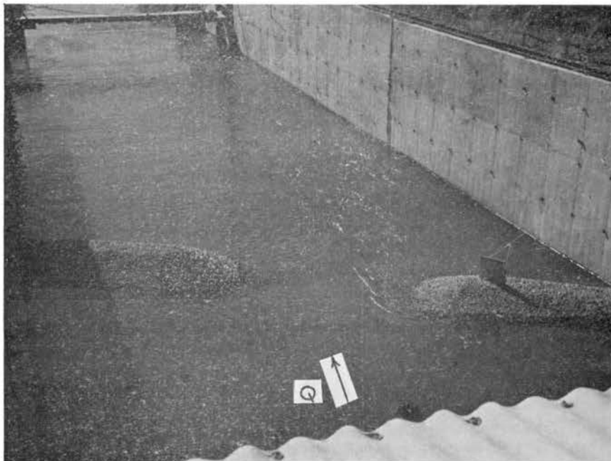
Fig. 26 - Photograph of the protected nose of the downstream embankment and the jet properties at Q = 13.9 cfs
