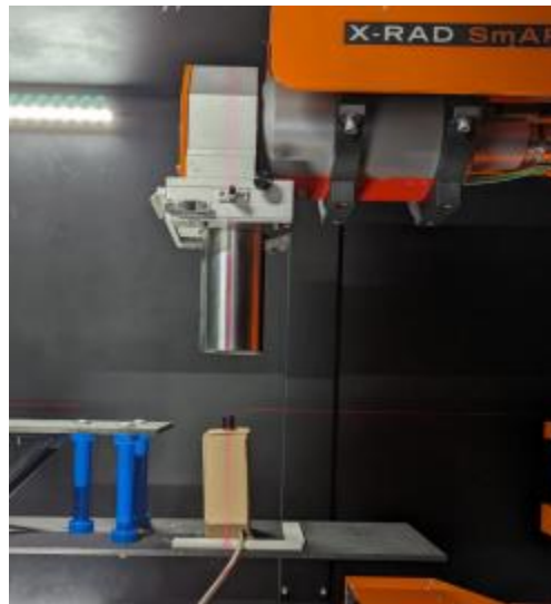
Figure 30: Low energy ion chamber placed at isocenter of the Small Animal Irradiator.
