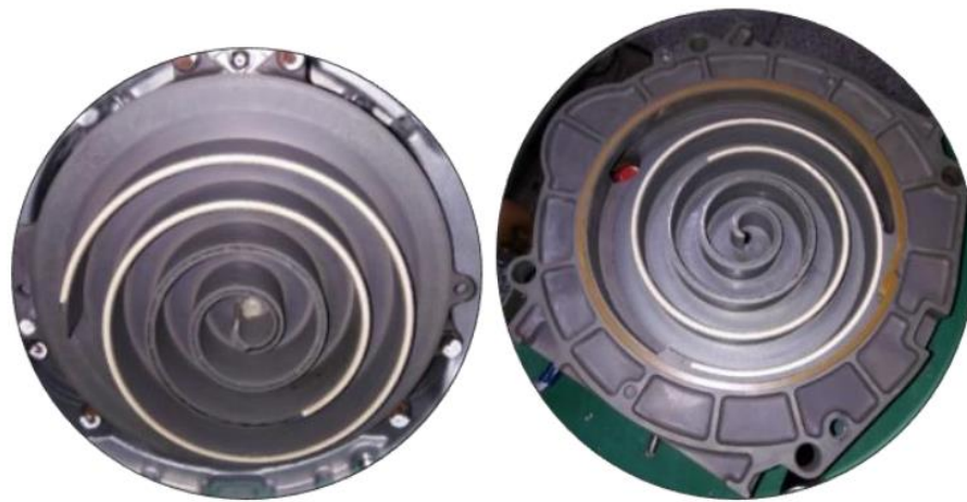
Figure 2-5. Picture of what the scrolls within a scroll compressor with the orbiting scroll on the left and stationary scroll on the right [74].
