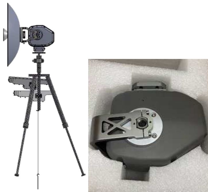
Figure 4.2. Geometry of the QPRA (Left) and Gimbal Mechanism (Right)
