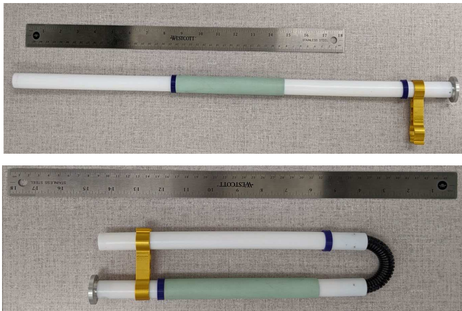
Figure 3.13. RMA Prototype showing Deployed (Top) and Stowed (Bottom) Configuration
