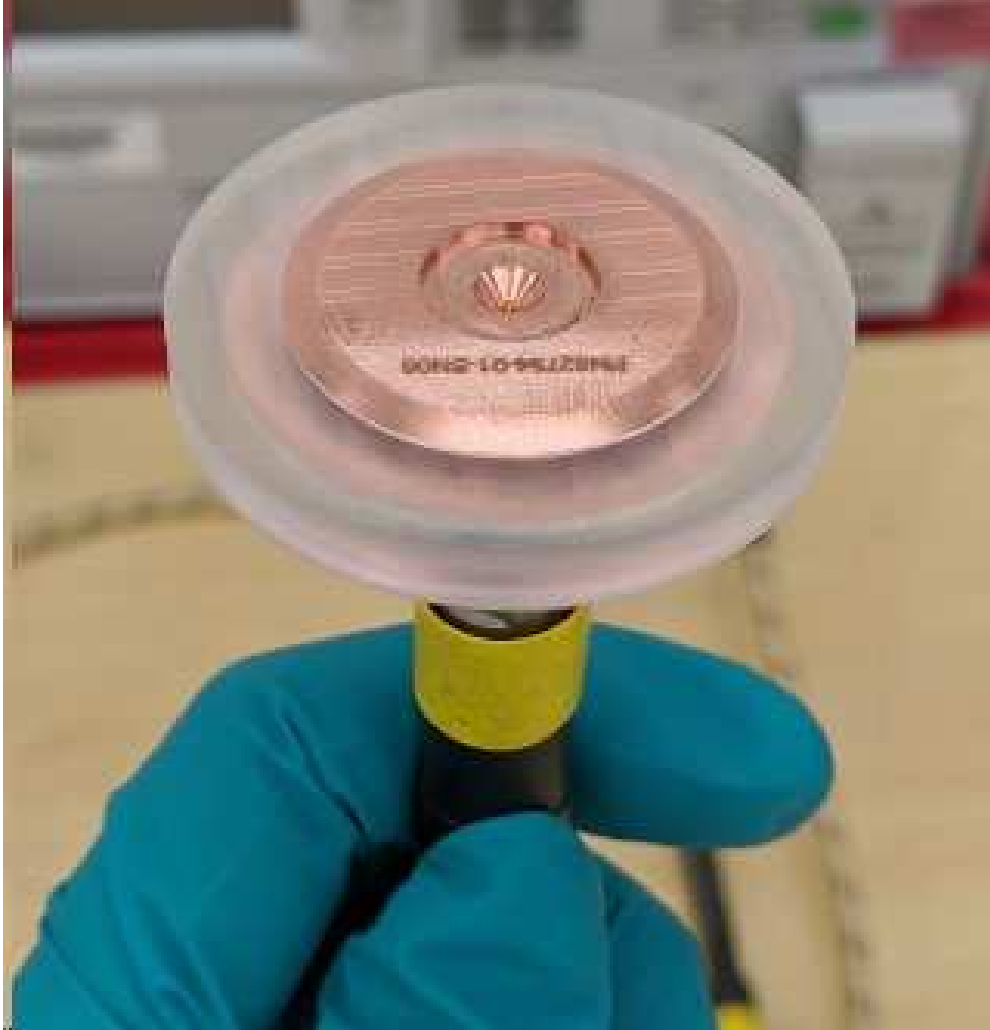
Figure 3.19. Prototype Unit of the BCA with a Protective Radome and the RMA
