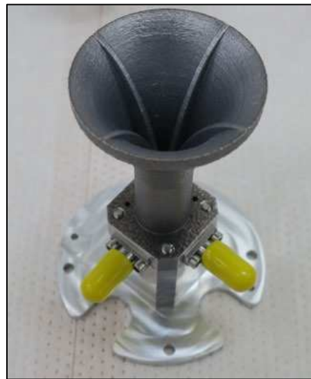
Figure 4.4. Quad-Ridge Horn Assembly with Transitions showing Orthogonal Ports
