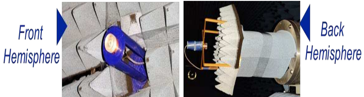
Figure 3.7. Pen-Cap Air Antenna in Anechoic Chamber Setup
