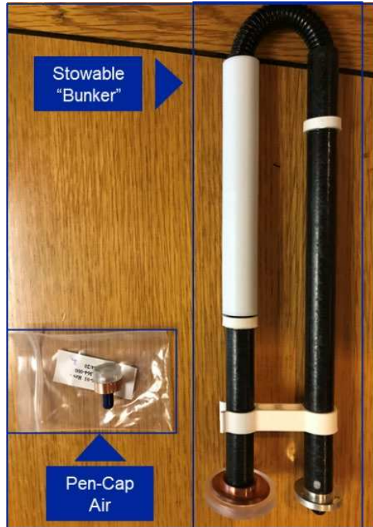
Figure 3.28. Pen-Cap Air & Bunker Antenna Prototypes
