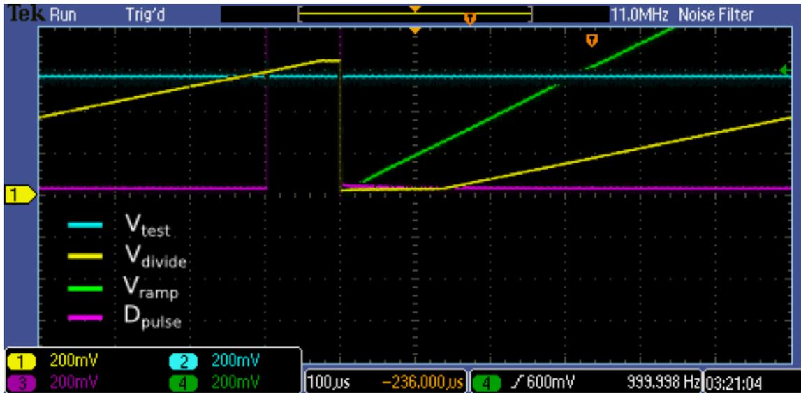
FIGURE 7.1. Negative Output in Silicon Capacitive Sensor
