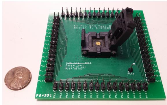
(B) Socket installed on breakout board
