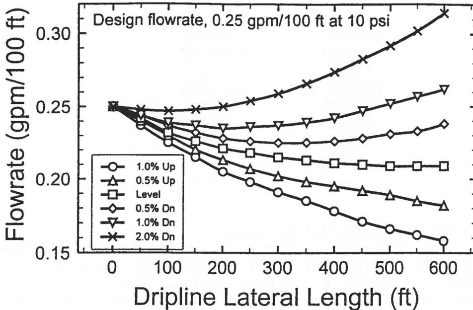
Figure 3. Calculated dripline flowrates as affected by slope.
